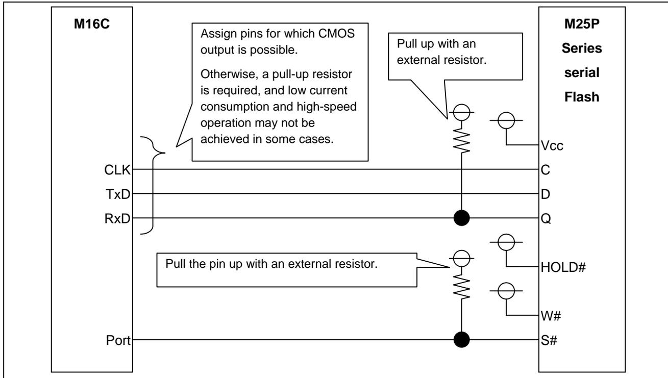
**Figure 1.1 Serial Flash Connection Example**
