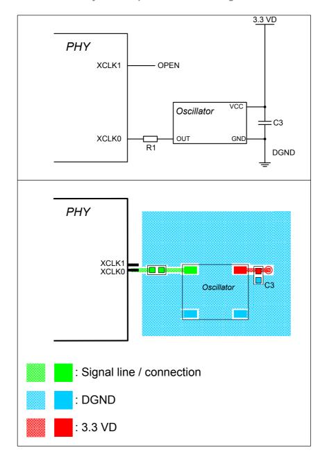
Figure 7-2 Schematic and layout example for oscillator usage
