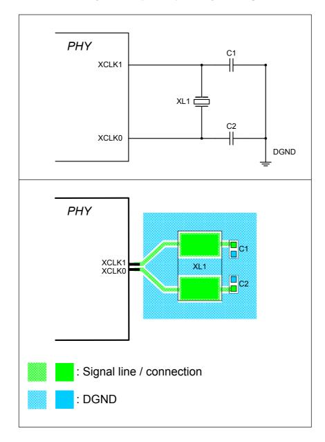
Figure 7-1 Schematic and layout example for quartz crystal usage
