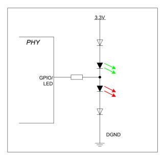
Figure 8-2 Circuit for LED-MUX operation
