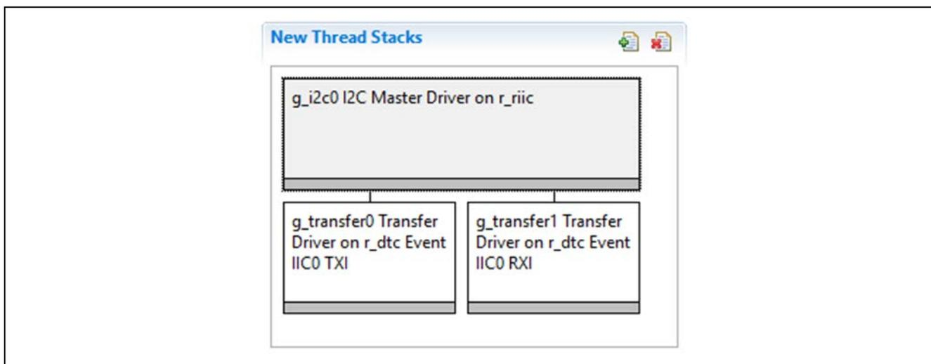
**Figure 2 I<sup>2</sup>C Master HAL Module Stack**
