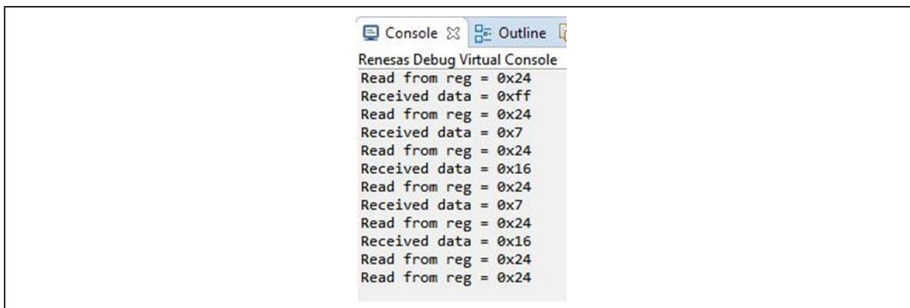
Figure 5 Example Output from I<sup>2</sup>C Master HAL Module Application Project
