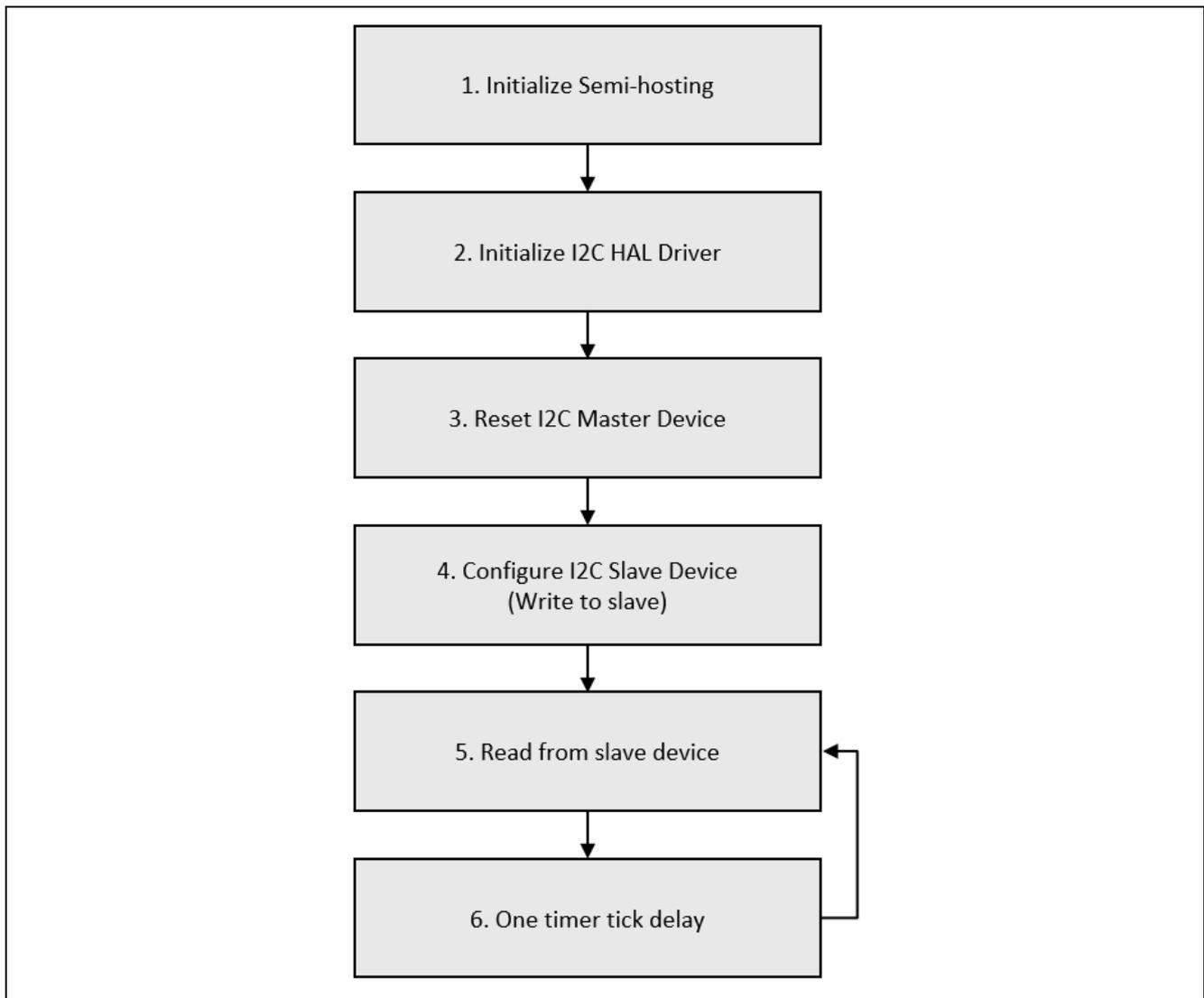
**Figure 4 Detailed flow chart of I<sup>2</sup>C Master HAL Module Application Project**
