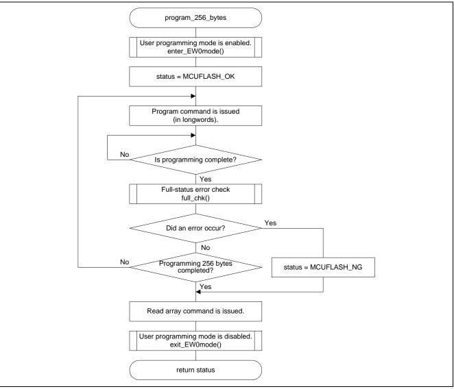
Figure 12 Flowchart (program\_256\_bytes)
