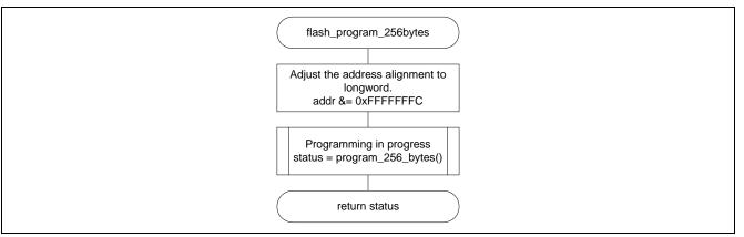
Figure 8 Flowchart (flash\_program\_256bytes)
