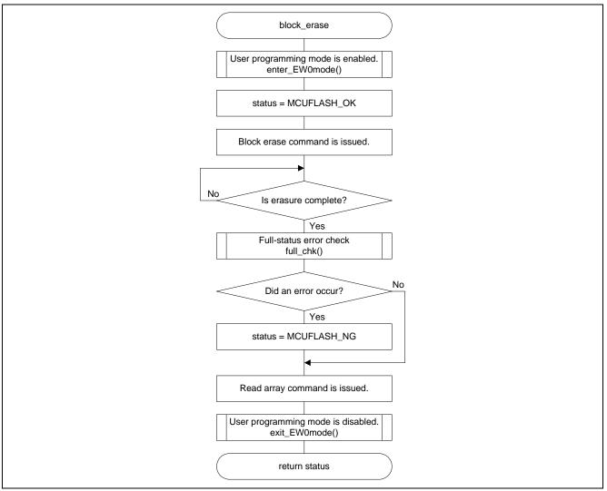
Figure 11 Flowchart (block\_erase)
