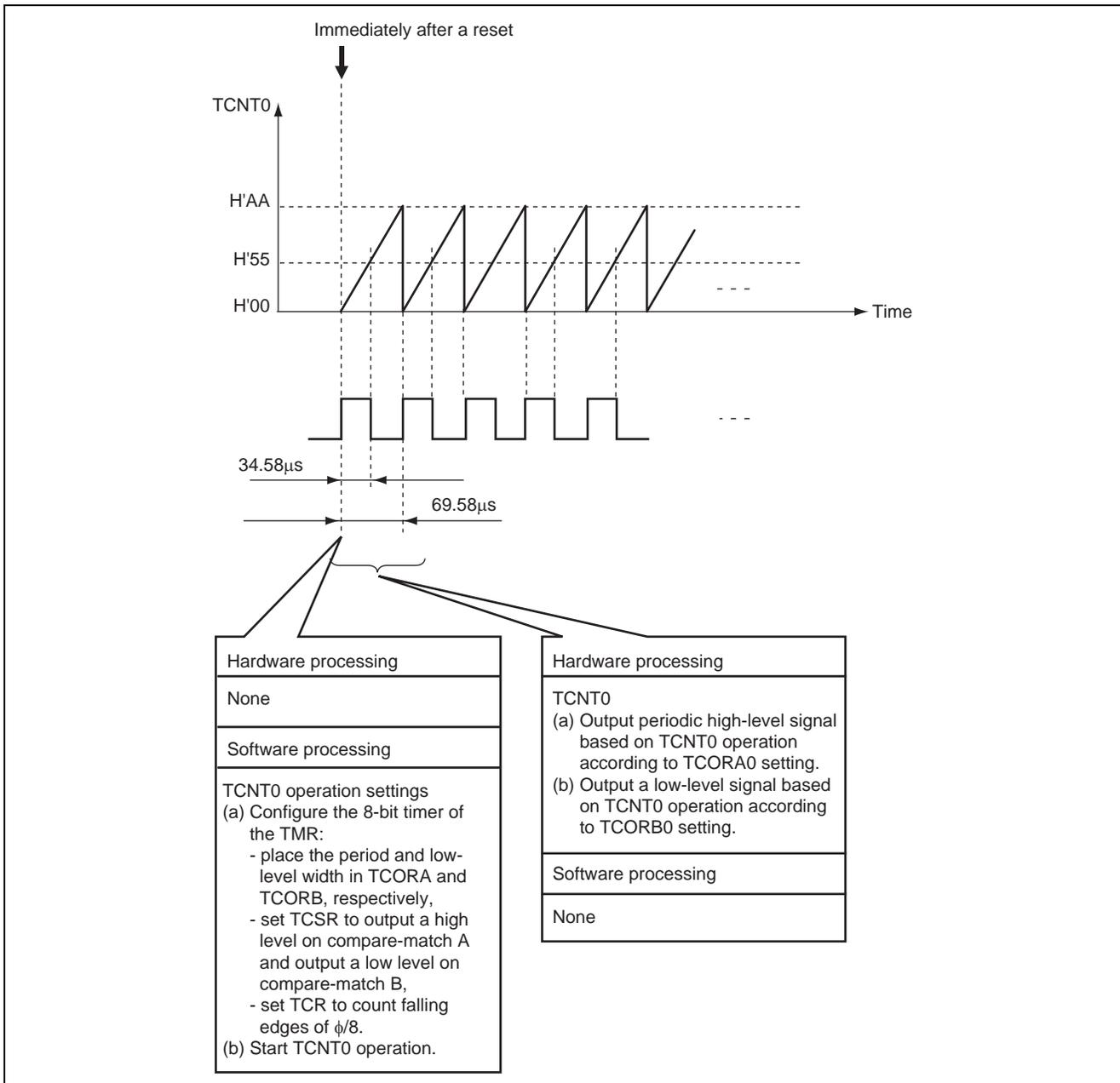
Figure 3 Output of Pulses with a Specified Duty Cycle Using 8-Bit Timer
