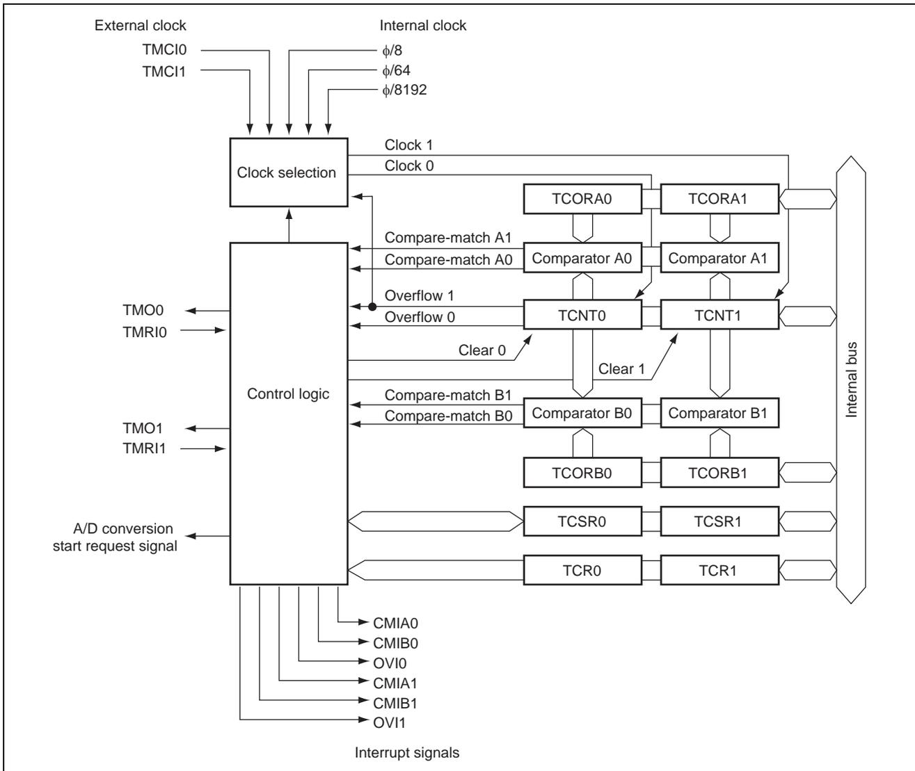
Figure 2 Block Diagram of 8-Bit Timer
