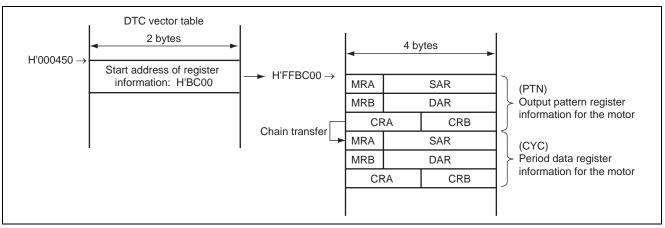
Figure 3 Example of DTC Vector Table and Memory Allocation
