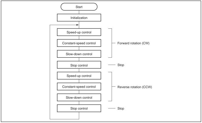
Figure 7 Flowchart of Stepping Motor Control
