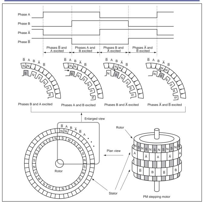
Figure 4 Example of Stepping Motor Operation
