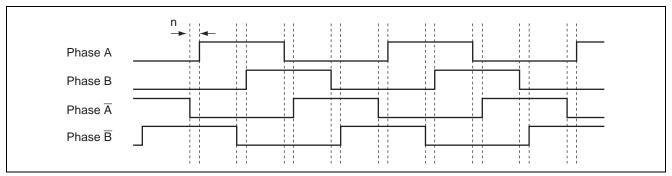
Figure 5 Example of Output with Non-Overlap Time
