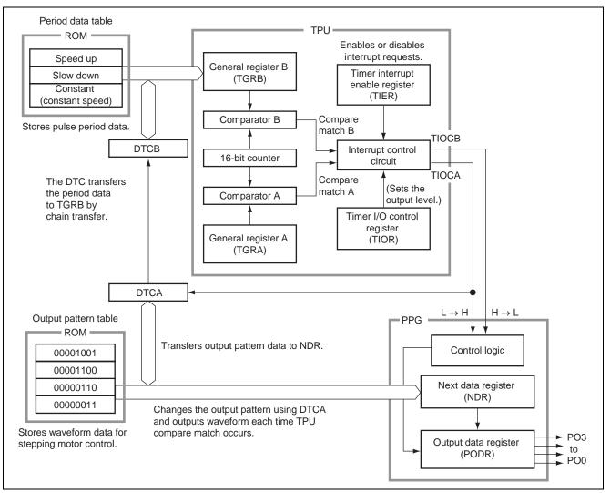
Figure 2 H8S/2377's Functions Used in This Application
