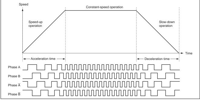
Figure 6 Speed-Up and Slow-Down Operations
