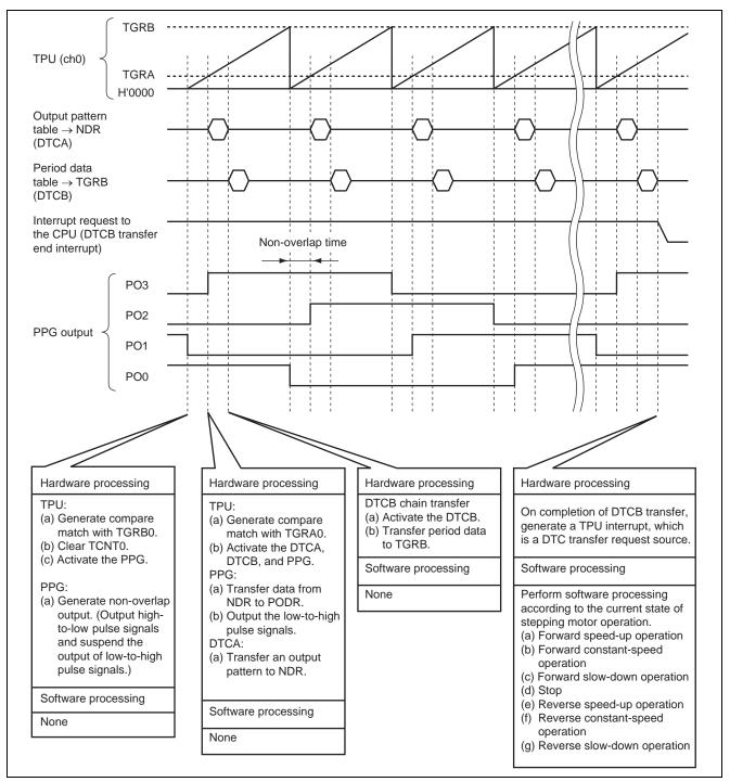
Figure 8 Timing of Stepping Motor Operation
