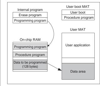
(2) The procedure program in the on-chip RAM then downloads the internal program (for erasing) into the on-chip RAM, which subsequently erases the flash memory in the specified block area.
