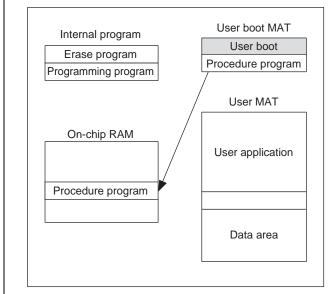
(3) The procedure program in the on-chip RAM downloads the internal program (programming program) into the on-chip RAM, stores the programming data received from the programming tool into the on-chip RAM on a single occasion, and writes the data in 128-byte blocks from the specified start address.
