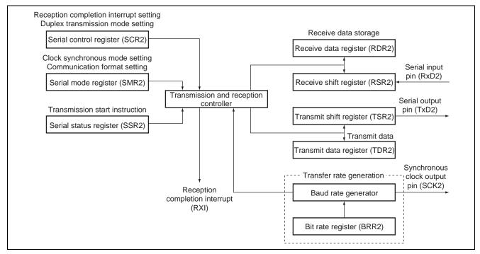
Figure 2 SCI Block Diagram
