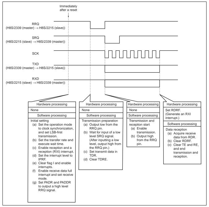
Figure 3 Principles of Operations Used for Duplex Transmission
