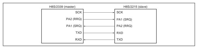
Figure 1 Block Diagram of Clock Synchronous SCI by H8S/2339
