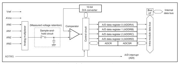
Figure 2 A/D Converter Block Diagram
