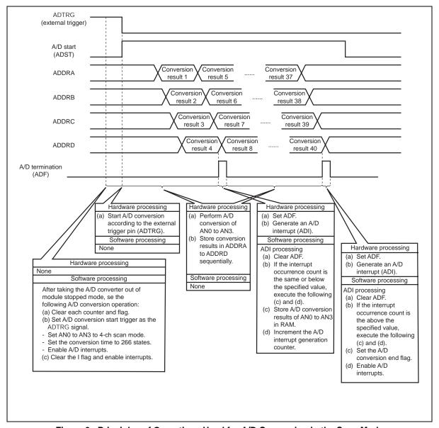
Figure 3 Principles of Operations Used for A/D Conversion in the Scan Mode
