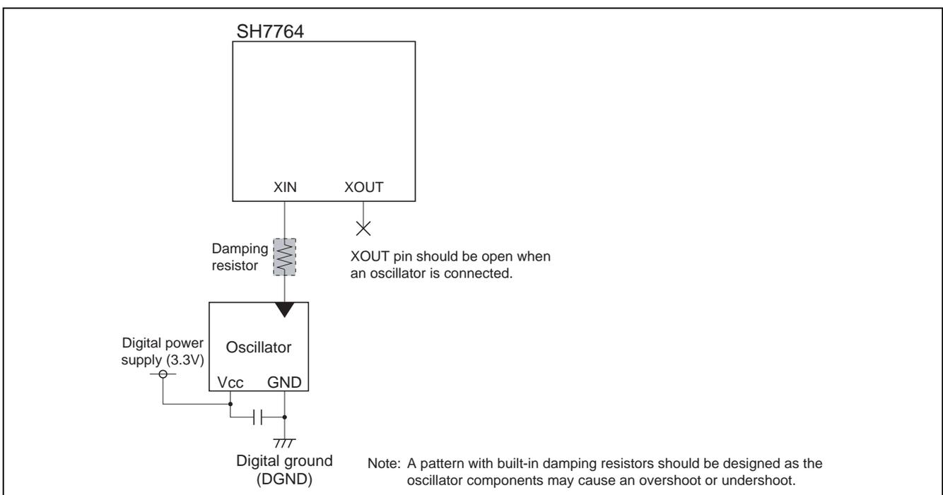
Figure 5 Example of the Oscillator Connection
