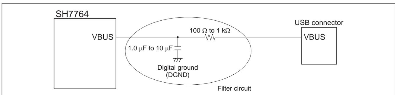
Figure 7 Example of the Function Controller VBUS Power Supply Circuit
