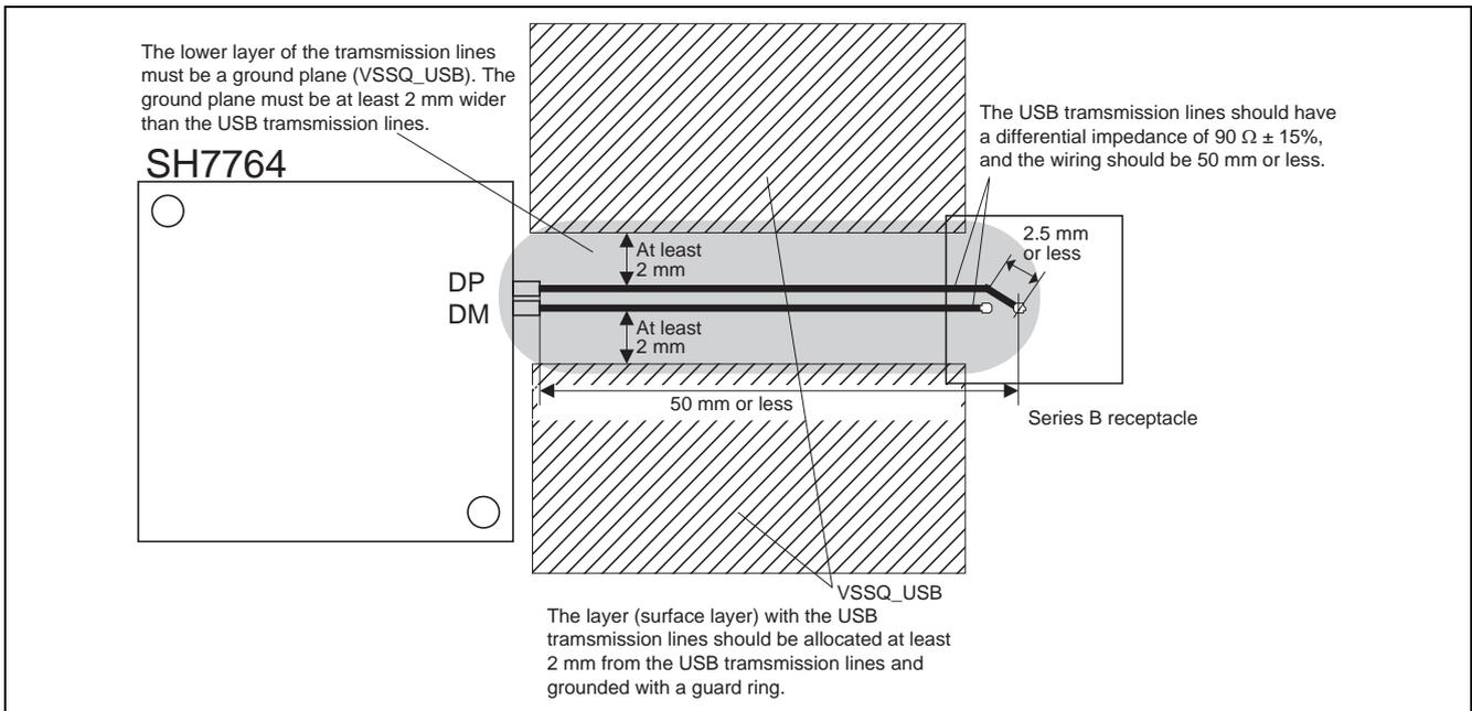
Figure 2 Design Example of the Function Controller USB Transmission Line Pattern
