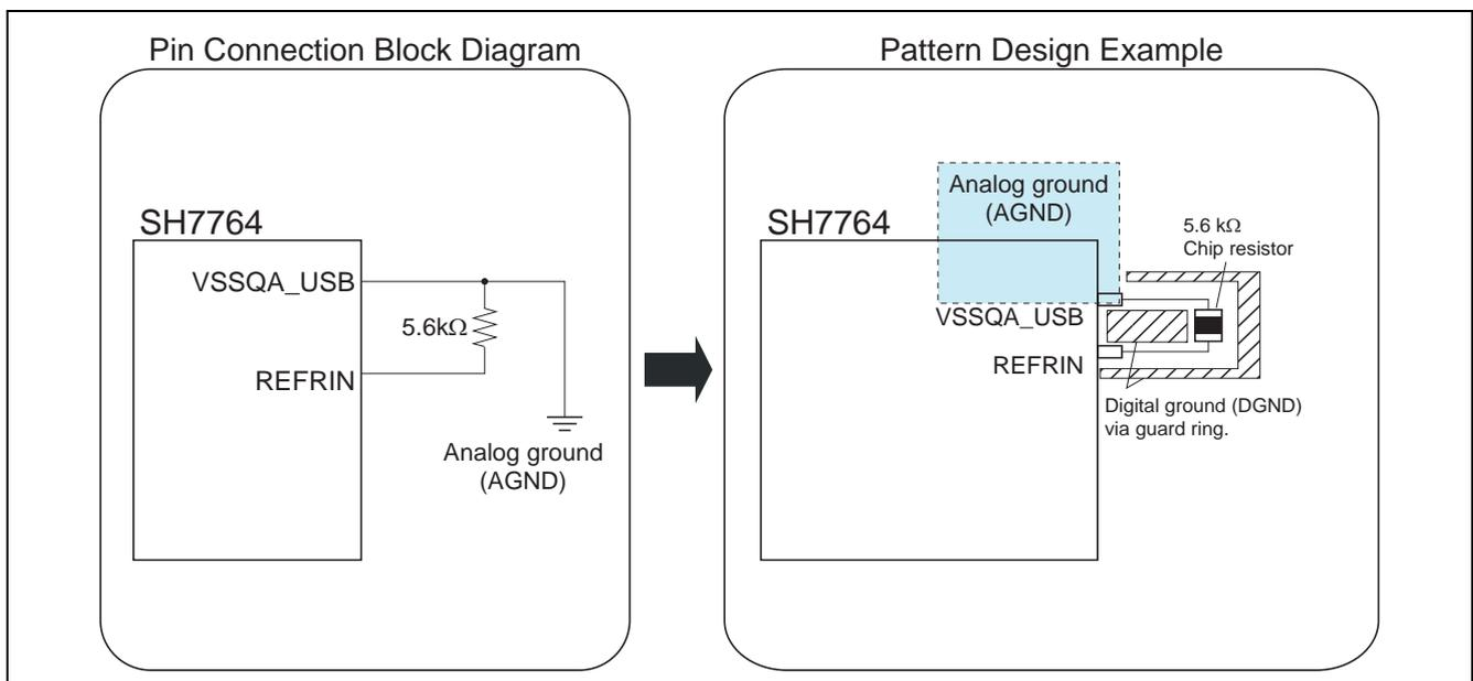
**Figure 8 Pin Connection and Design Example of the Pattern Around the REFRIN Pin**
