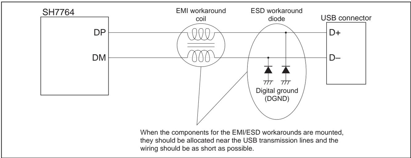
Figure 9 Connection Example When Components for EMI/ESD Workarounds are Used
