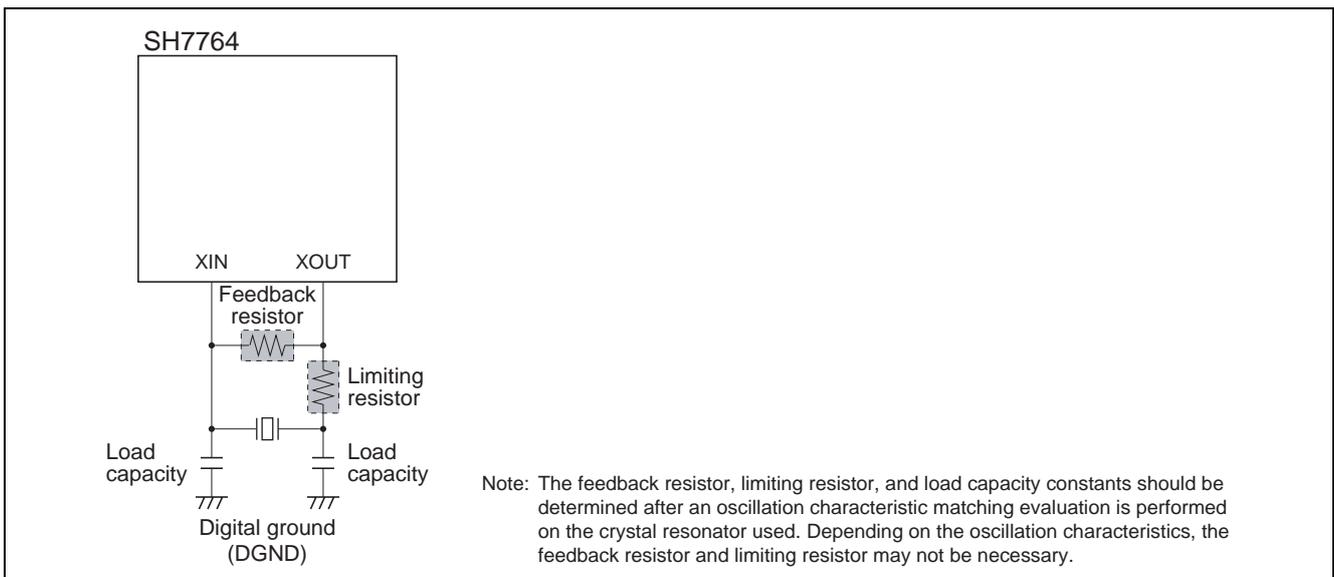
Figure 4 Example of the Crystal Resonator Connection
