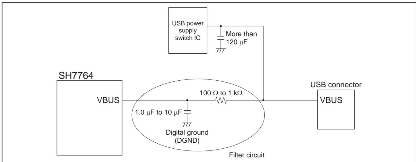
Figure 6 Example of the Host Controller VBUS Power Supply Circuit
