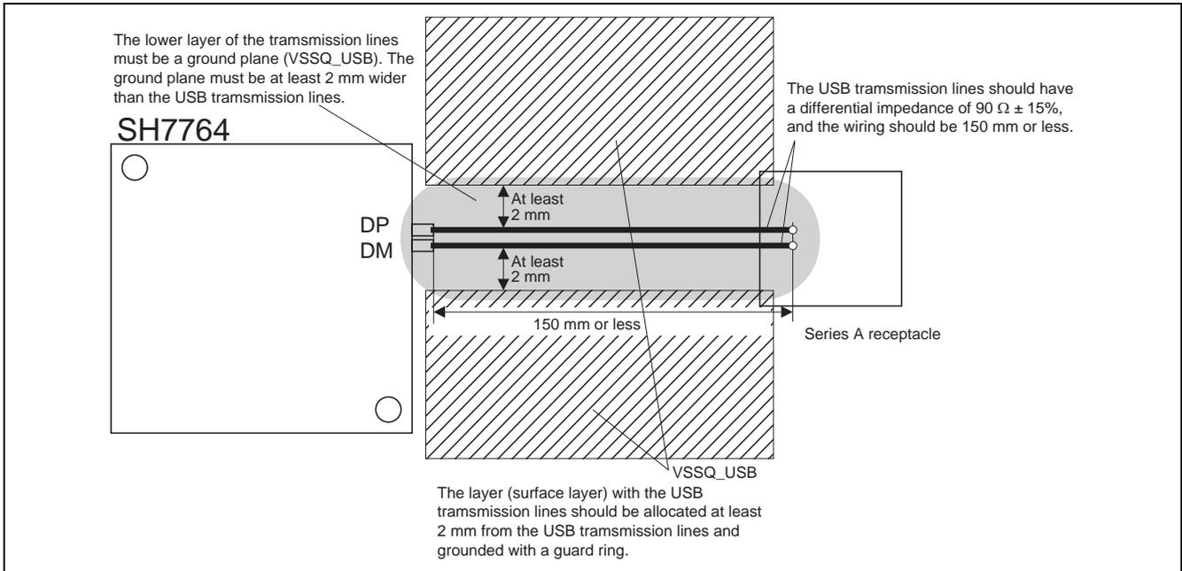
Figure 1 Design Example of the Host Controller USB Transmission Line Pattern
