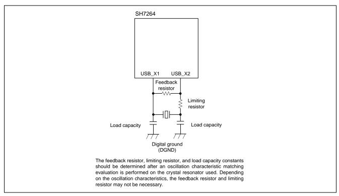
Figure 4 Example of the Crystal Resonator Connection
