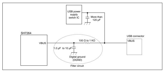
Figure 6 Example of the Host Controller VBUS Power Supply Circuit
