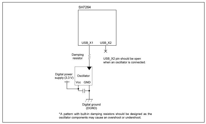
Figure 5 Example of the Oscillator Connection
