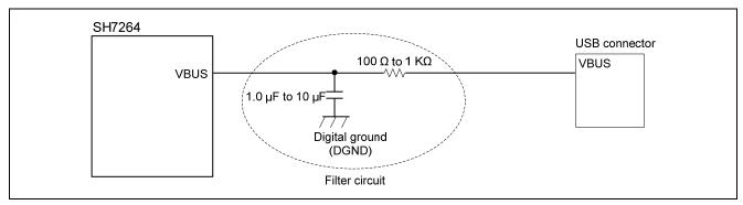
Figure 7 Example of the Function Controller VBUS Power Supply Circuit
