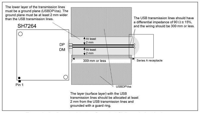
Figure 1 Design Example of the Host Controller USB Transmission Line Pattern
