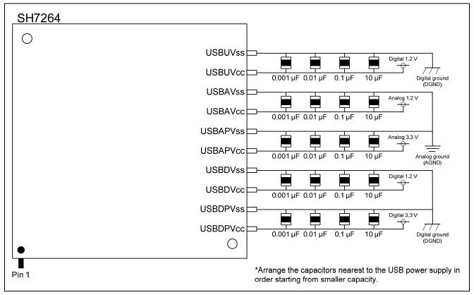
Figure 3 Example of the Decoupling Capacitor Allocation
