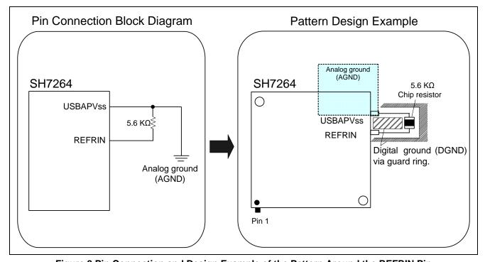
Figure 8 Pin Connection and Design Example of the Pattern Around the REFRIN Pin
