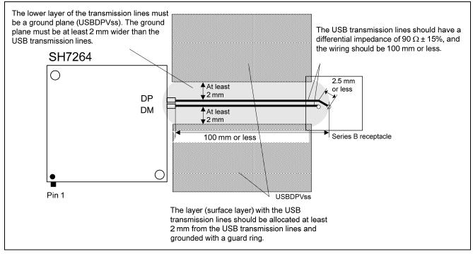
Figure 2 Design Example of the Function Controller USB Transmission Line Pattern
