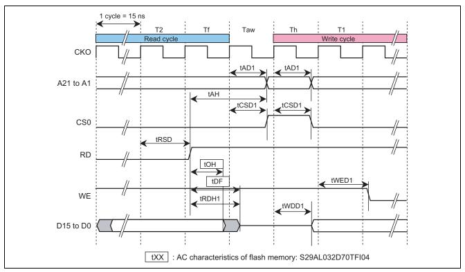
Figure 10 Timing between Read and Write Cycles for Flash Memory
