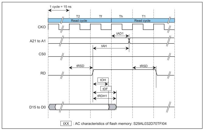
Figure 11 Timing between Read and Read Cycles for Flash Memory
