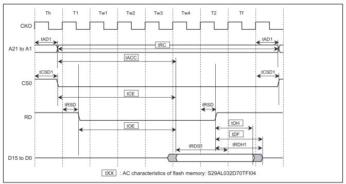
Figure 5 Read Timing for Flash Memory (tRSD = Min.)
