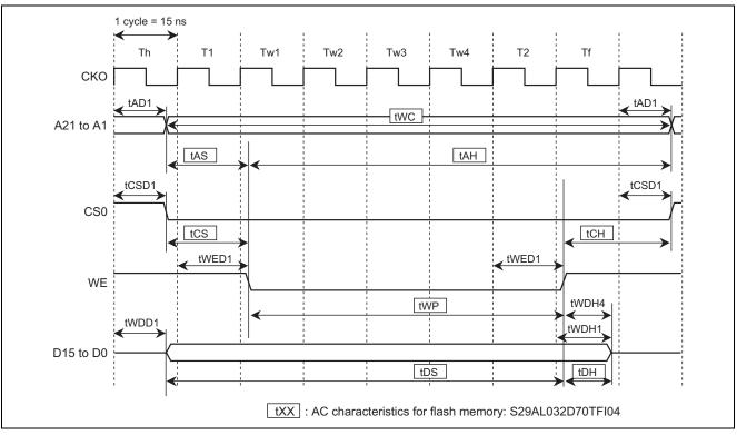
Figure 7 Write Timing for Flash Memory
