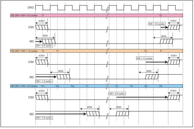
(Setting of the SW or HW bits - 0.5) number of cycles
