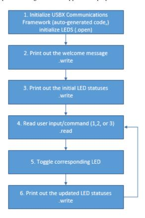
Figure 4 Communications Framework Application Project Flow Diagram
