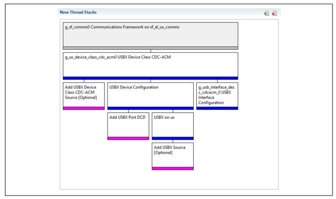
Figure 2 Communications Framework on USBX Module Stack
