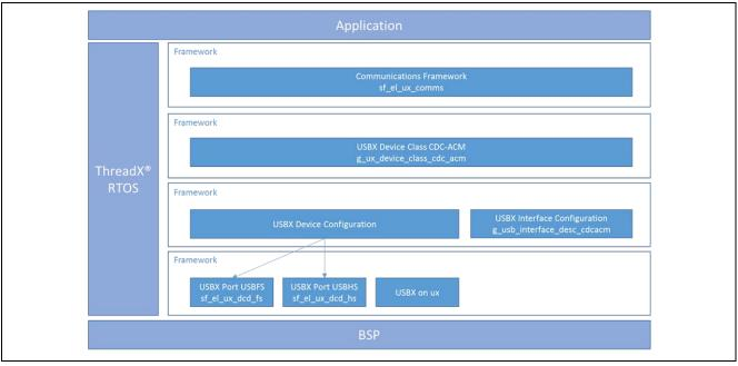
Figure 1 Communications Framework on USBX Module Block Diagram
