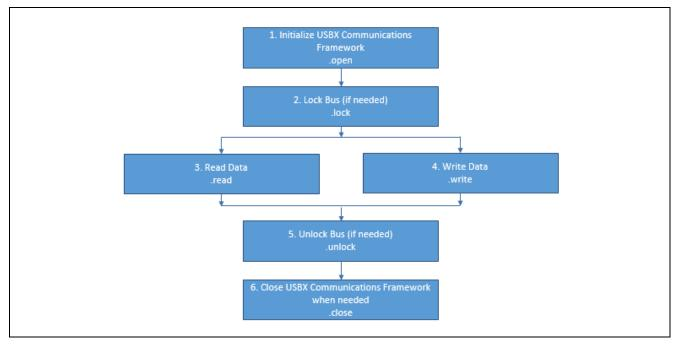
Figure 3 Flow Diagram of a Typical Communications Framework on USBX Application
