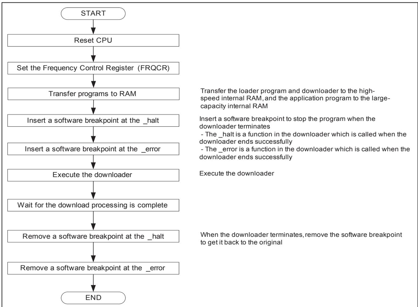
Figure 15 Command Batch File Flow Chart
