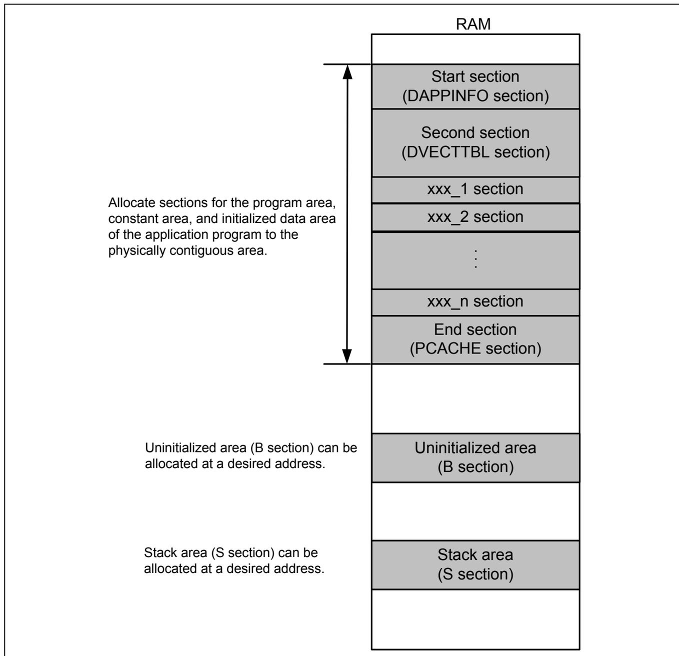
Figure 8 Application Program Section Alignment
