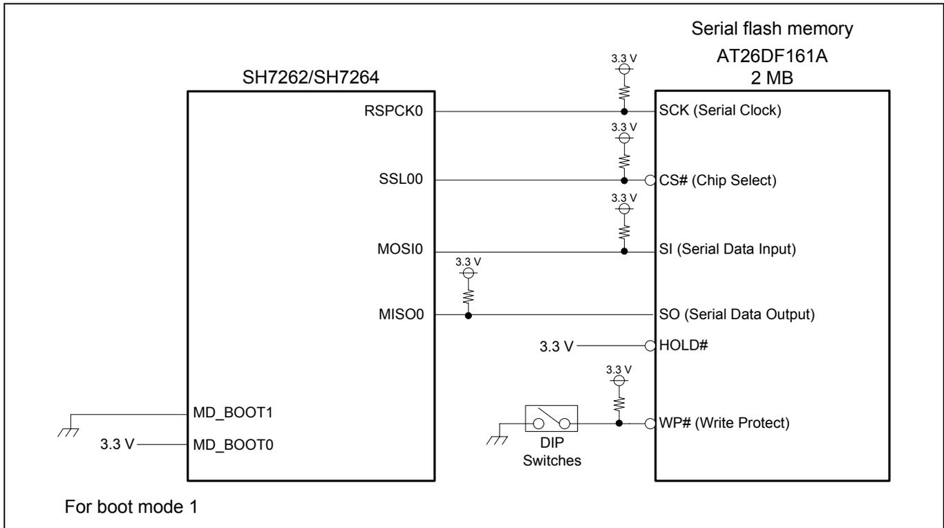
**Figure 4 Connection Circuit for the SH7264 and Serial Flash Memory**
