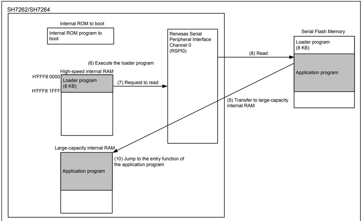
Figure 2 Operation Image of the Loader Program
