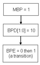
Once a zero-to-one transition is created on BPE bit, the entire Connection Memory block will be initialized in 2 frames  $(2x125\mu s = 250\mu s)$ . The initialization process put A[15:14] = BPD[1:0], A[13:0] = 0x0000 in every single locations in Connection Memory block. By completion, the device will reset BPD[1:0] = 00.
