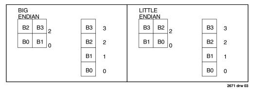
Figure 1c. Little-endian and Big-endian Byte Mapping Between 16-bit and 8-bit Buses — Bo, B1, B2 and B3 are Bytes Within the 16-bit and 8-bit Words
