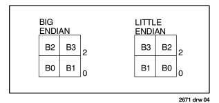
Figure 1d. Little-endian and Big-endian Byte Mapping Between 16-bit Buses — B0, B1, B2 and B3 are Bytes Within the 16-bit Words
