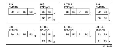
Figure 1a. Little-endian and Big-endian Byte Mapping Between 32-bit and 16-bit Buses — Bo, B1, B2 and B3 are Bytes Within the 32-bit and 16-bit Words
