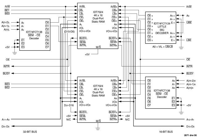
Figure 3. An Interface to Connect a 32-Bit Bus to a 16-Bit Bus
