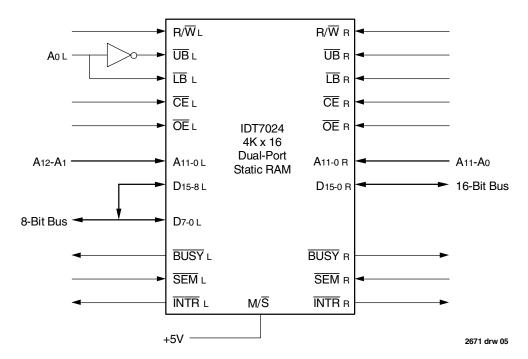
Figure 2. An Interface to Connect 8- and 16-Bit Buses
