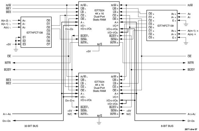
Figure 4. An Interface to Connect a 32-Bit Bus to an 8-Bit Bus
