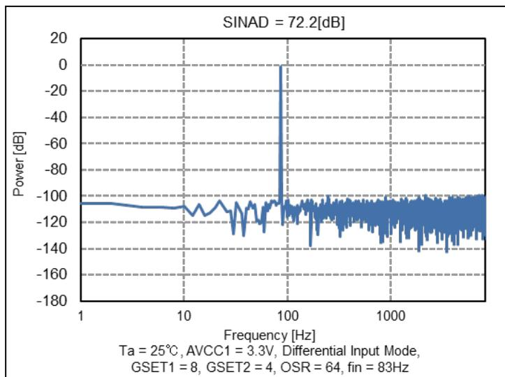
Figure 16. Power versus Frequency ( $G_{SET1} = 8$ ,  $G_{SET2} = 4$ , OSR = 64)
