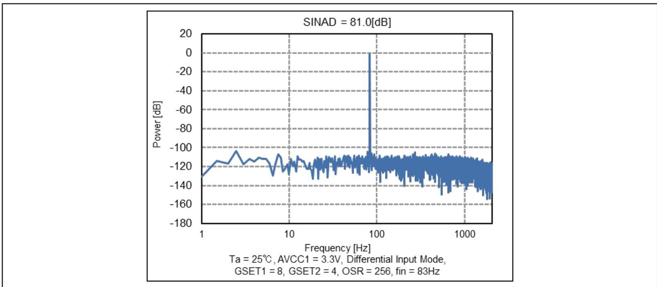
Figure 17. Power versus Frequency ( $G_{SET1} = 8, G_{SET2} = 4, OSR = 256$ )
