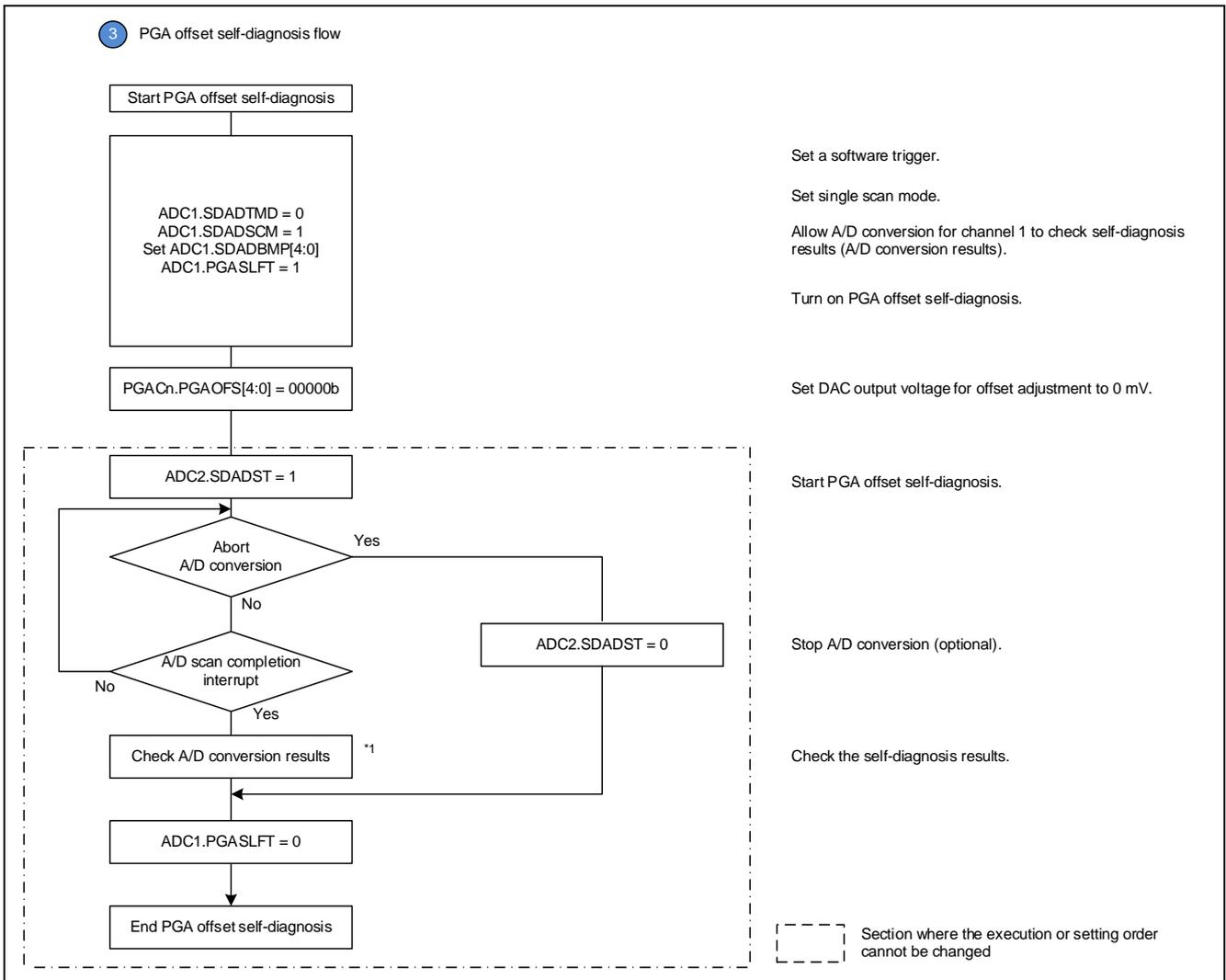
Figure 28. Self-diagnosis Flow for PGA Offset
