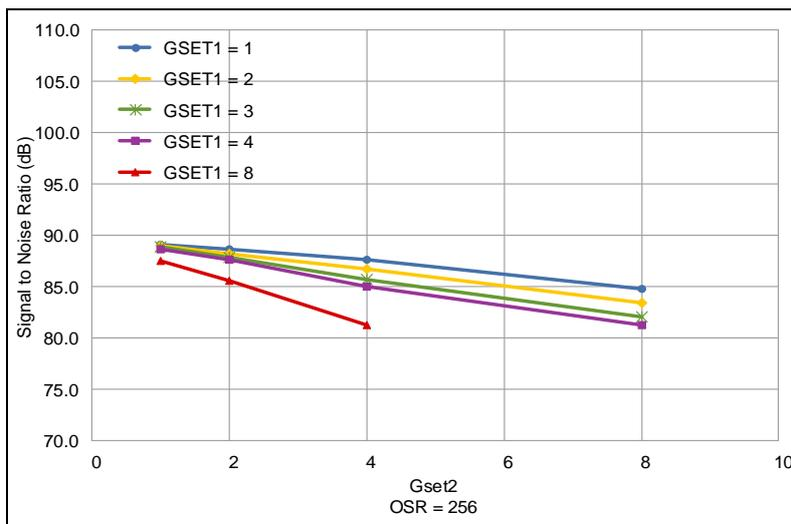
Figure 10. Dependence of SNR on G<sub>SET2</sub>
