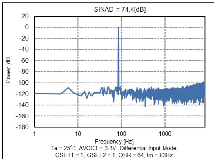
Figure 13. Power versus Frequency (G<sub>SET1</sub> = 1, G<sub>SET2</sub> = 1, OSR = 64)
