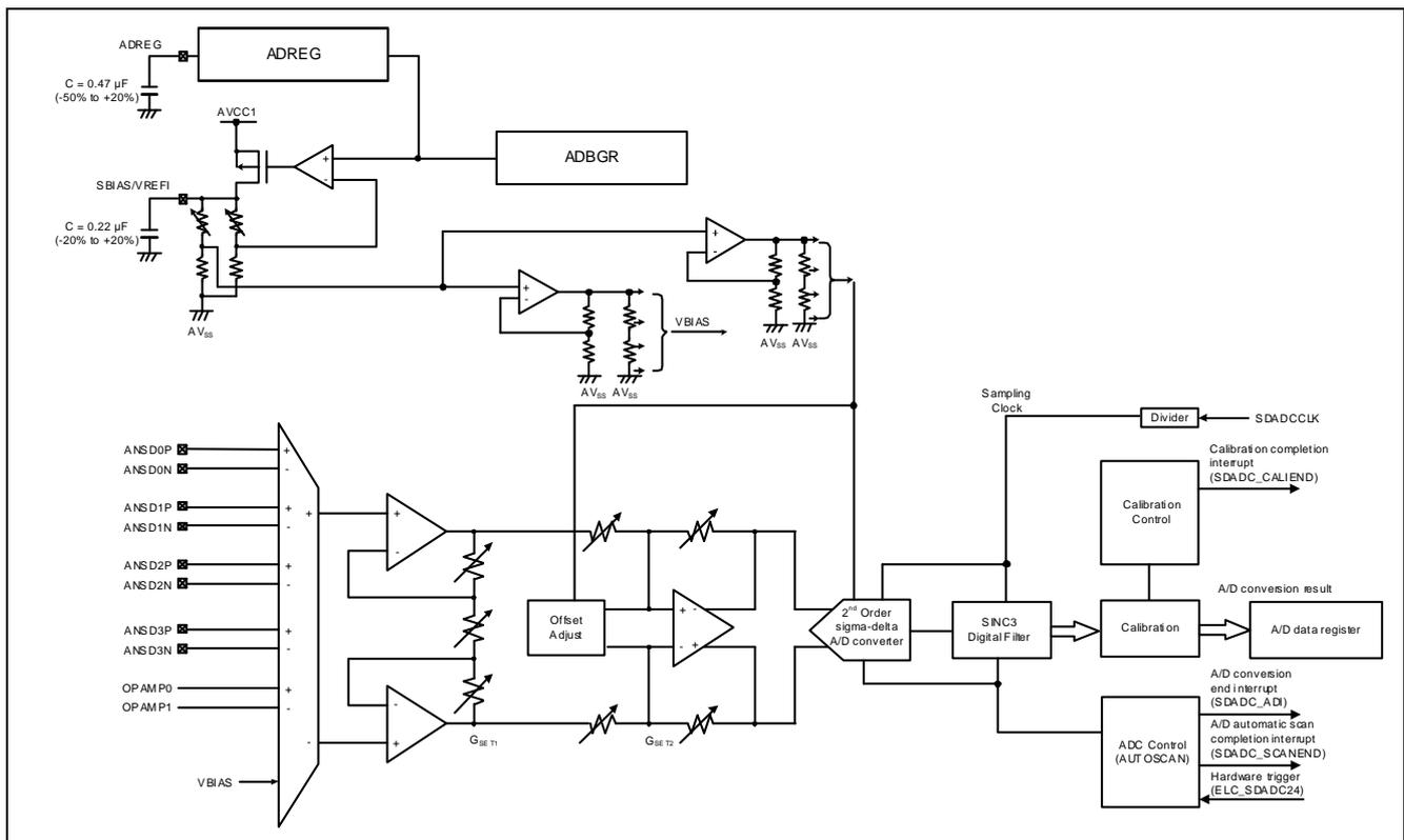
Figure 1. SDADC24 Block Diagram
