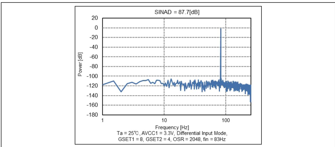
Figure 18. Power versus Frequency ( $G_{SET1} = 8, G_{SET2} = 4, OSR = 2048$ )
