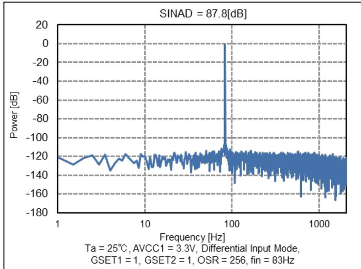
Figure 14. Power versus Frequency ( $G_{SET1} = 1$ ,  $G_{SET2} = 1$ , OSR = 256)
