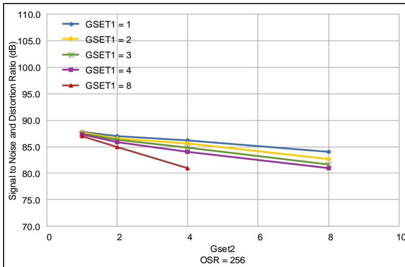
Figure 12. Dependence of SINAD on G<sub>SET2</sub>
