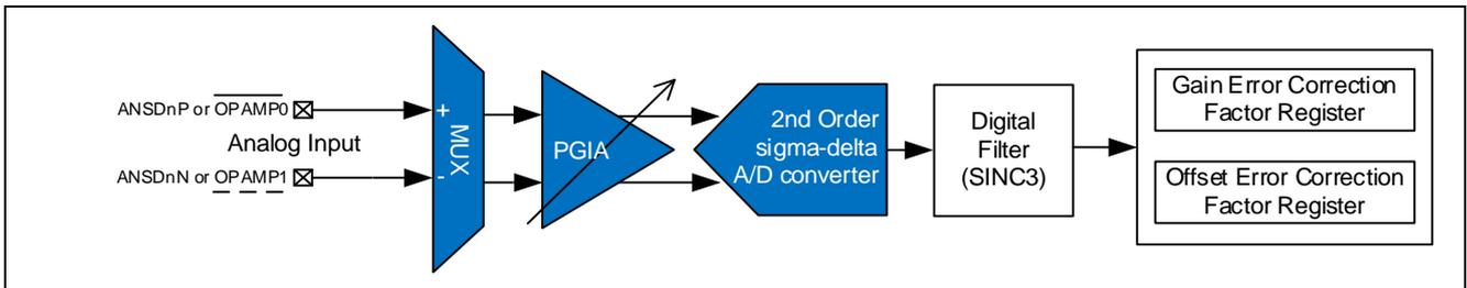
**Figure 24. External Calibration**
