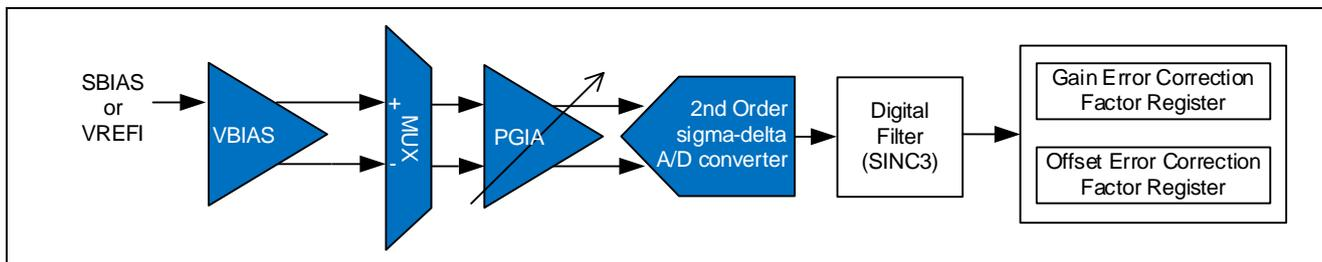
**Figure 23. Internal Calibration**
