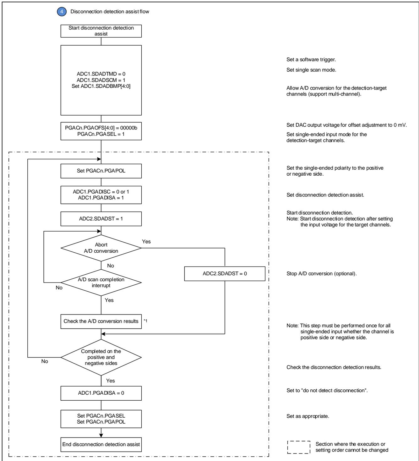
**Figure 29. Disconnection Detection Assist Flow**
