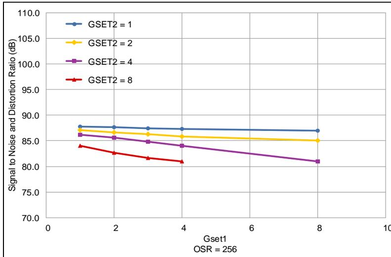
Figure 11. Dependence of SINAD on G<sub>SET1</sub>
