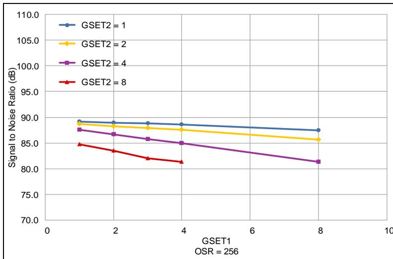
Figure 9. Dependence of SNR on G<sub>SET1</sub>
