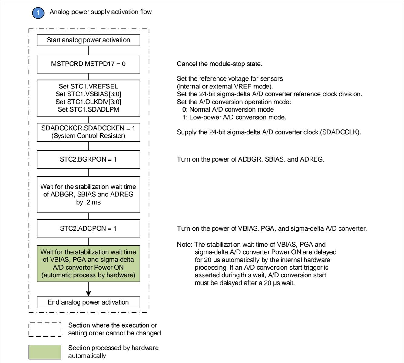
Figure 26. Analog Power Supply Activation Flow
