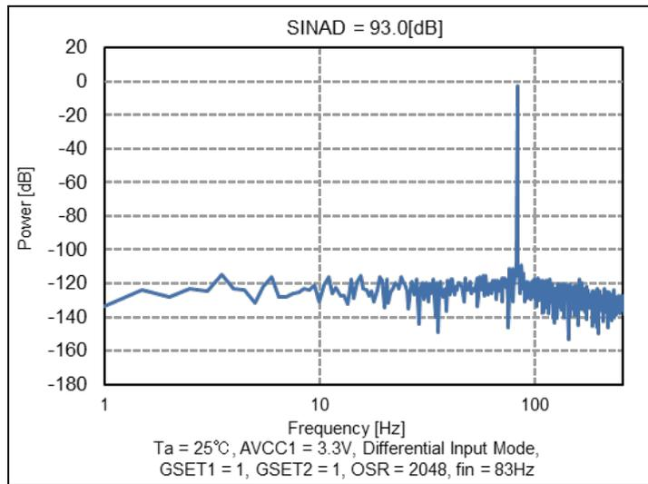
Figure 15. Power versus Frequency ( $G_{SET1} = 1$ ,  $G_{SET2} = 1$ , OSR = 2048)
