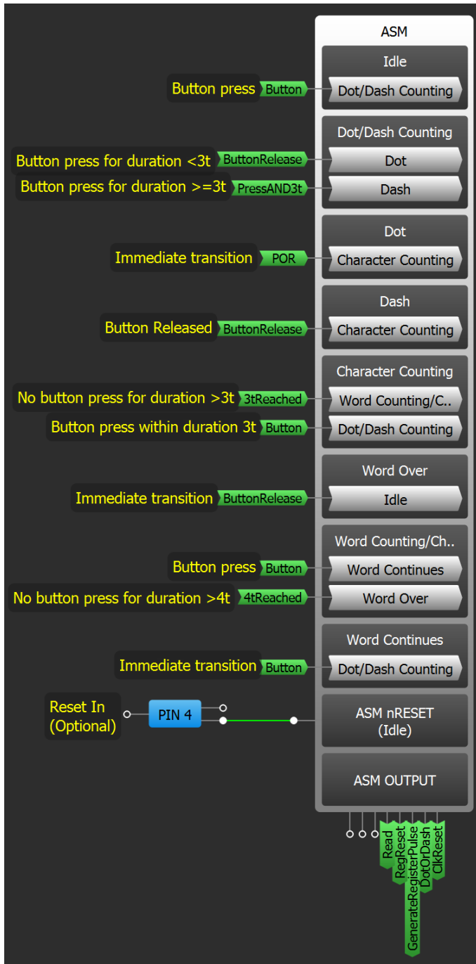
Figure 5. State transition signals of the ASM. The ASM nRESET input returns the ASM to the Idle state when it goes LOW. For testing purposes, this is controlled with an external button
