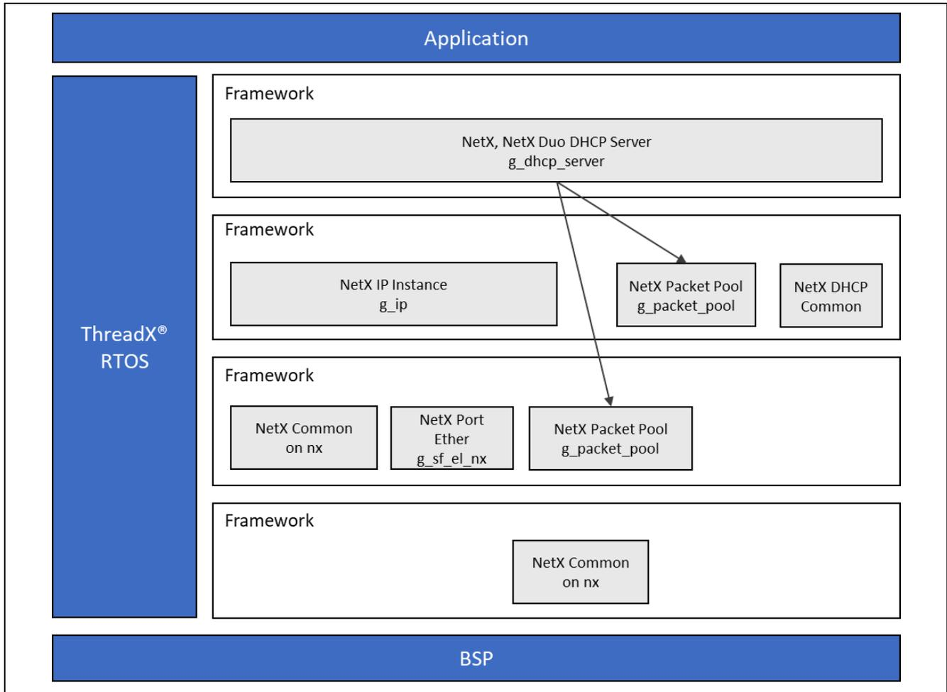
Figure 1. NetX DHCP Server Module Block Diagram
