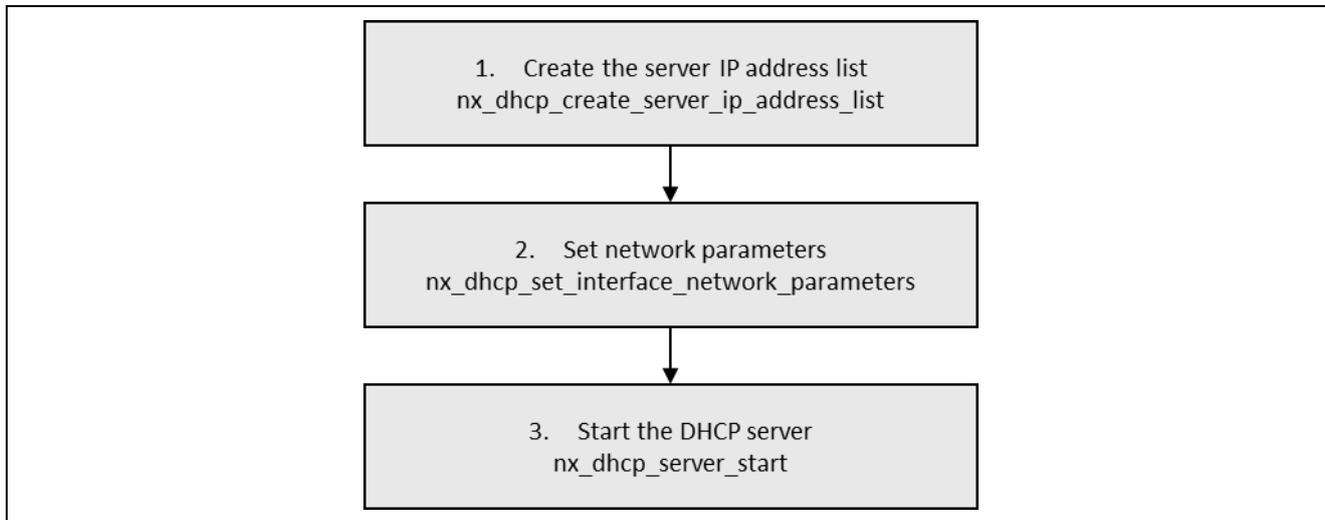
**Figure 3. Flow Diagram of a Typical NetX DHCP Server Module Application**
