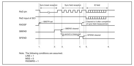
Figure 16.8 Example of Operation in the Reception of a Header Field
