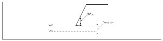
Figure 25.1 Rising of Vcc Power Supply
