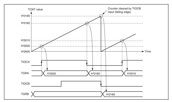
Figure 10.10 Example of Input Capture Operation
