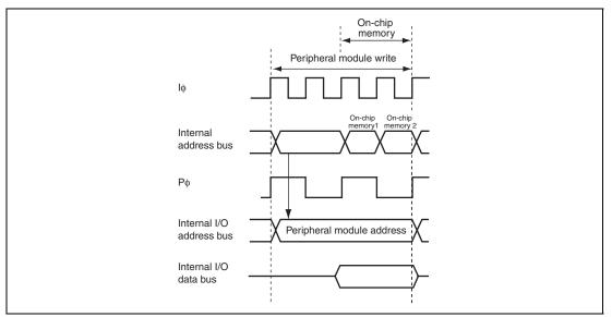
Figure 6.3 Example of Timing when Peripheral Module Write Data Buffer Function is Used
