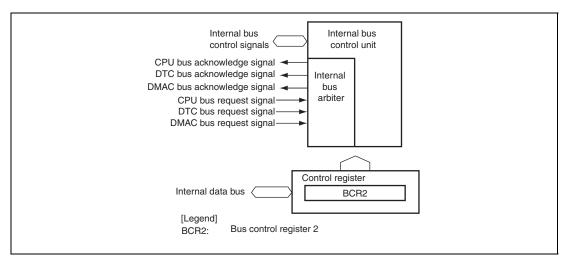
Figure 6.1 Block Diagram of Bus Controller
