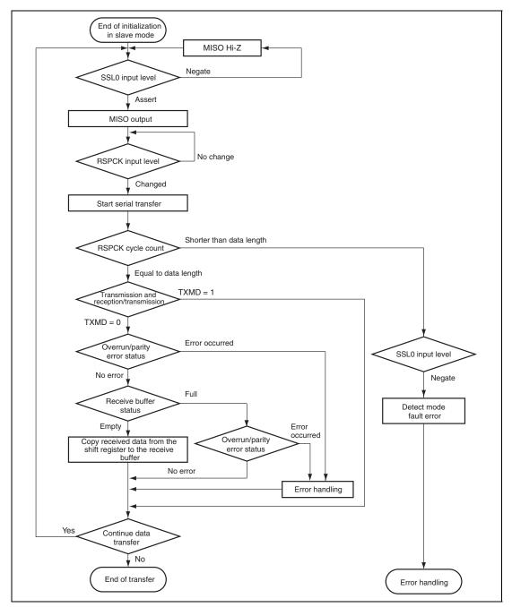
Figure 15.32 Transfer Operation Flowchart in Slave Mode (CPHA = 1)
