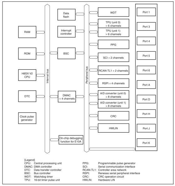
Figure 1.1 Block Diagram of H8SX/1725S and H8SX/1727S
