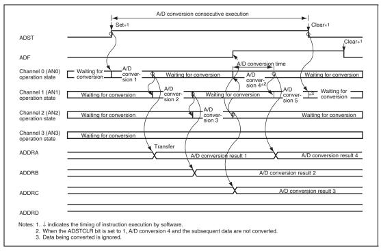
Figure 18.4 Example of A/D Converter Operation (Scan Mode, Three Channels (AN0 to AN2) Selected)
