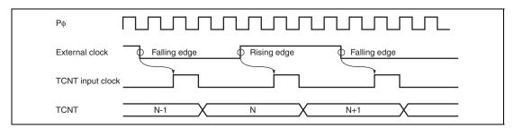
Figure 10.32 Count Timing in External Clock Operation
