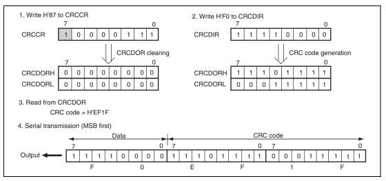
Figure 17.3 MSB-First Data Transmission
