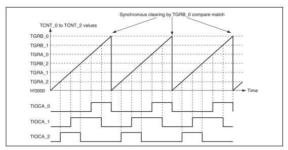
Figure 10.12 Example of Synchronous Operation
