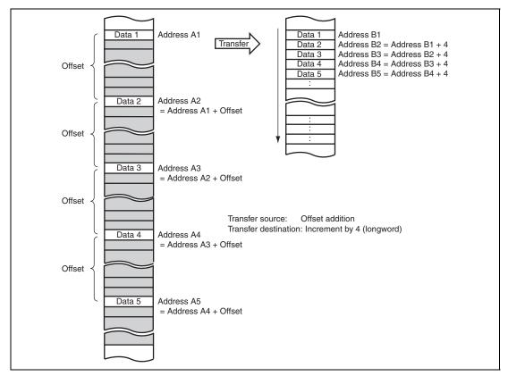
Figure 7.18 Operation of Offset Addition
