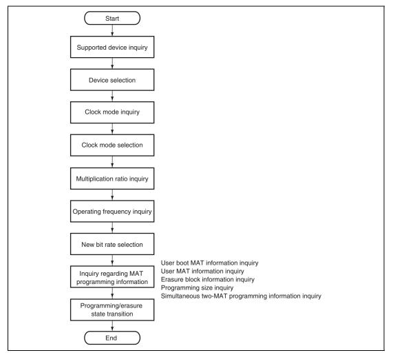
Figure 20.9 Example of Procedure to Use Inquiry/Selection Host Commands
