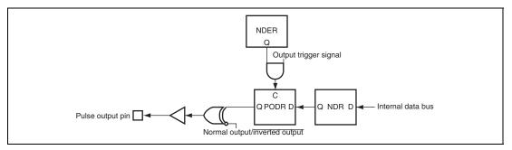
Figure 11.2 Schematic Diagram of PPG
