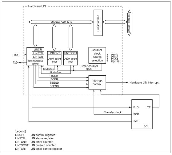
Figure 16.1 Block Diagram of Hardware LIN
