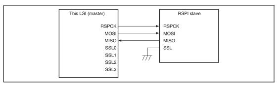
Figure 15.3 Single-Master/Single-Slave Configuration Example (This LSI = Master)
