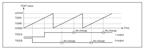
Figure 10.7 Example of 0-Output/1-Output Operation
