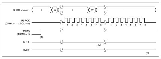
Figure 15.22 Operation Example of TXMD = 1
