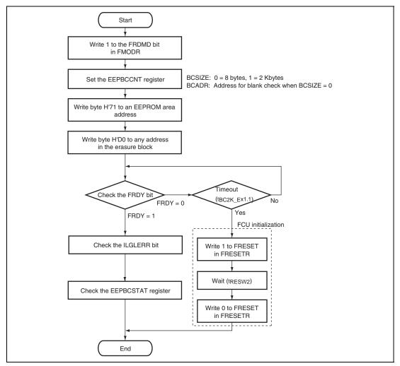
Figure 21.7 Procedure for EEPROM Blank Check
