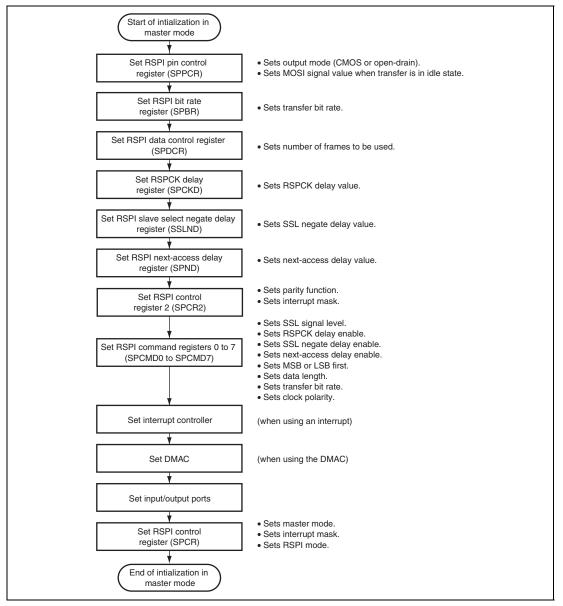
Figure 15.34 Example of Initialization Flowchart in Master Mode
