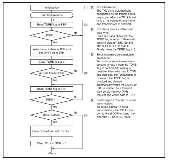
Figure 13.11 Sample Multiprocessor Serial Transmission Flowchart
