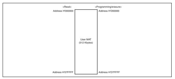
Figure 20.1 Memory MAT Configuration in Flash Memory
