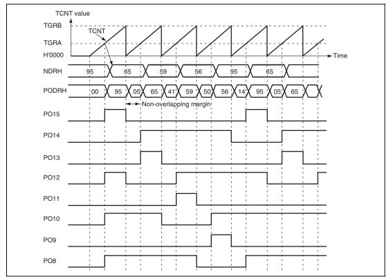
Figure 11.9 Non-Overlapping Pulse Output Example (4-Phase Complementary)
