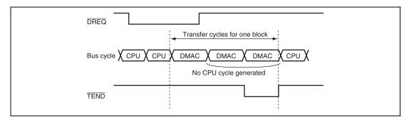
Figure 7.10 Operations in Block Transfer Mode
