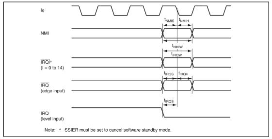
Figure 25.13 Interrupt Input Timing
