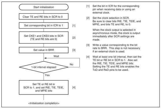
Figure 13.5 Sample SCI Initialization Flowchart
