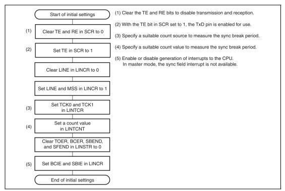
Figure 16.3 Example of Initial Settings in Master Mode
