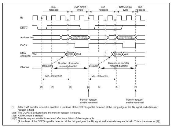
Figure 7.37 Example of Transfer in Single Address Mode Activated by  $\overline{DREQ}$  Low Level
