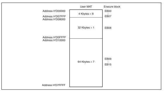
Figure 20.3 Block Configuration of User MAT
