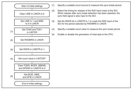
Figure 16.9 Example of Initial Settings in Slave Mode
