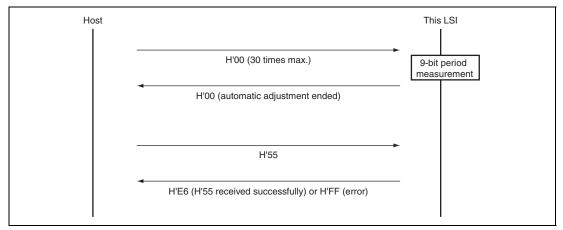
Figure 20.8 Communication Sequence between Host and this LSI
