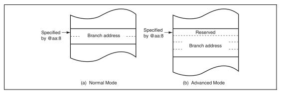
Figure 2.15 Branch Address Specification in Memory Indirect Mode
