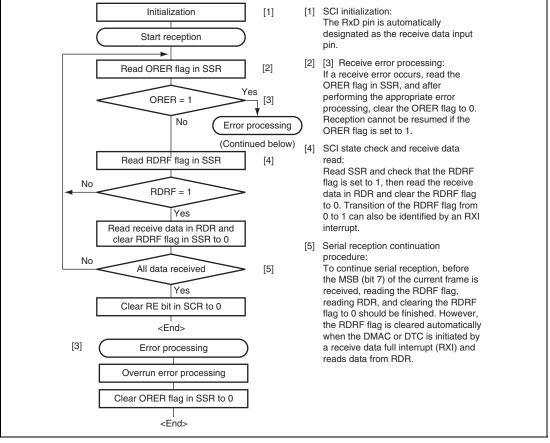
Figure 13.19 Sample Serial Reception Flowchart
