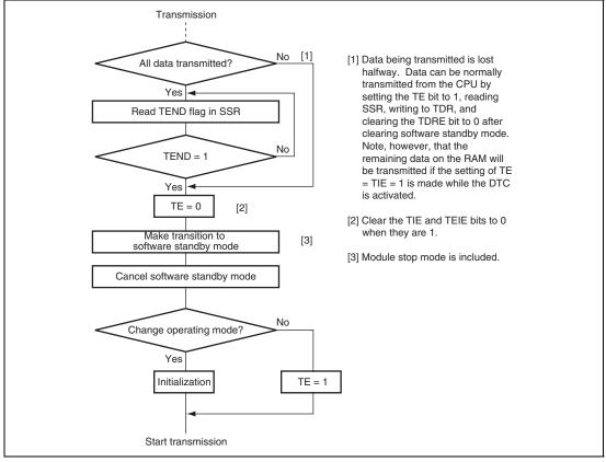
Figure 13.22 Sample Flowchart for Mode Transition during Transmission
