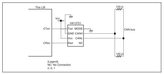
Figure 14.28 High-Speed CAN Interface Using HA13721
