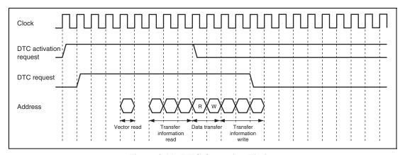
Figure 8.11 DTC Operation Timing (Example of Short Address Mode in Normal Transfer Mode or Repeat Transfer Mode)
