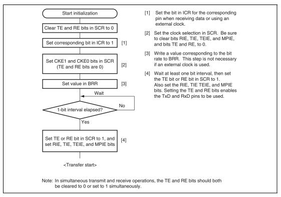
Figure 13.15 Sample SCI Initialization Flowchart
