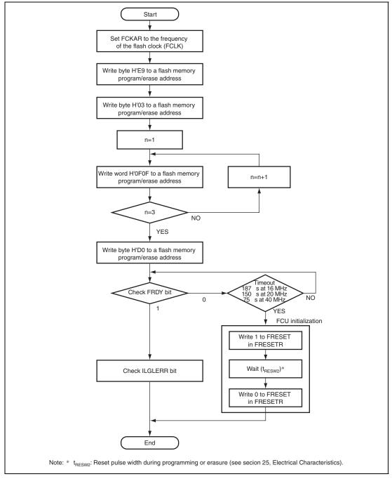
Figure 20.19 Procedure for Issuing Flash Clock Notification Command
