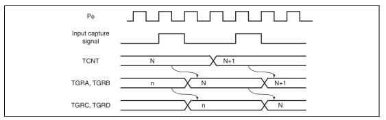
**Figure 10.38 Buffer Operation Timing (Input Capture)**
