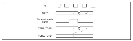
**Figure 10.37 Buffer Operation Timing (Compare Match)**
