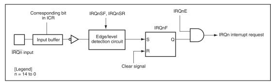
Figure 5.2 Block Diagram of Interrupts IRQn
