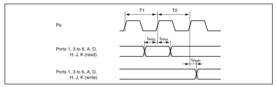
Figure 25.14 I/O Port Input/Output Timing
