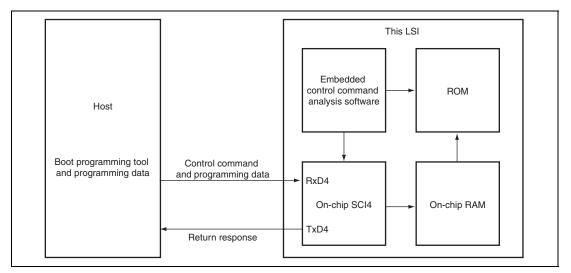
Figure 20.5 System Configuration in Boot Mode
