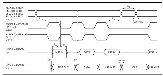
Figure 25.24 RSPI Timing (Master, CPHA = 1)
