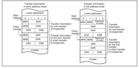
Figure 8.2 Transfer Information on Data Area
