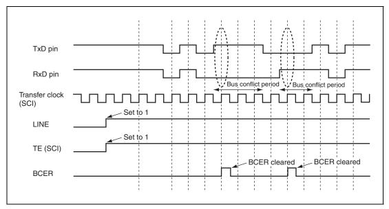
Figure 16.14 Example of Operation When a Bus Conflict is Detected
