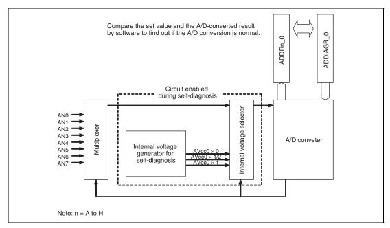
Figure 18.10 Overview of Self-Diagnosis of the A/D Converter
