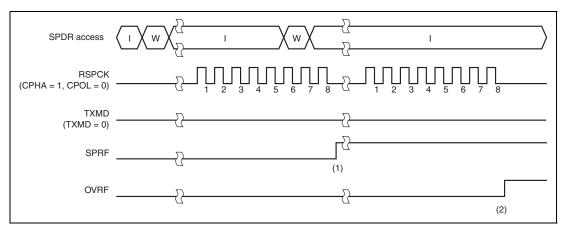
Figure 15.21 Operation Example of TXMD = 0
