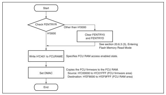
Figure 20.15 Procedure for Firmware Transfer to FCU RAM
