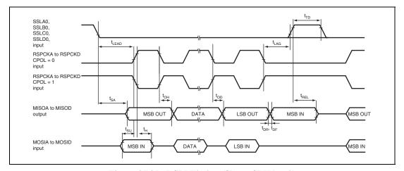
Figure 25.25 RSPI Timing (Slave, CPHA = 0)
