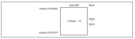
Figure 21.3 Block Configuration of Data MAT
