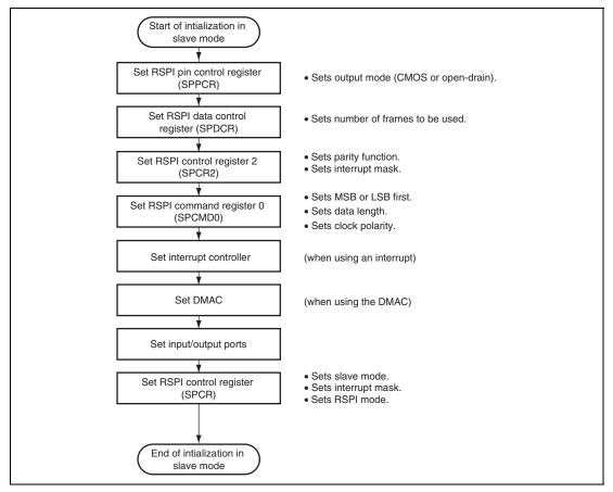
Figure 15.36 Example of Initialization Flowchart in Slave Mode
