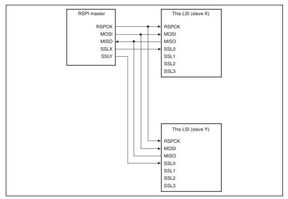
Figure 15.7 Single-Master/Multi-Slave Configuration Example (This LSI = Slave)
