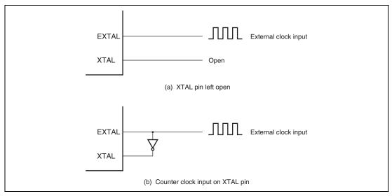
Figure 22.4 External Clock Input (Examples)
