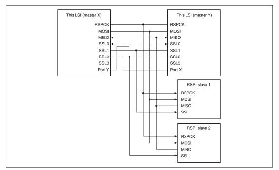
Figure 15.8 Multi-Master/Multi-Slave Configuration Example (This LSI = Master)
