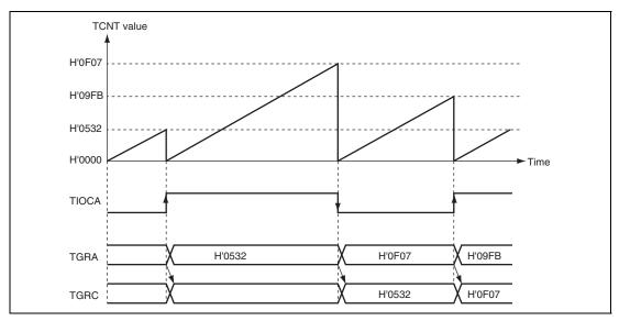
Figure 10.17 Example of Buffer Operation (2)
