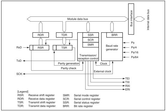
Figure 13.1 Block Diagram of SCI
