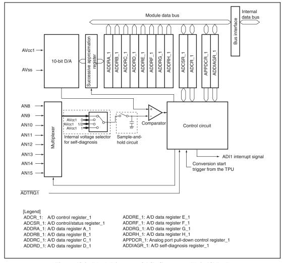
Figure 18.2 Block Diagram of A/D Converter (Unit 1/AD 1)
