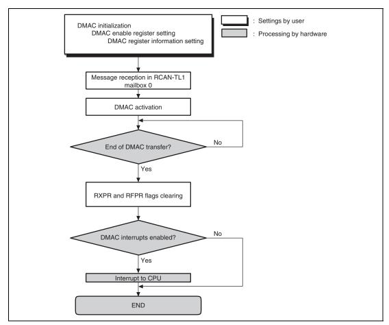
Figure 14.26 DMAC Transfer Flowchart
