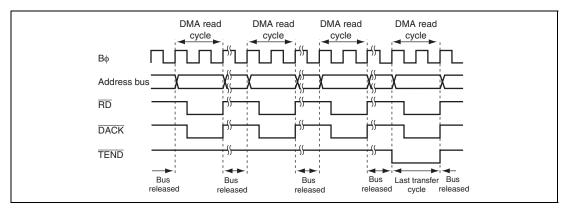
Figure 7.34 Example of Transfer in Single Address Mode (Byte Read)
