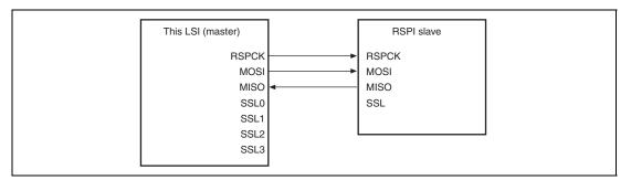
Figure 15.9 Master (Clock Synchronous Operation)/Slave (Clock Synchronous Operation)
