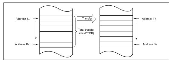
Figure 7.8 Operations in Normal Transfer Mode
