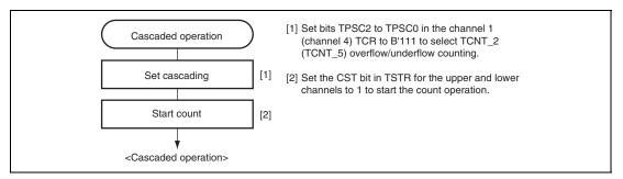
Figure 10.18 Example of Cascaded Operation Setting Procedure
