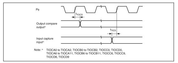
Figure 25.15 TPU Input/Output Timing
