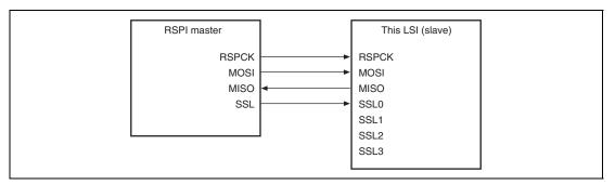
Figure 15.4 Single-Master/Single-Slave Configuration Example (This LSI = Slave)
