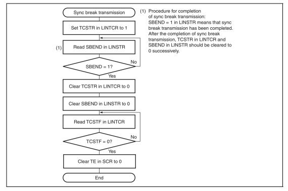
Figure 16.4 Example of Settings for Sync Break Transmission in Master Mode
