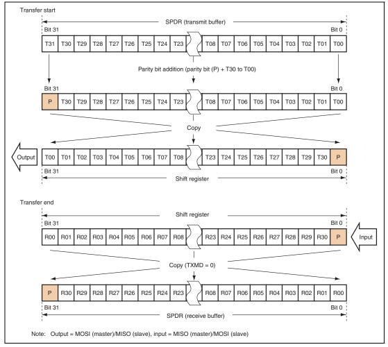
Figure 15.18 LSB First Transfer (32-Bit Data, Parity Function Enabled)
