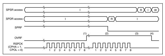
Figure 15.24 SPRF and OVRF Bit Operation Example
