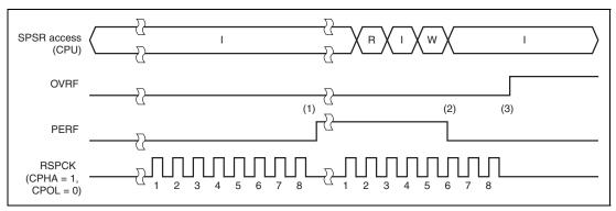
Figure 15.25 PERF Bit Operation Example
