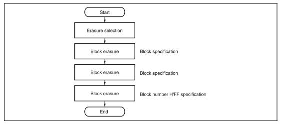
Figure 20.12 Procedure for Flash Memory Erasure in Boot Mode
