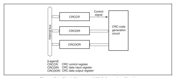
Figure 17.1 Block Diagram of CRC Operation Circuit
