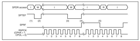
Figure 15.23 SPTEF and SPRF Bit Operation Example
