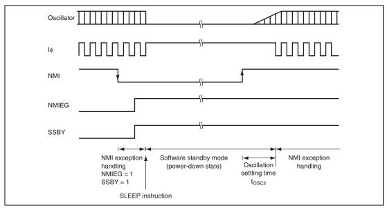
Figure 23.2 Software Standby Mode Application Example
