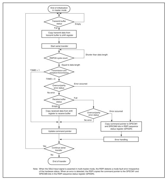
Figure 15.29 Transfer Operation Flowchart in Master Mode
