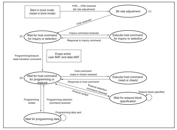
Figure 20.6 State Transition in Boot Mode
