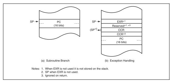
Figure 2.3 Stack Structure (Normal Mode)
