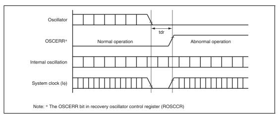
Figure 25.29 Timing of External Oscillation Stoppage Detection
