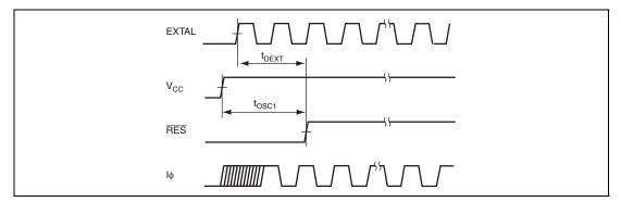
Figure 25.5 Oscillation Settling Timing
