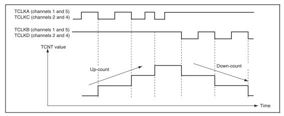
Figure 10.28 Example of Phase Counting Mode 3 Operation
