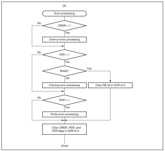
Figure 13.9 Sample Serial Reception Flowchart (2)
