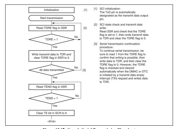
Figure 13.17 Sample Serial Transmission Flowchart
