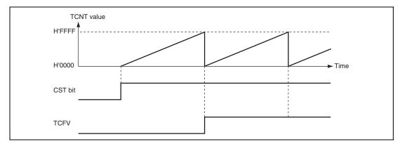
Figure 10.4 Free-Running Counter Operation
