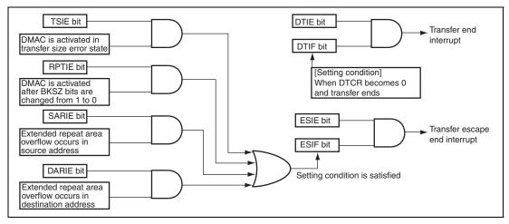
Figure 7.39 Interrupt and Interrupt Sources
