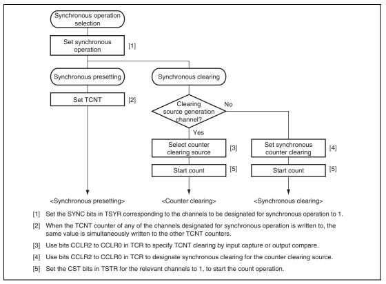
Figure 10.11 Example of Synchronous Operation Setting Procedure
