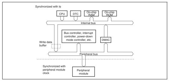
Figure 6.2 Internal Bus Configuration
