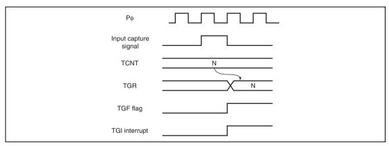
Figure 10.40 TGI Interrupt Timing (Input Capture)
