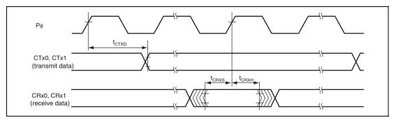
Figure 25.21 RCAN-TL1 Input/Output Timing
