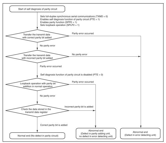
Figure 15.42 Parity Circuit Self Diagnosis Flowchart
