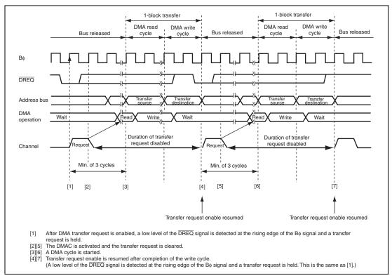
Figure 7.32 Example of Transfer in Block Transfer Mode Activated by DREO Low Level
