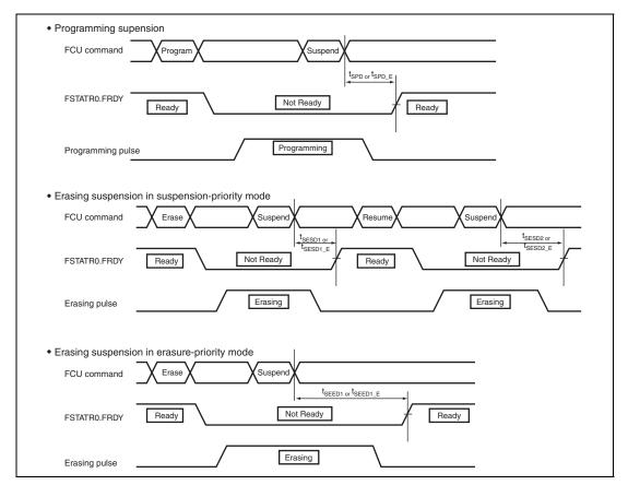
Figure 25.27 Flash Programming/Erasing Suspend Timing
