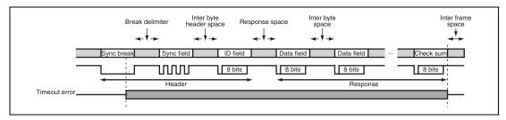
Figure 16.16 Timeout Error Detection Target in Slave Mode
