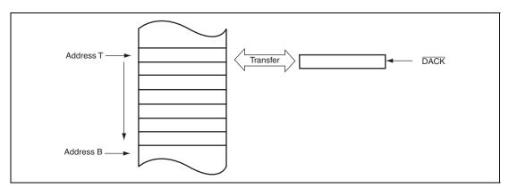
Figure 7.6 Operations in Single Address Mode
