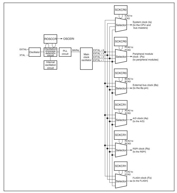
Figure 22.1 Block Diagram of Clock Pulse Generator
