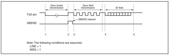
Figure 16.2 Example of Operation in the Transmission of a Header Field
