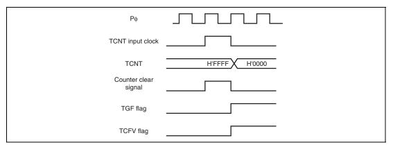
Figure 10.53 Conflict between Overflow and Counter Clearing
