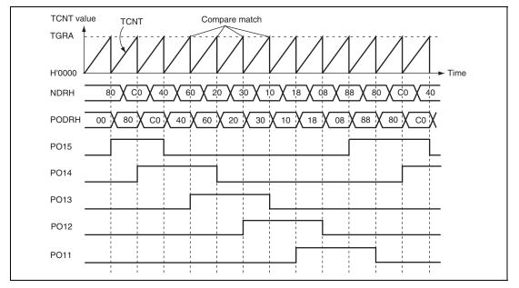
Figure 11.5 Normal Pulse Output Example (5-Phase Pulse Output)
