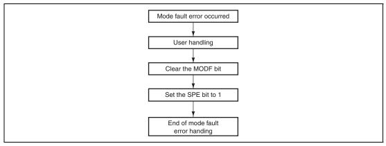
Figure 15.40 Error Handling (Mode Fault Error)
