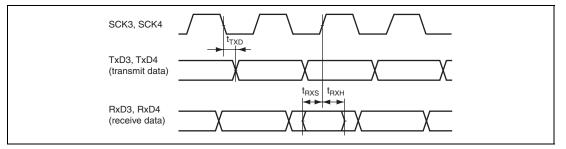
Figure 25.19 SCI Input/Output Timing: Clocked Synchronous Mode
