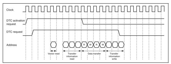
Figure 8.12 DTC Operation Timing (Example of Short Address Mode in Block Transfer Mode with Block Size of 2)
