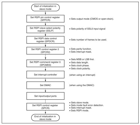
Figure 15.30 Example of Initialization Flowchart in Slave Mode
