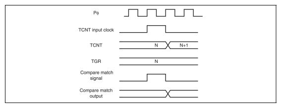
Figure 10.33 Output Compare Output Timing
