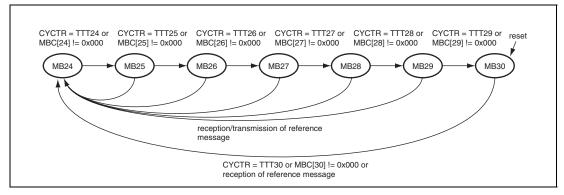
Figure 14.13 TTTSEL modification algorithm
