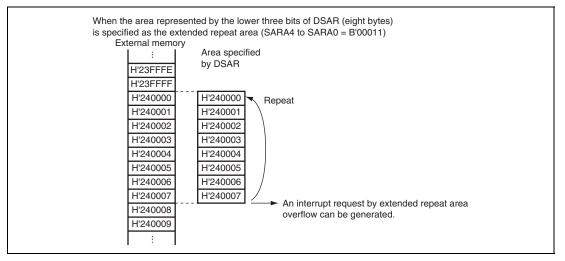
Figure 7.15 Example of Extended Repeat Area Operation
