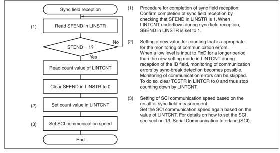
Figure 16.11 Example of Settings for Sync Field Reception in Slave Mode
