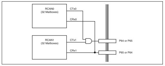
Figure 14.30 Connection Example when Using RCAN-TL1 as 1-Channel Module (64 Mailboxes × 1 Channel)
