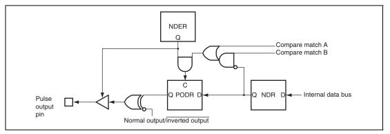
Figure 11.6 Non-Overlapping Pulse Output
