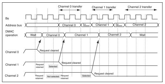
Figure 7.22 Example of Timing for Channel Priority
