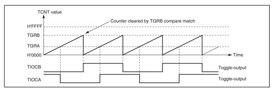
Figure 10.8 Example of Toggle Output Operation
