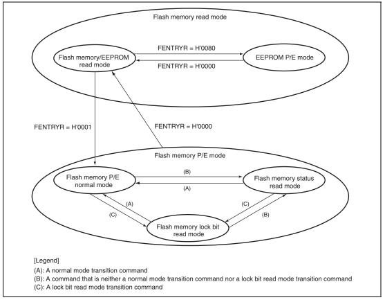
Figure 20.13 FCU Mode Transition Diagram (Flash Memory-Related Modes)
