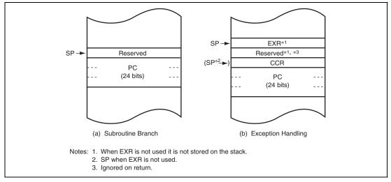
Figure 2.5 Stack Structure (Middle and Advanced Modes)
