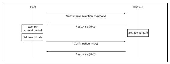
Figure 20.10 New Bit Rate Selection Sequence
