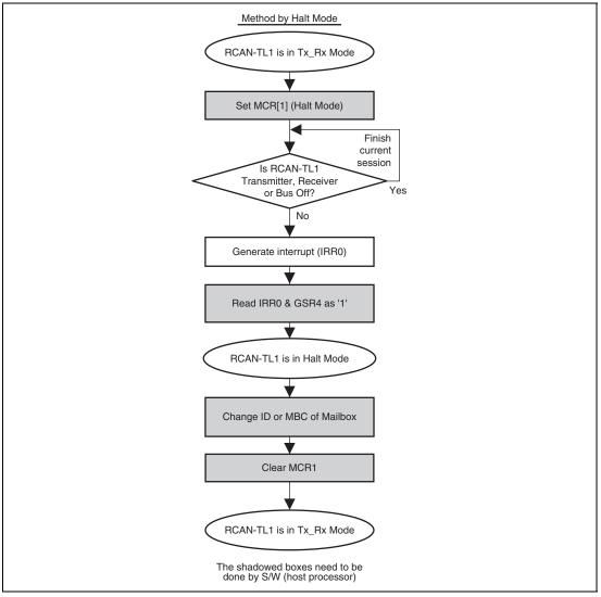
Figure 14.25 Change ID of receive box or Change receive box to transmit box
