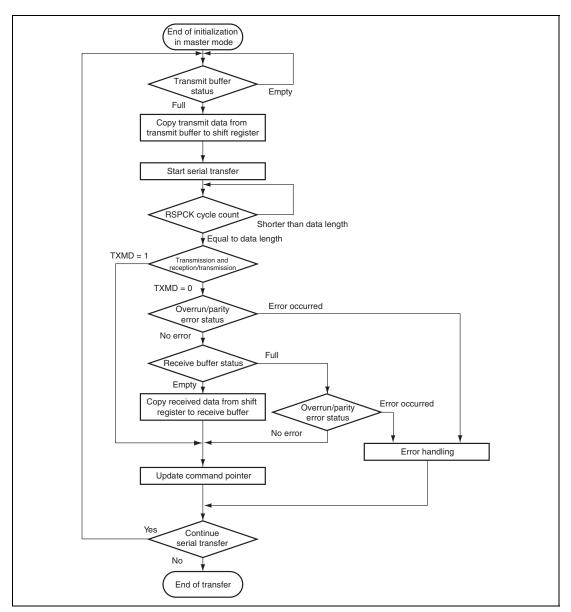
Figure 15.35 Transfer Operation Flowchart in Master Mode
