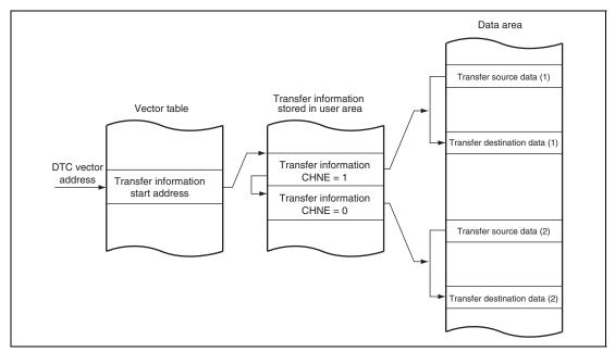
Figure 8.10 Operation of Chain Transfer
