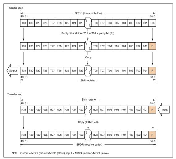
Figure 15.14 MSB First Transfer (32-Bit Data, Parity Function Enabled)
