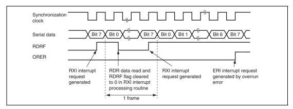
Figure 13.18 Example of Operation for Reception in Clocked Synchronous Mode
