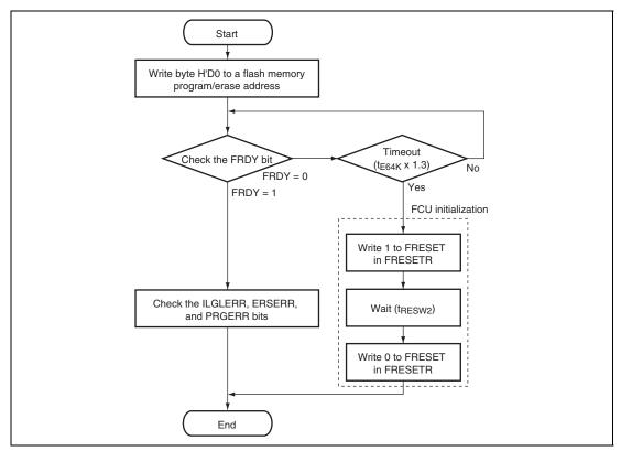
Figure 20.23 Procedure for Resuming Programming or Erasure
