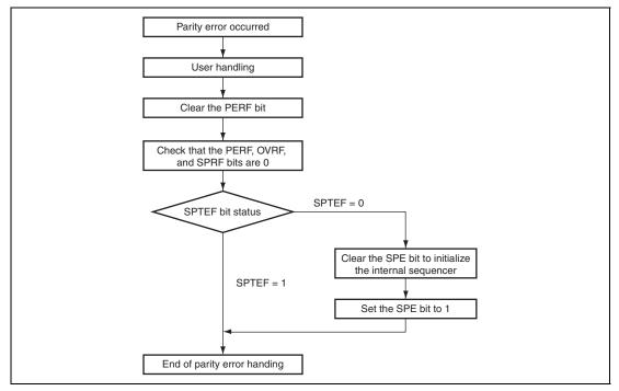
Figure 15.39 Error Handling (Parity Error)
