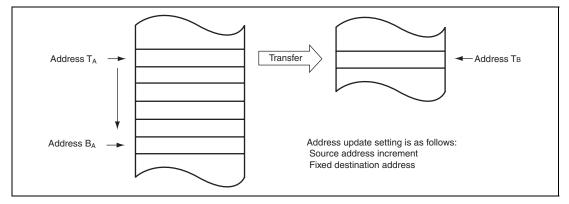
Figure 7.3 Operations in Dual Address Mode
