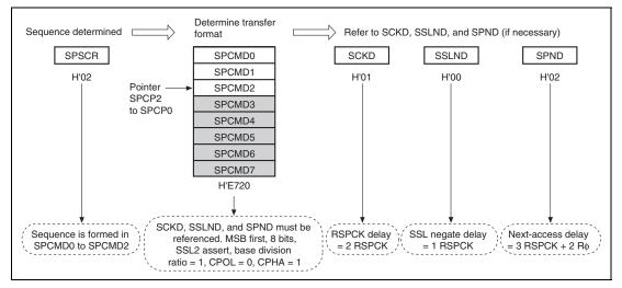
Figure 15.33 Determination Procedure of Serial Transfer Mode in Master Mode
