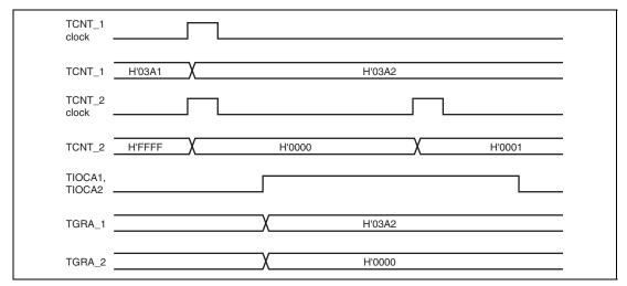
Figure 10.19 Example of Cascaded Operation (1)
