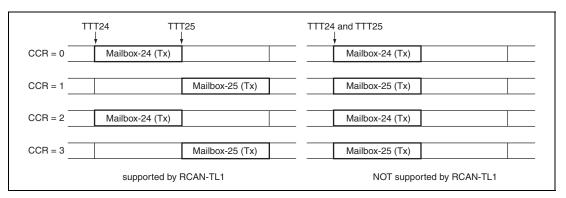
Figure 14.18 Limitation on Tx-Trigger Time
