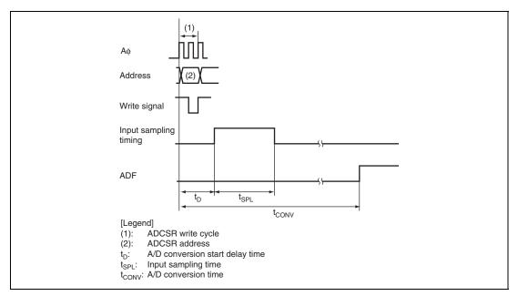
Figure 18.5 A/D Conversion Timing
