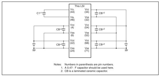
Figure 22.7 Connection Example of Bypass Capacitor
