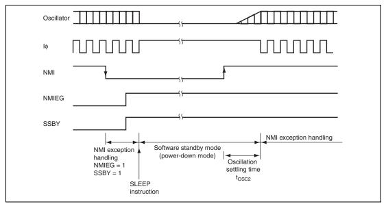
Figure 25.4 Oscillation Settling Timing after Software Standby Mode
