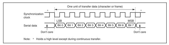
Figure 13.14 Data Format in Clocked Synchronous Communication (LSB-First)
