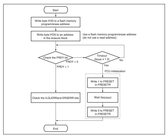
Figure 20.21 Procedure for Flash Memory Erasure
