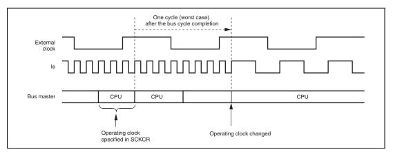
Figure 22.5 Clock Modification Timing
