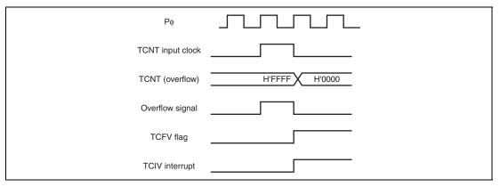
Figure 10.41 TCIV Interrupt Setting Timing
