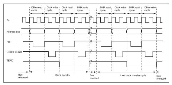
Figure 7.28 Example of Transfer in Block Transfer Mode
