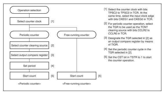
Figure 10.3 Example of Counter Operation Setting Procedure
