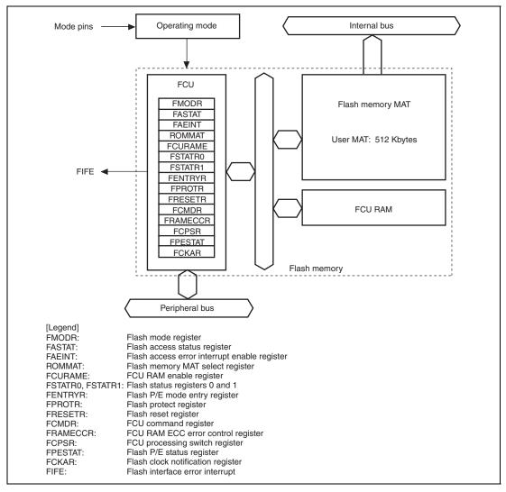
Figure 20.2 Block Diagram of Flash Memory
