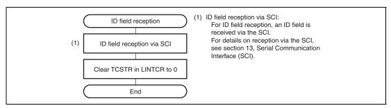
Figure 16.12 Example of Settings for ID Field Reception in Slave Mode
