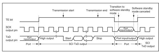
Figure 13.23 Port Pin States during Mode Transition (Internal Clock, Asynchronous Transmission)
