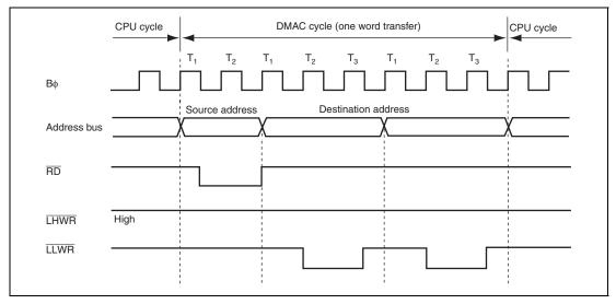
Figure 7.23 Example of Bus Timing of DMA Transfer
