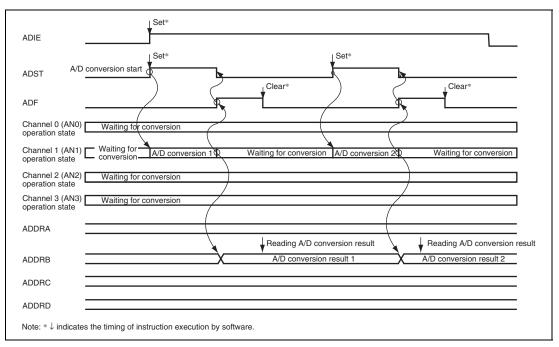
Figure 18.3 Example of A/D Converter Operation (Single Mode, Channel 1 Selected)
