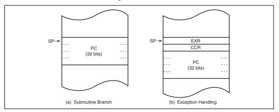
Figure 2.7 Stack Structure (Maximum Mode)
