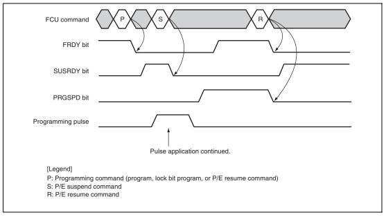
Figure 20.29 Suspending Programming Processing
