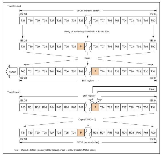
Figure 15.20 LSB First Transfer (24-Bit Data, Parity Function Enabled)
