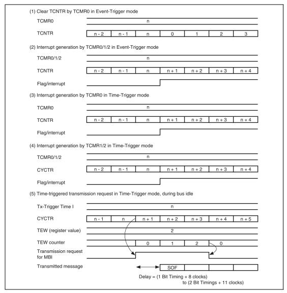
Figure 14.23 Timing Diagram of Timer
