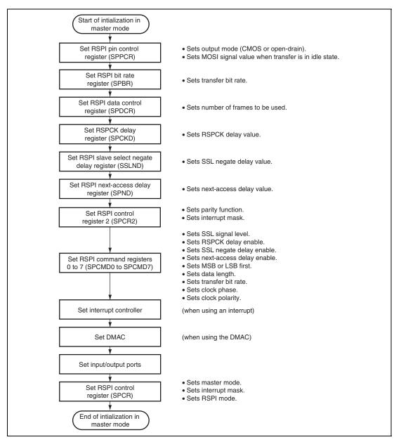
Figure 15.28 Example of Initialization Flowchart in Master Mode
