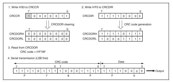
Figure 17.2 LSB-First Data Transmission
