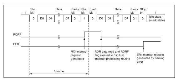
Figure 13.8 Example of SCI Operation for Reception (Example with 8-Bit Data, Parity, One Stop Bit)
