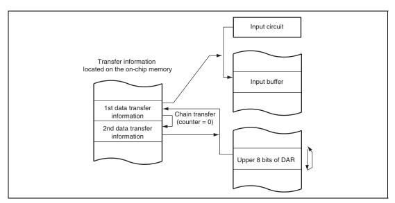
Figure 8.16 Chain Transfer when Counter = 0
