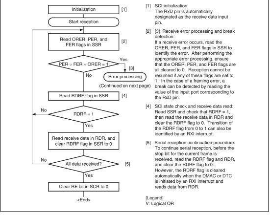
Figure 13.9 Sample Serial Reception Flowchart (1)
