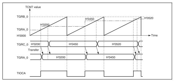
Figure 10.16 Example of Buffer Operation (1)
