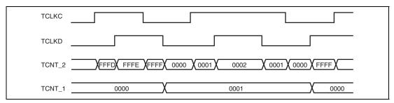
Figure 10.20 Example of Cascaded Operation (2)
