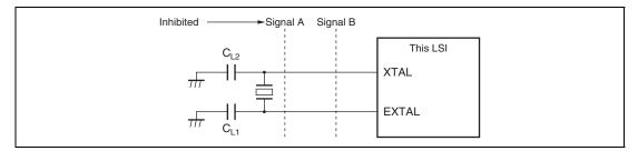
Figure 22.6 Note on Board Design for Oscillation Circuit
