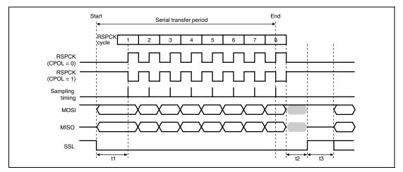
Figure 15.11 RSPI Transfer Format (CPHA = 0)
