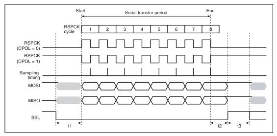
Figure 15.12 RSPI Transfer Format (CPHA = 1)
