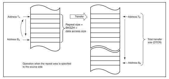
Figure 7.9 Operations in Repeat Transfer Mode
