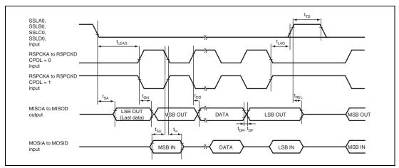
Figure 25.26 RSPI Timing (Slave, CPHA = 1)
