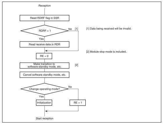
Figure 13.25 Sample Flowchart for Mode Transition during Reception
