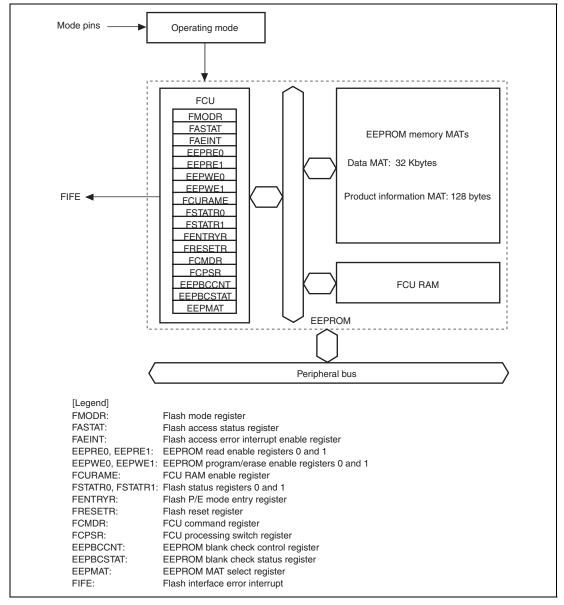
Figure 21.2 Block Diagram of EEPROM
