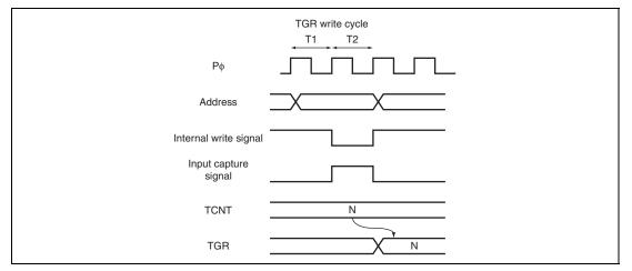
Figure 10.51 Conflict between TGR Write and Input Capture
