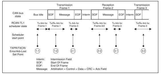
Figure 14.17 Internal Arbitration for transmission
