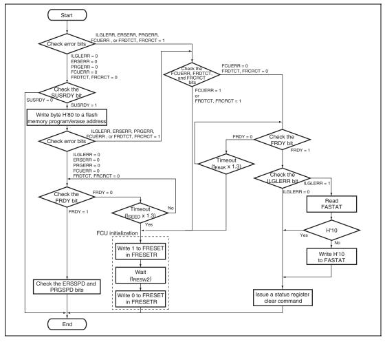
Figure 20.22 Procedure for Programming/Erasure Suspension
