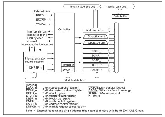
Figure 7.1 Block Diagram of DMAC
