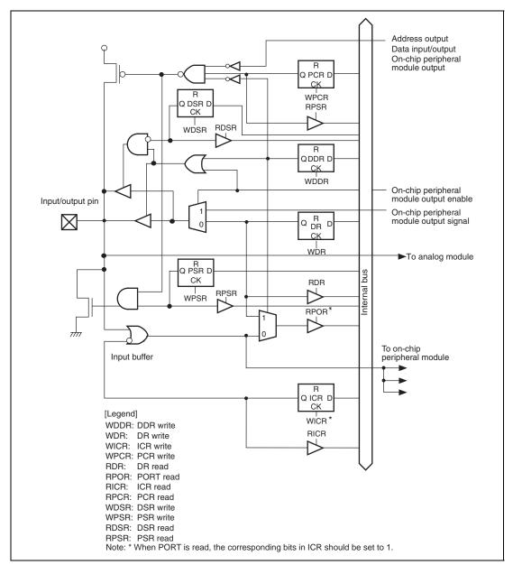
Figure 9.1 I/O Port Block Diagram
