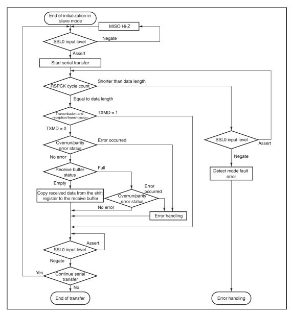
Figure 15.31 Transfer Operation Flowchart in Slave Mode (CPHA = 0)
