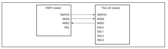
Figure 15.10 Master (Clock Synchronous Operation)/Slave (Clock Synchronous Operation)
