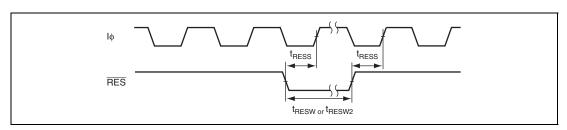
Figure 25.12 Reset Input Timing
