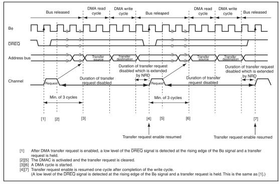
Figure 7.33 Example of Transfer in Normal Transfer Mode Activated by DREQ Low Level with NRD = 1
