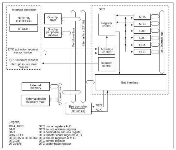
Figure 8.1 Block Diagram of DTC
