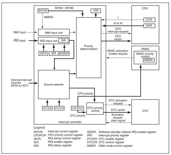
Figure 5.1 Block Diagram of Interrupt Controller
