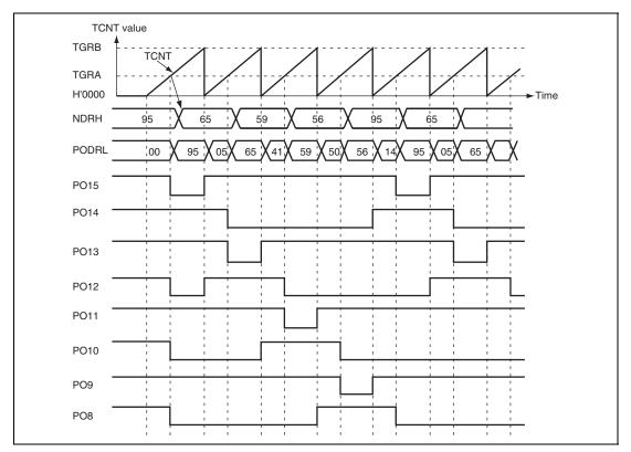
Figure 11.10 Inverted Pulse Output (Example)
