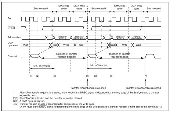
Figure 7.31 Example of Transfer in Normal Transfer Mode Activated by DREQ Low Level
