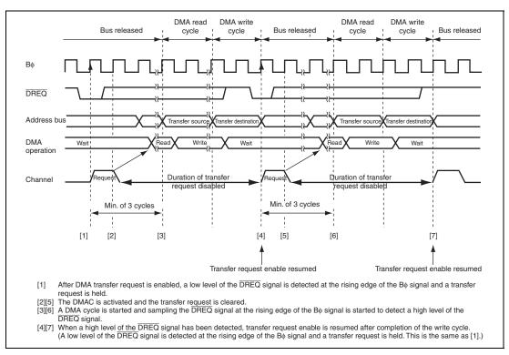
Figure 7.29 Example of Transfer in Normal Transfer Mode Activated by DREQ Falling Edge
