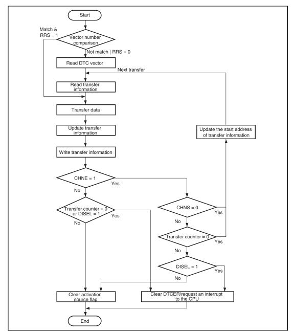
Figure 8.4 Flowchart of DTC Operation
