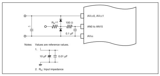
Figure 18.12 Example of Analog Input Protection Circuit
