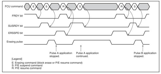
Figure 20.30 Suspending Erasure Processing (Suspension-Priority Mode)
