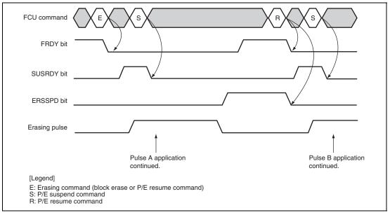
Figure 20.31 Suspending Erasure Processing (Erasure-Priority Mode)
