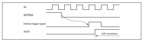
Figure 18.6 External Trigger Input Timing
