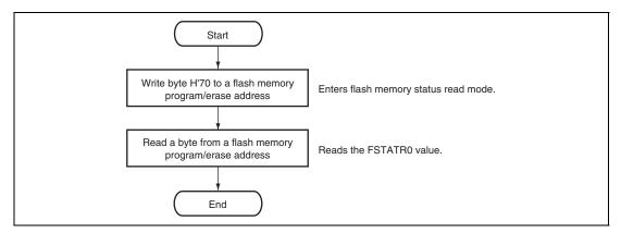
Figure 20.25 Procedure for Checking Status Register 0
