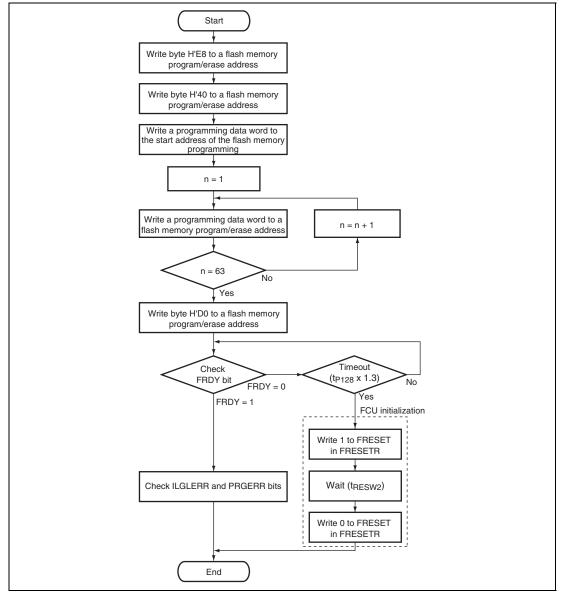
Figure 20.20 Procedure for Flash Memory Programming
