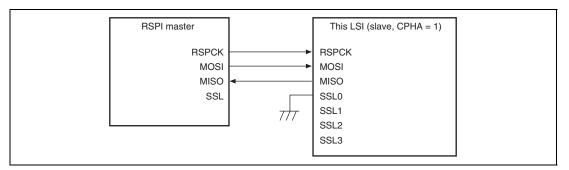
Figure 15.5 Single-Master/Single-Slave Configuration Example (This LSI = Slave, CPHA = 1)
