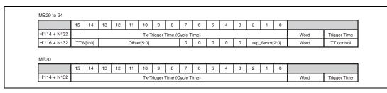
Figure 14.6 Tx-Trigger control field
