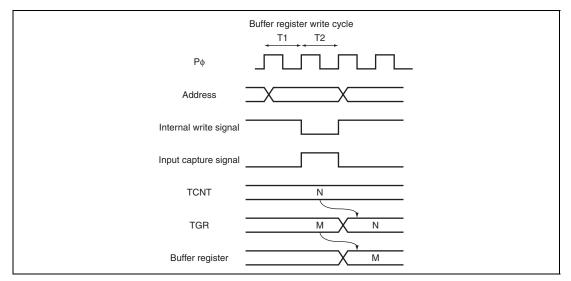
Figure 10.52 Conflict between Buffer Register Write and Input Capture
