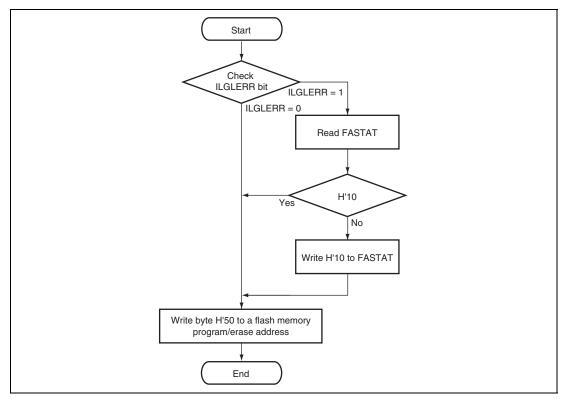
Figure 20.24 Procedure for Clearing Status Register 0
