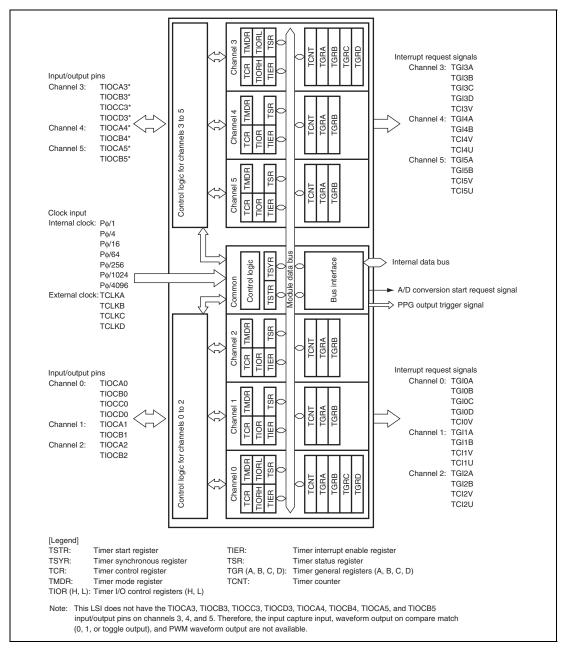
Figure 10.1 Block Diagram of TPU (Unit 0)
