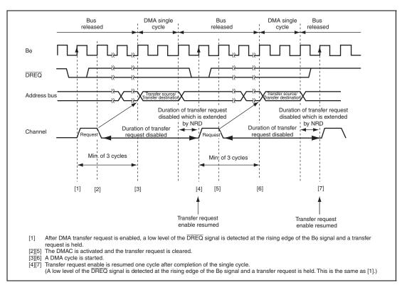
Figure 7.38 Example of Transfer in Single Address Mode Activated by  $\overline{DREQ}$  Low Level with NRD = 1
