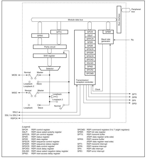
Figure 15.1 Block Diagram of RSPI (for One Channel)
