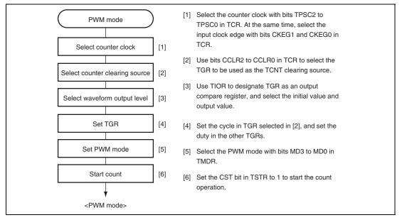
Figure 10.21 Example of PWM Mode Setting Procedure
