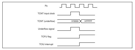
Figure 10.42 TCIU Interrupt Setting Timing
