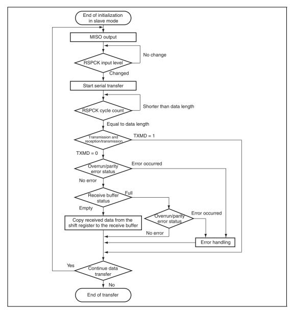
Figure 15.37 Transfer Operation Flowchart in Slave Mode (CPHA = 1)
