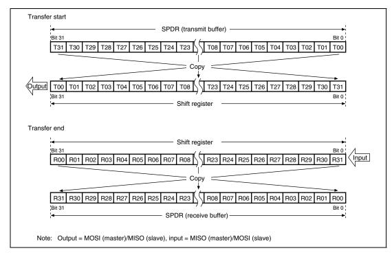
Figure 15.17 LSB First Transfer (32-Bit Data, Parity Function Disabled)
