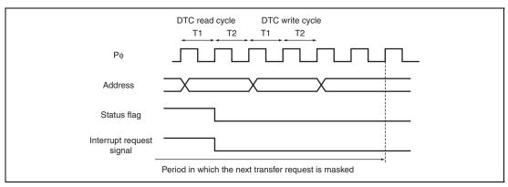
Figure 10.44 Timing for Status Flag Clearing by DTC Activation
