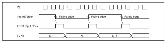
Figure 10.31 Count Timing in Internal Clock Operation
