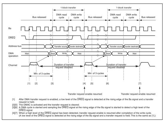
Figure 7.30 Example of Transfer in Block Transfer Mode Activated by DREQ Falling Edge
