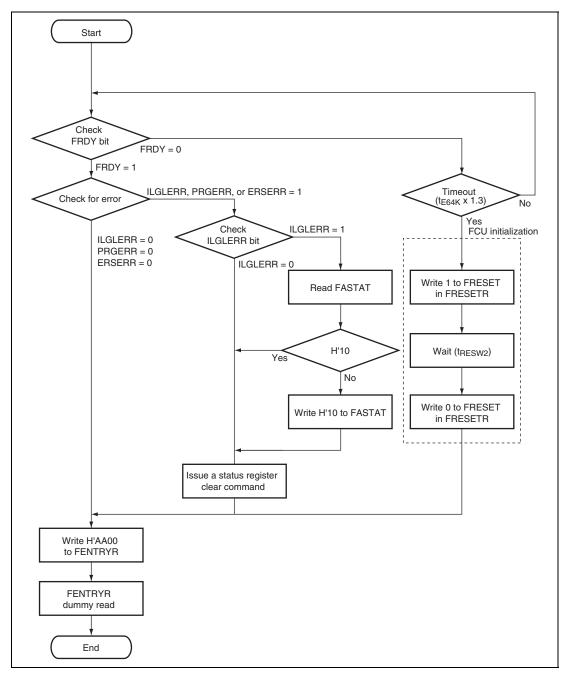
Figure 20.17 Procedure for Transition to Flash Memory Read Mode
