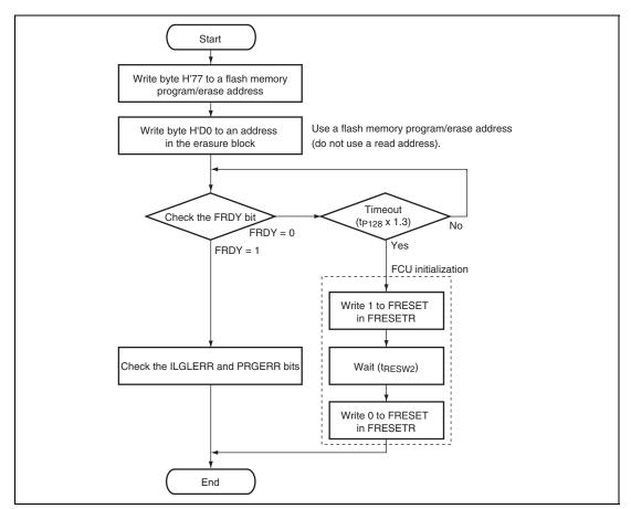
Figure 20.28 Procedure for Writing to the Lock Bit
