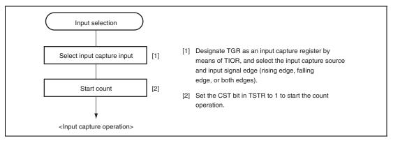
Figure 10.9 Example of Setting Procedure for Input Capture Operation
