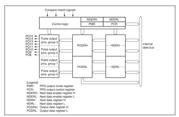
Figure 11.1 Block Diagram of PPG
