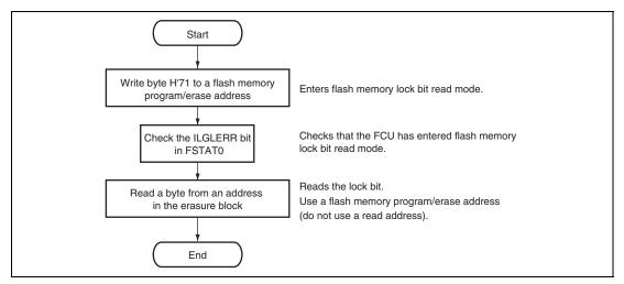
Figure 20.26 Procedure for Reading Lock Bit in Memory Area Read Mode
