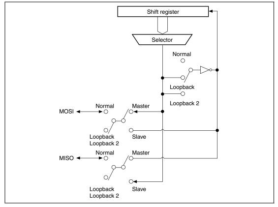
Figure 15.41 Configuration of Shift Register Input/Output Paths in Loopback Mode (Master Mode)
