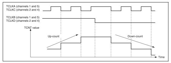
Figure 10.27 Example of Phase Counting Mode 2 Operation
