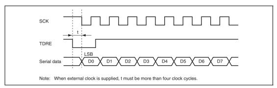
Figure 13.21 Sample Transmission using DMAC or DTC in Clocked Synchronous Mode
