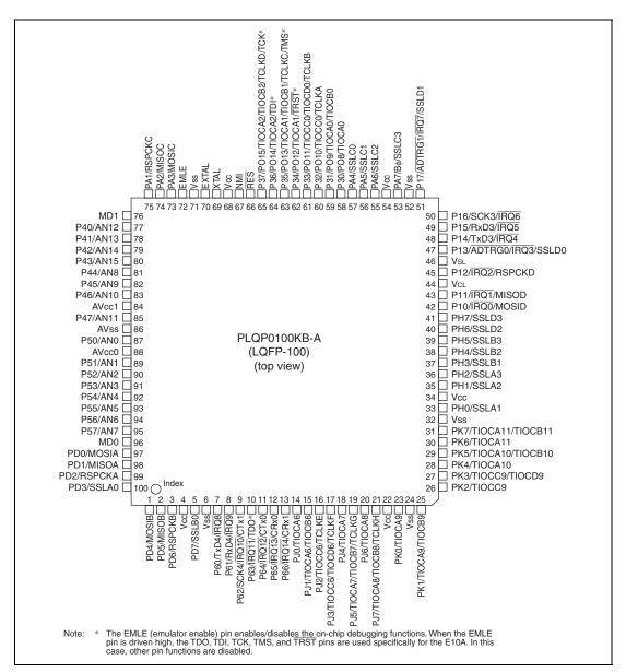
Figure 1.2 Pin Assignments of H8SX/1725S and H8SX/1727S
