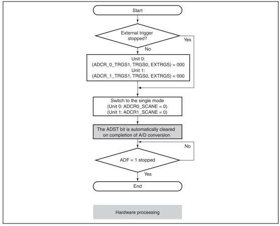
Figure 18.15 When Continuous Scan Mode is Stopped by an External Trigger
