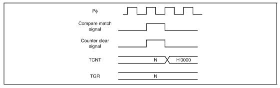
Figure 10.35 Counter Clear Timing (Compare Match)
