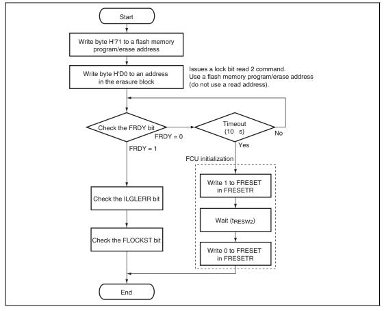
Figure 20.27 Procedure for Reading Lock Bit in Register Read Mode
