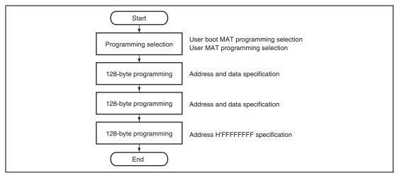
Figure 20.11 Procedure for Flash Memory Programming in Boot Mode
