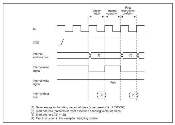
Figure 4.1 Reset Sequence (On-chip ROM Enabled Advanced Mode)
