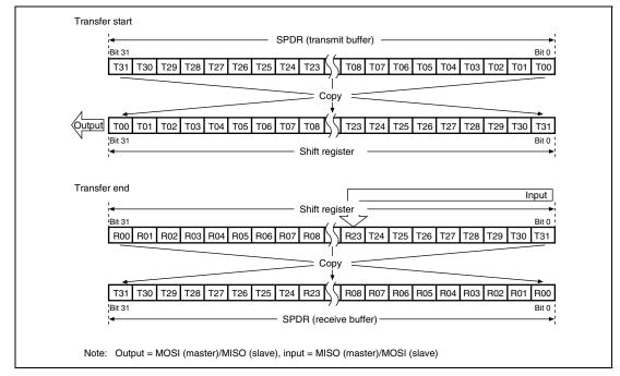
Figure 15.19 LSB First Transfer (24-Bit Data, Parity Function Disabled)
