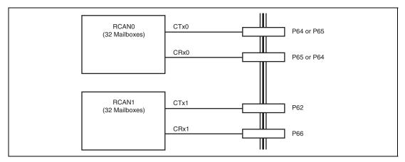
Figure 14.29 Connection Example when Using RCAN-TL1 as 2-Channel Module  $(32 \text{ Mailboxes} \times 2 \text{ Channels})$
