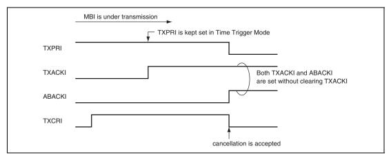
Figure 14.7 TXACK and ABACK in Time Trigger Transmission
