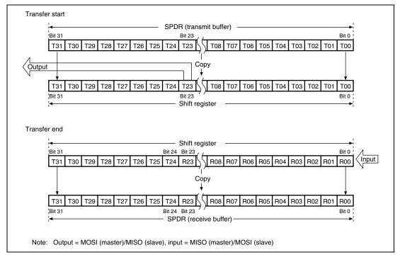
Figure 15.15 MSB First Transfer (24-Bit Data, Parity Function Disabled)
