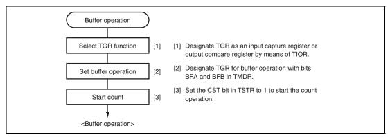
Figure 10.15 Example of Buffer Operation Setting Procedure
