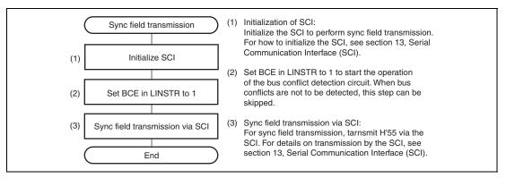
Figure 16.5 Example of Settings for Sync Field Transmission in Master Mode
