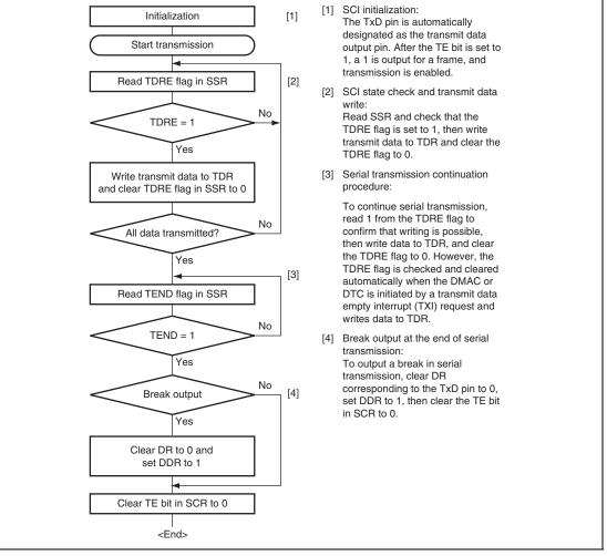
Figure 13.7 Sample Serial Transmission Flowchart
