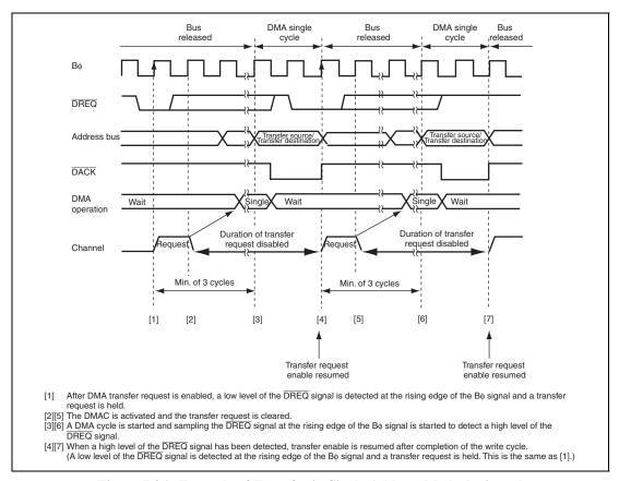
Figure 7.36 Example of Transfer in Single Address Mode Activated by DREQ Falling Edge
