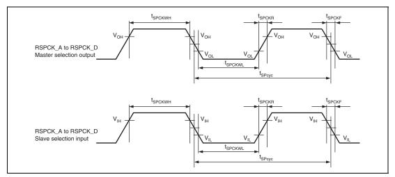
Figure 25.22 RSPI Clock Timing
