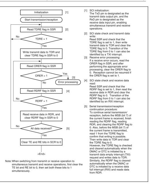
Figure 13.20 Sample Flowchart of Simultaneous Serial Transmission and Reception
