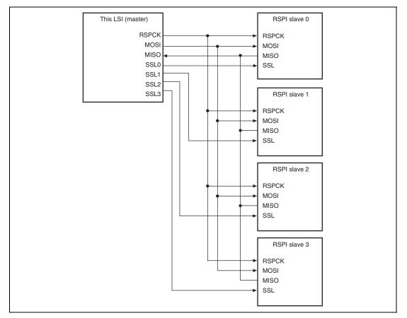
Figure 15.6 Single-Master/Multi-Slave Configuration Example (This LSI = Master)
