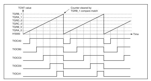
Figure 10.23 Example of PWM Mode Operation (2)
