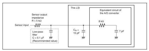
Figure 18.11 Example of Analog Input Circuit
