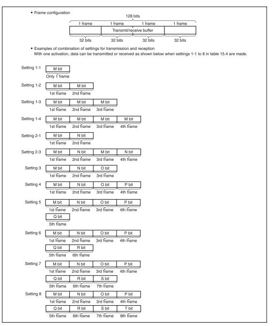
Figure 15.2 Frame Configurations and Examples of Combinations of Transmission and Reception Settings
