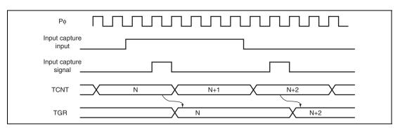
Figure 10.34 Input Capture Input Signal Timing
