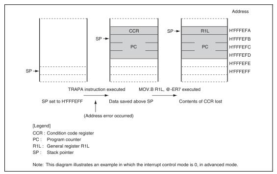
Figure 4.3 Operation when SP Value is Odd
