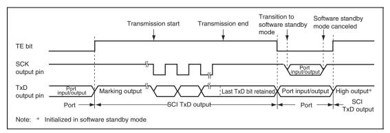
Figure 13.24 Port Pin States during Mode Transition (Internal Clock, Clocked Synchronous Transmission)
