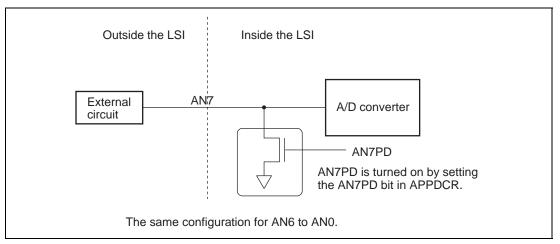
Figure 18.9 Overview of Analog Port Pull-Down Function
