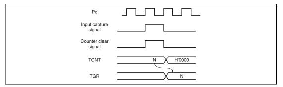
Figure 10.36 Counter Clear Timing (Input Capture)
