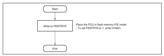
Figure 20.16 Procedure for Transition to Flash Memory P/E Mode
