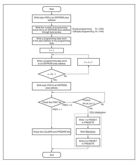
Figure 21.6 Procedure for EEPROM Programming
