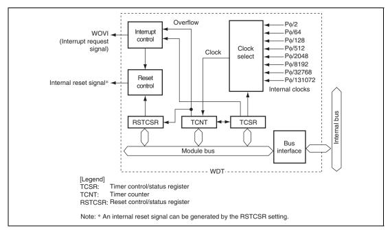
Figure 12.1 Block Diagram of WDT
