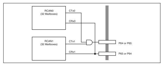
Figure 14.31 Connection Example when Using RCAN-TL1 as 1-Channel Module (64 Mailboxes × 1 Channel)
