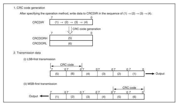
Figure 17.6 LSB-First and MSB-First Transmit Data
