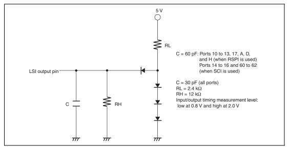
Figure 25.2 Output Load Circuit
