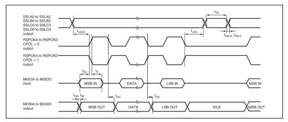
Figure 25.23 RSPI Timing (Master, CPHA = 0)
