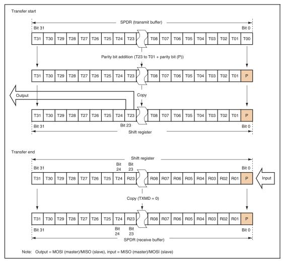
Figure 15.16 MSB First Transfer (24-Bit Data, Parity Function Enabled)
