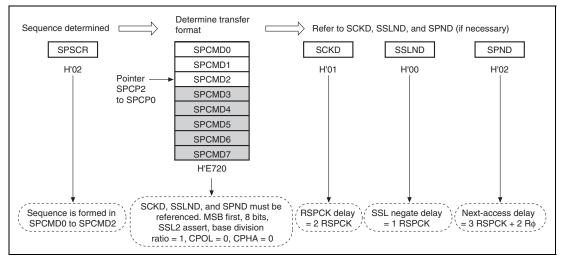
Figure 15.26 Determination Procedure of Serial Transfer Mode in Master Mode
