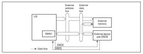
Figure 7.4 Data Flow in Single Address Mode
