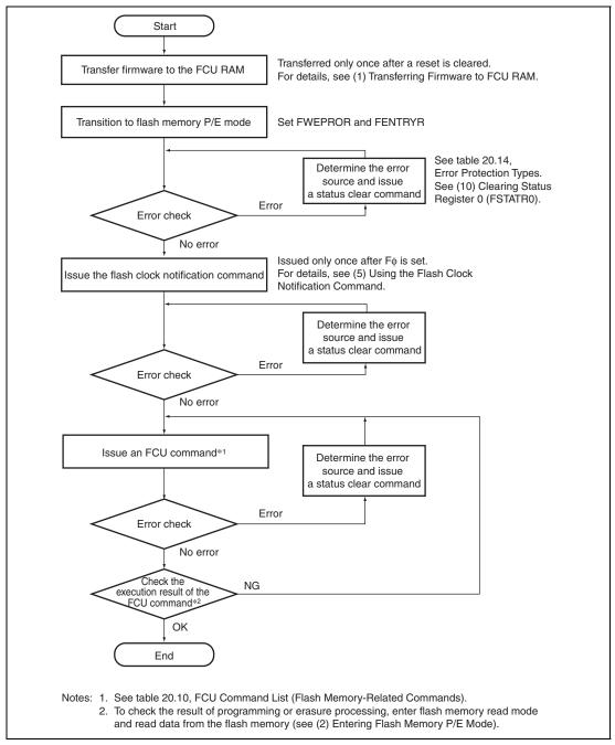
Figure 20.14 General Procedure of FCU Command Processing
