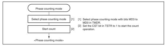
Figure 10.25 Example of Phase Counting Mode Setting Procedure
