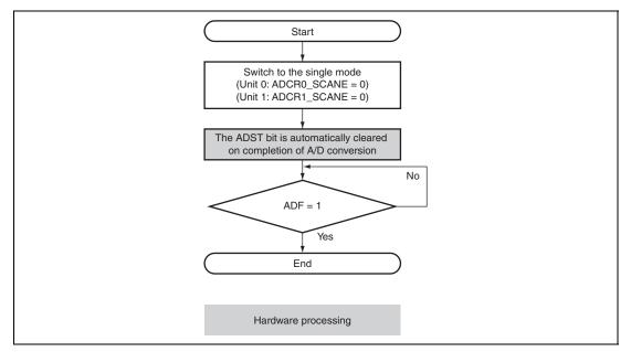
Figure 18.14 When Continuous Scan Mode is Stopped by Software
