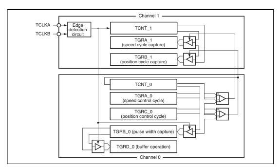
Figure 10.30 Phase Counting Mode Application Example
