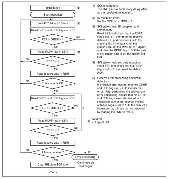
Figure 13.13 Sample Multiprocessor Serial Reception Flowchart (1)
