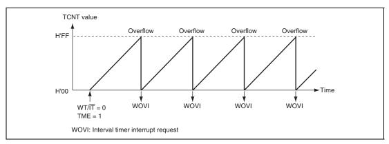
Figure 12.3 Operation in Interval Timer Mode
