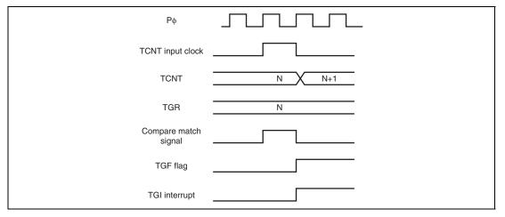
Figure 10.39 TGI Interrupt Timing (Compare Match)
