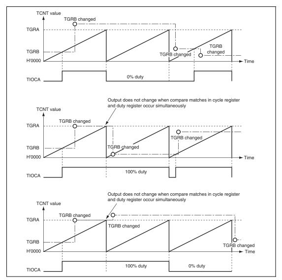
Figure 10.24 Example of PWM Mode Operation (3)
