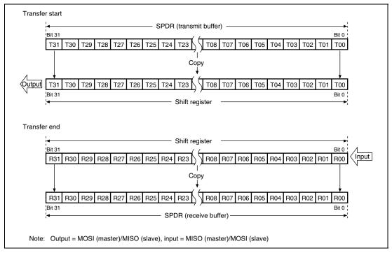
Figure 15.13 MSB First Transfer (32-Bit Data, Parity Function Disabled)
