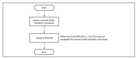
Figure 20.18 Procedure to Use Flash Memory P/E Normal Mode Transition Command
