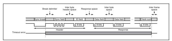
Figure 16.15 Timeout Error Detection Target in Master Mode
