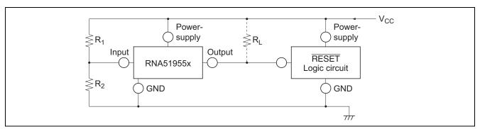
Figure 1 Reset Circuit of RNA51955
