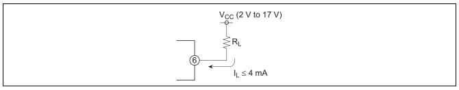
Figure 6 Output Load Resistance R<sub>L</sub>
