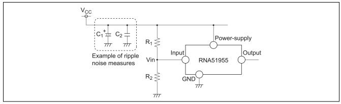
Figure 2 Example of Ripple Noise Measures
