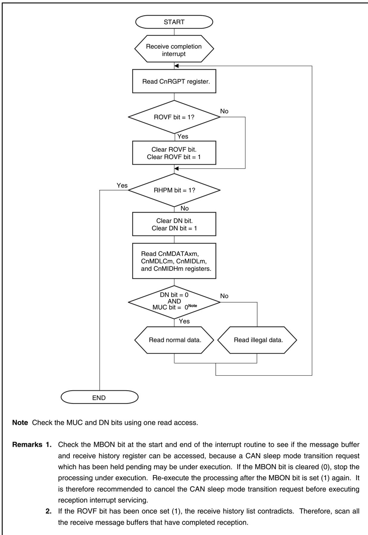
**Note** Check the MUC and DN bits using one read access.
