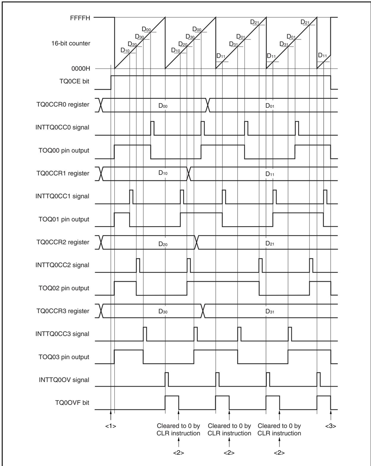
Figure 8-36. Software Processing Flow in Free-Running Timer Mode (Compare Function) (2/2)
