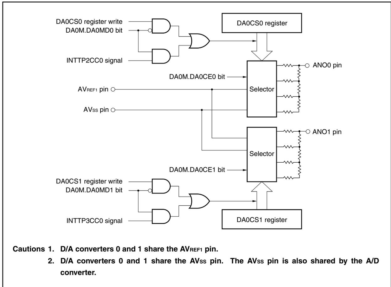
The D/A converter includes the following hardware.
