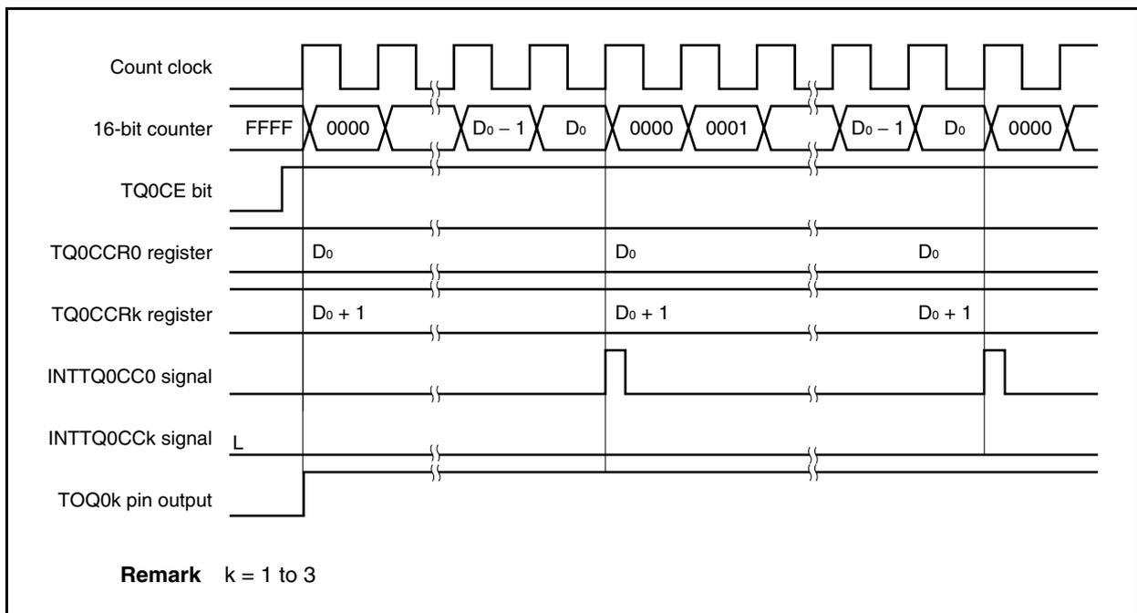
**(c) Generation timing of compare match interrupt request signal (INTTQ0CCk)**
