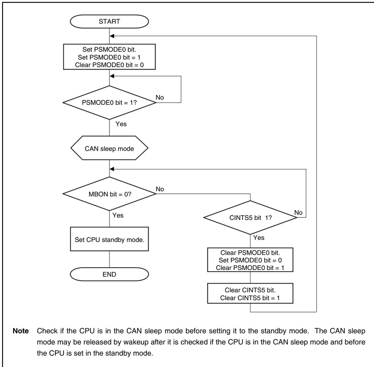
Figure 19-60. Setting CPU Standby (from CAN Stop Mode)
