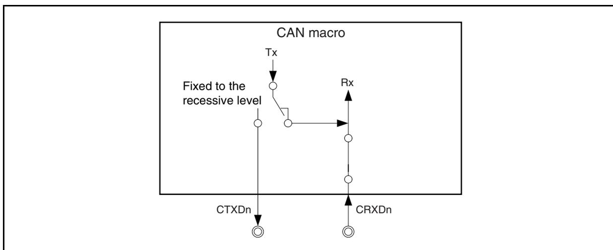
In the receive-only mode, no message frames can be transmitted from the CAN module to the CAN bus. Transmit requests issued for message buffers defined as transmit message buffers are held pending.
