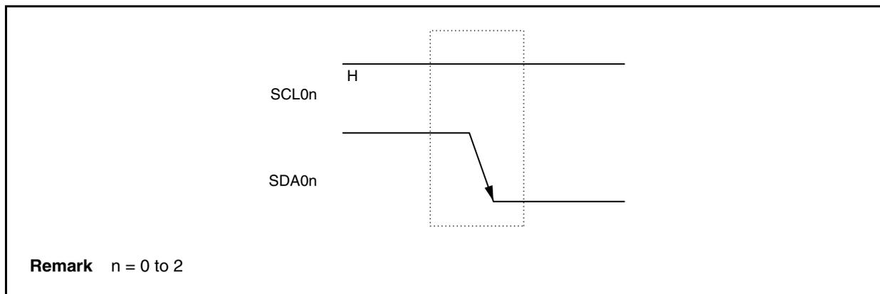
A start condition is generated when the IICn.STTn bit is set (1) after a stop condition has been detected (IICn.SPn bit = 1). When a start condition is detected, the IICn.STDn bit is set (1) (n = 0 to 2).
