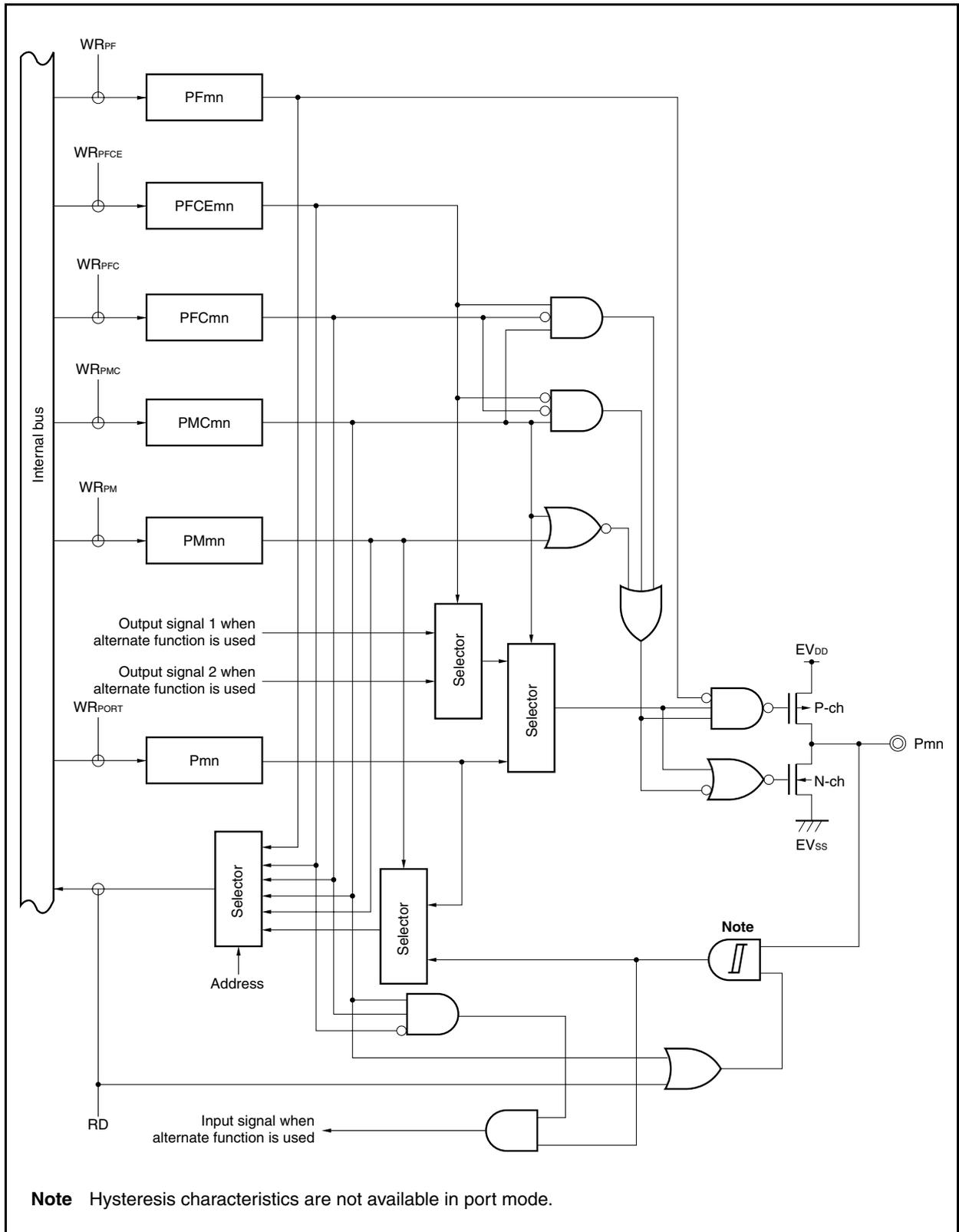
Figure 4-37. Block Diagram of Type U-13
