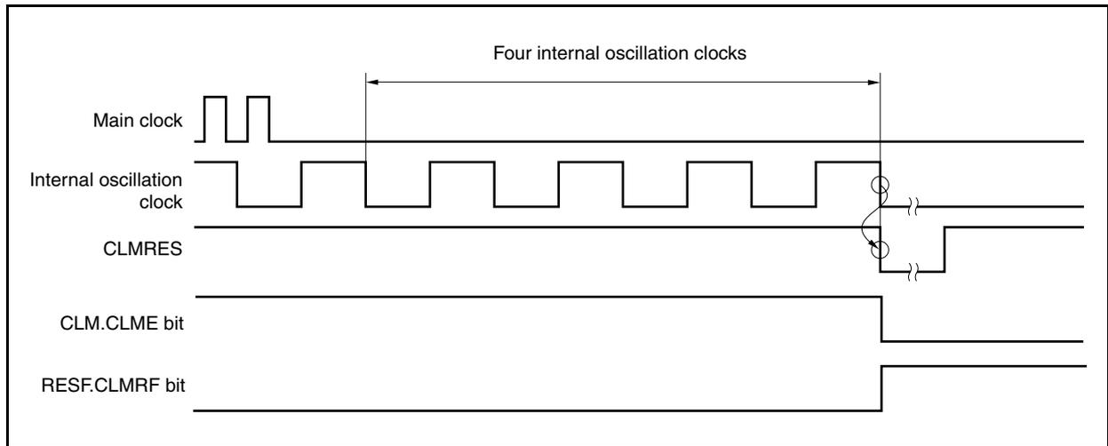
**(2) Clock monitor status after  $\overline{\text{RESET}}$  input**
