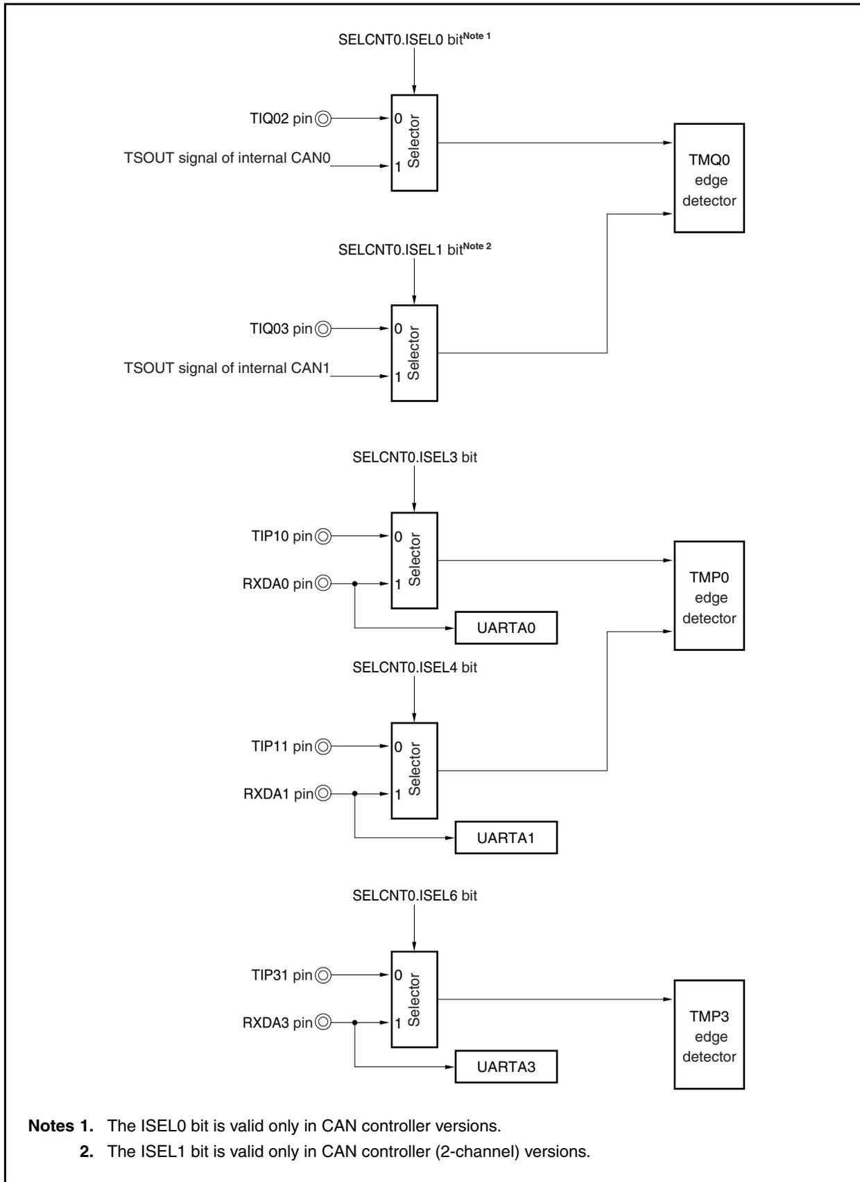
The capture trigger input for the selector function is specified by the following register.
