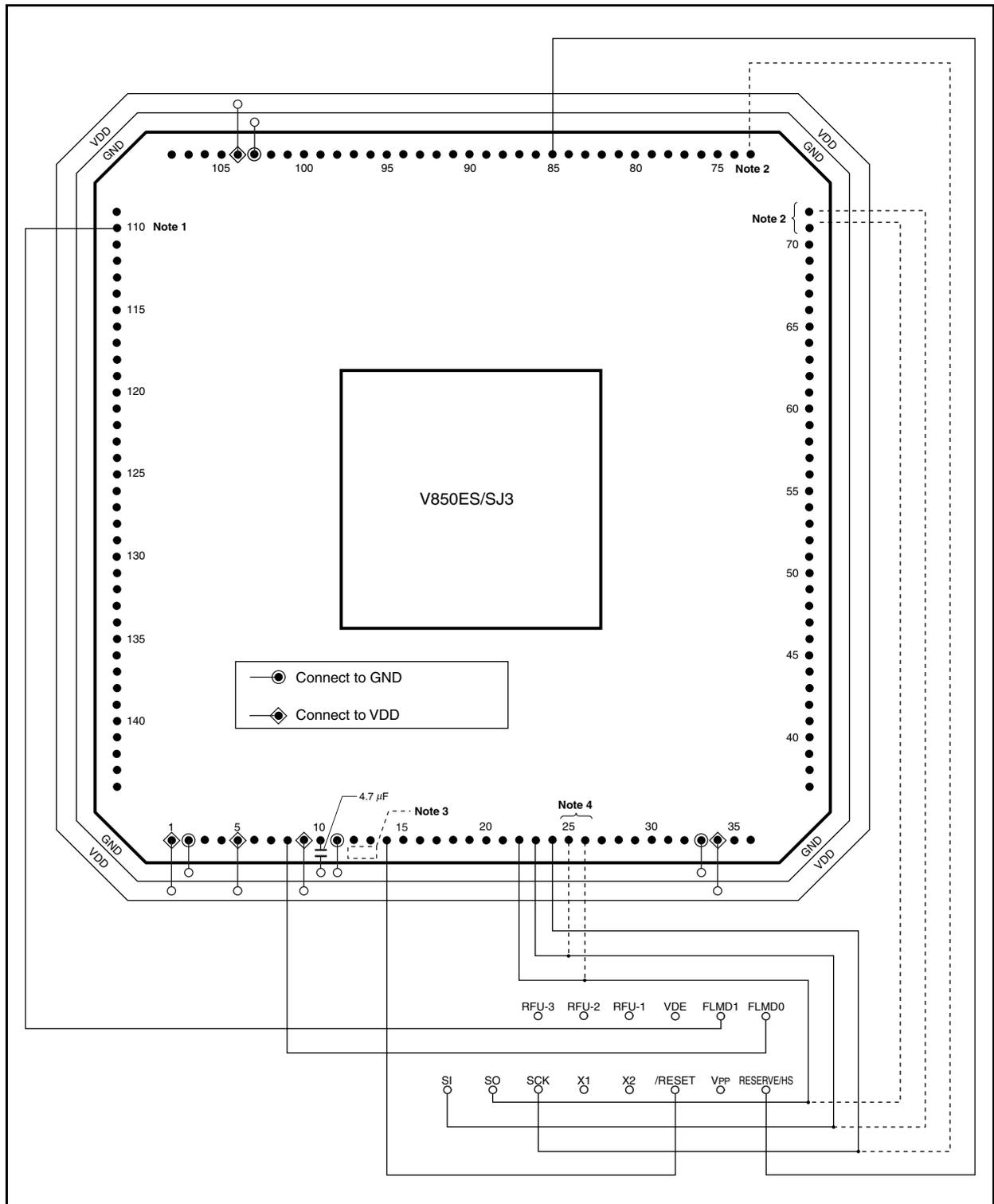
**Figure 30-6. Example of Wiring of V850ES/SJ3 Flash Writing Adapter (FA-144GJ-UEN-A)
