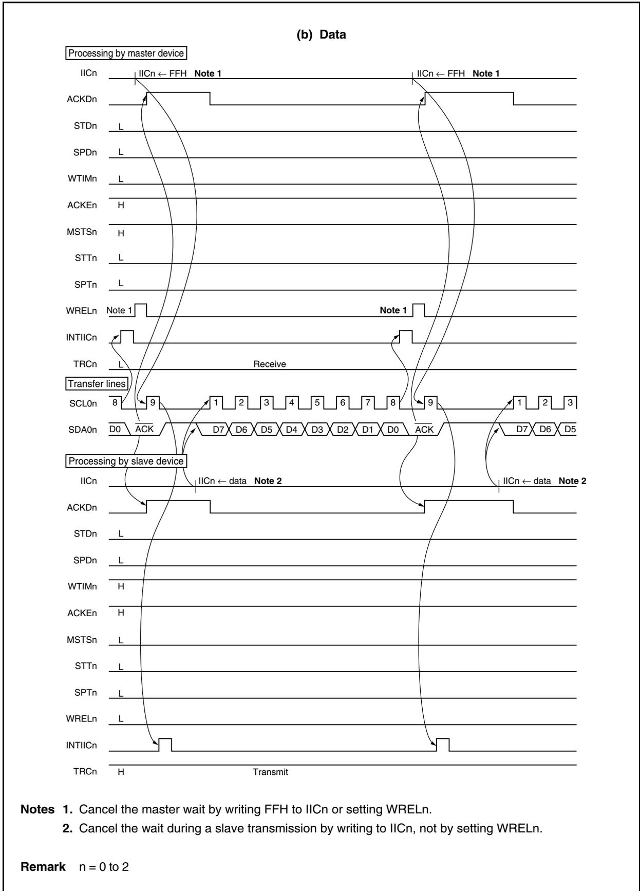
**Figure 17-21. Example of Slave to Master Communication**
