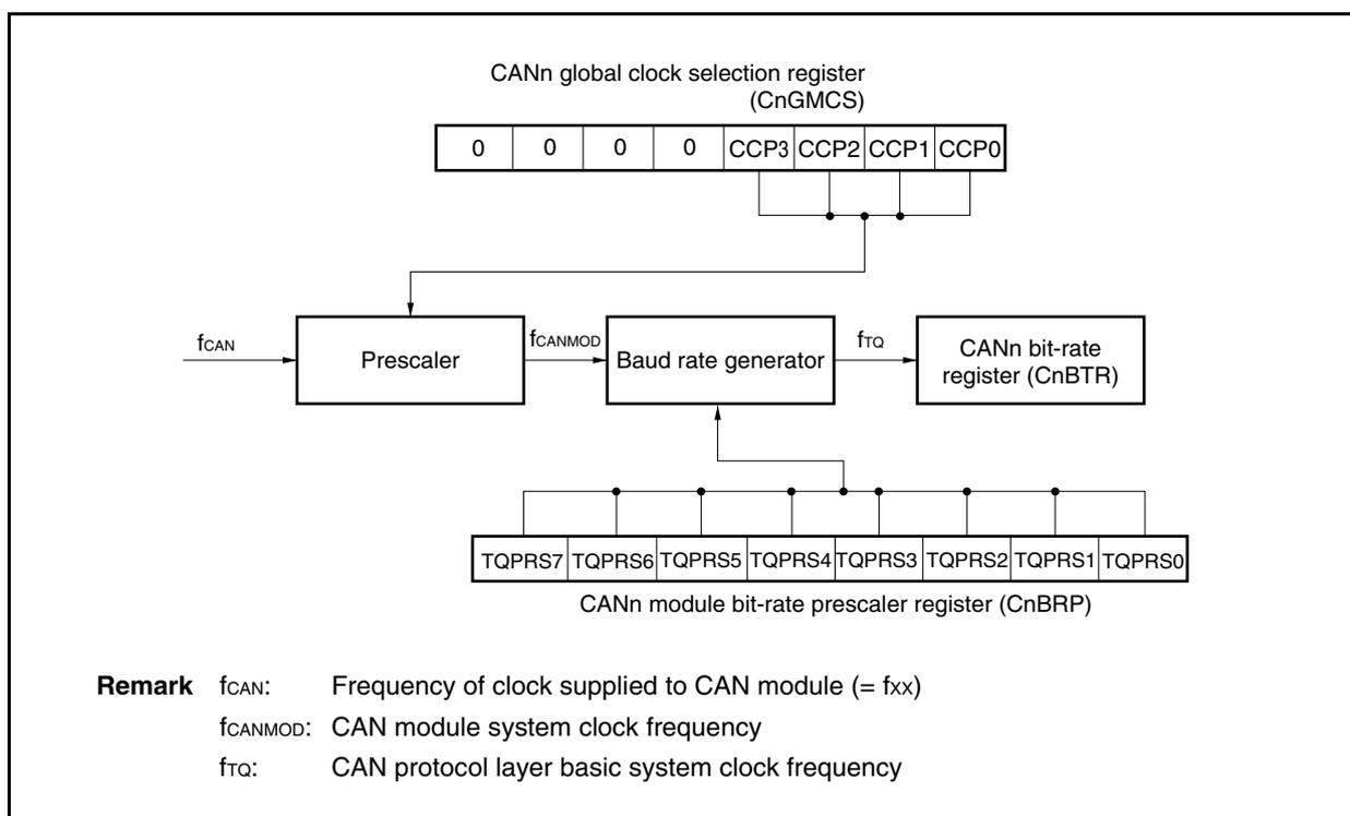
**(13) CANn module bit rate register (CnBTR)**
