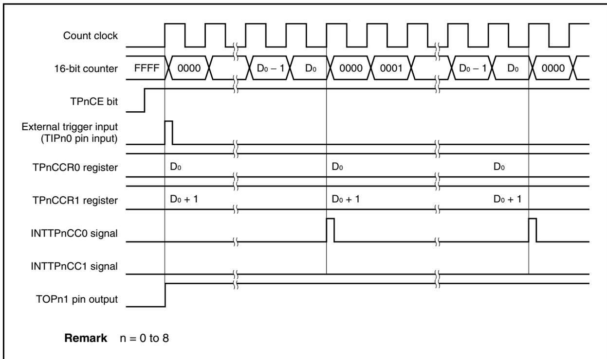
**(c) Conflict between trigger detection and match with CCR1 buffer register**
