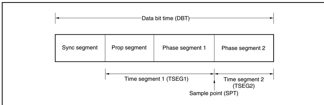
After reset: 370FH R/W Address: C0BTR 03FEC05CH, C1BTR 03FEC65CH
