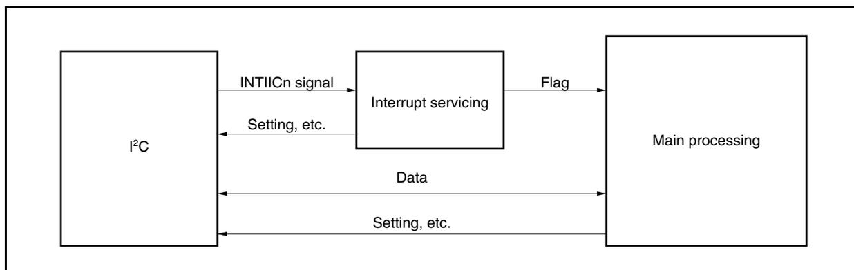
Therefore, the following three flags are prepared by software so that the data transfer processing can be performed by transmitting these flags to the main processing instead of INTIICn signal.
