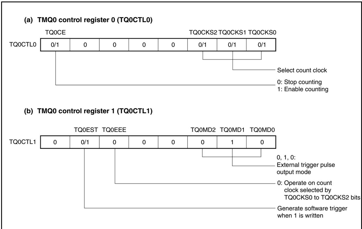
Figure 8-22. Setting of Registers in External Trigger Pulse Output Mode (2/3)
