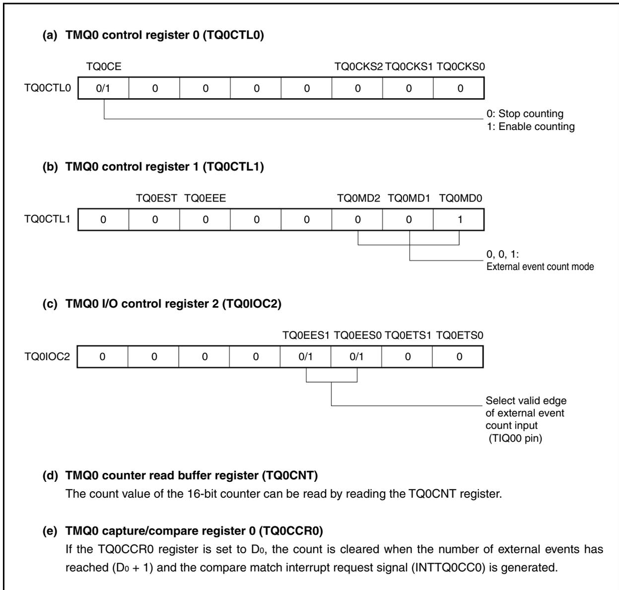
**Figure 8-15. Register Setting for Operation in External Event Count Mode (2/2)****(f) TMQ0 capture/compare registers 1 to 3 (TQ0CCR1 to TQ0CCR3)**
