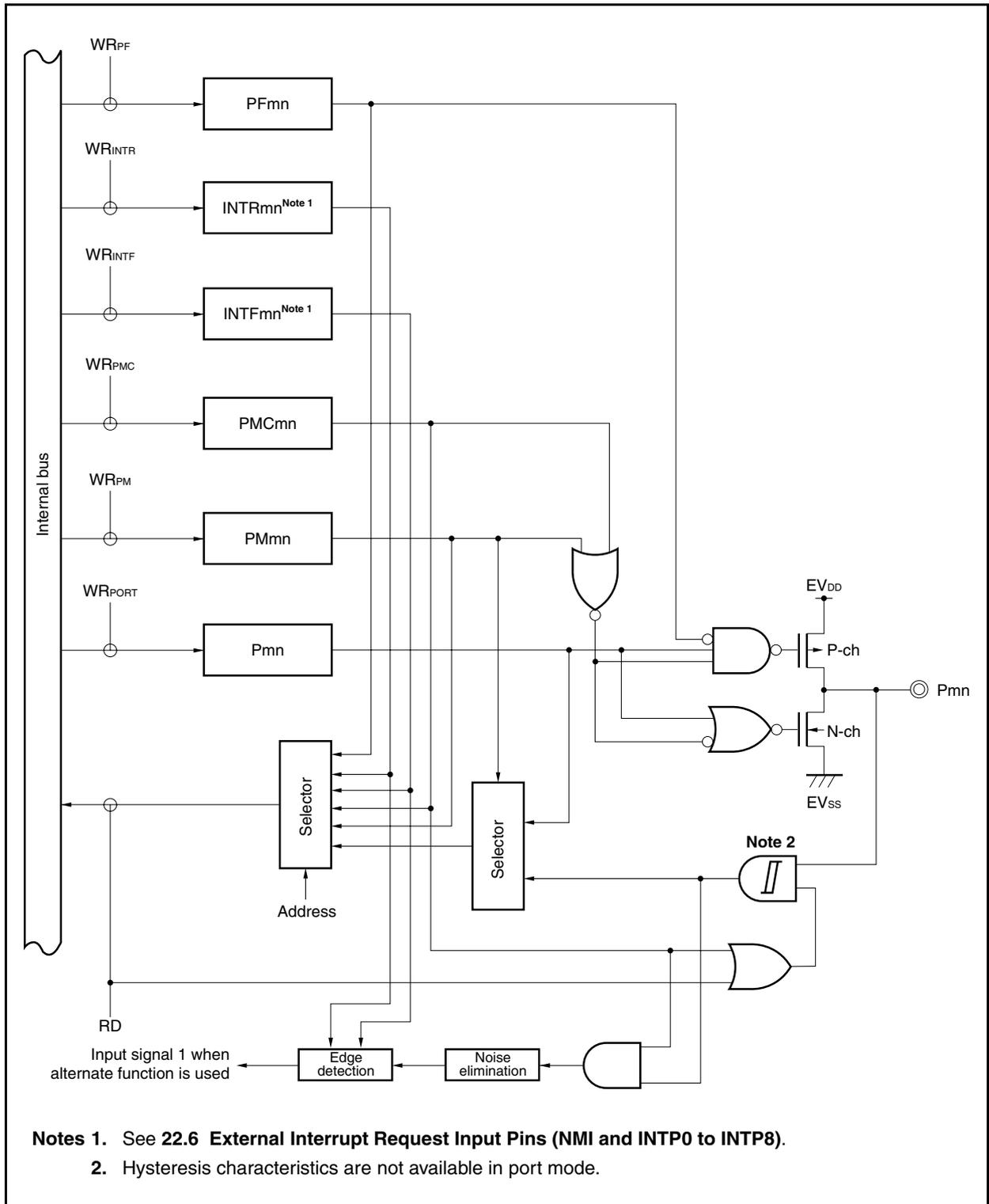
Figure 4-22. Block Diagram of Type N-1
