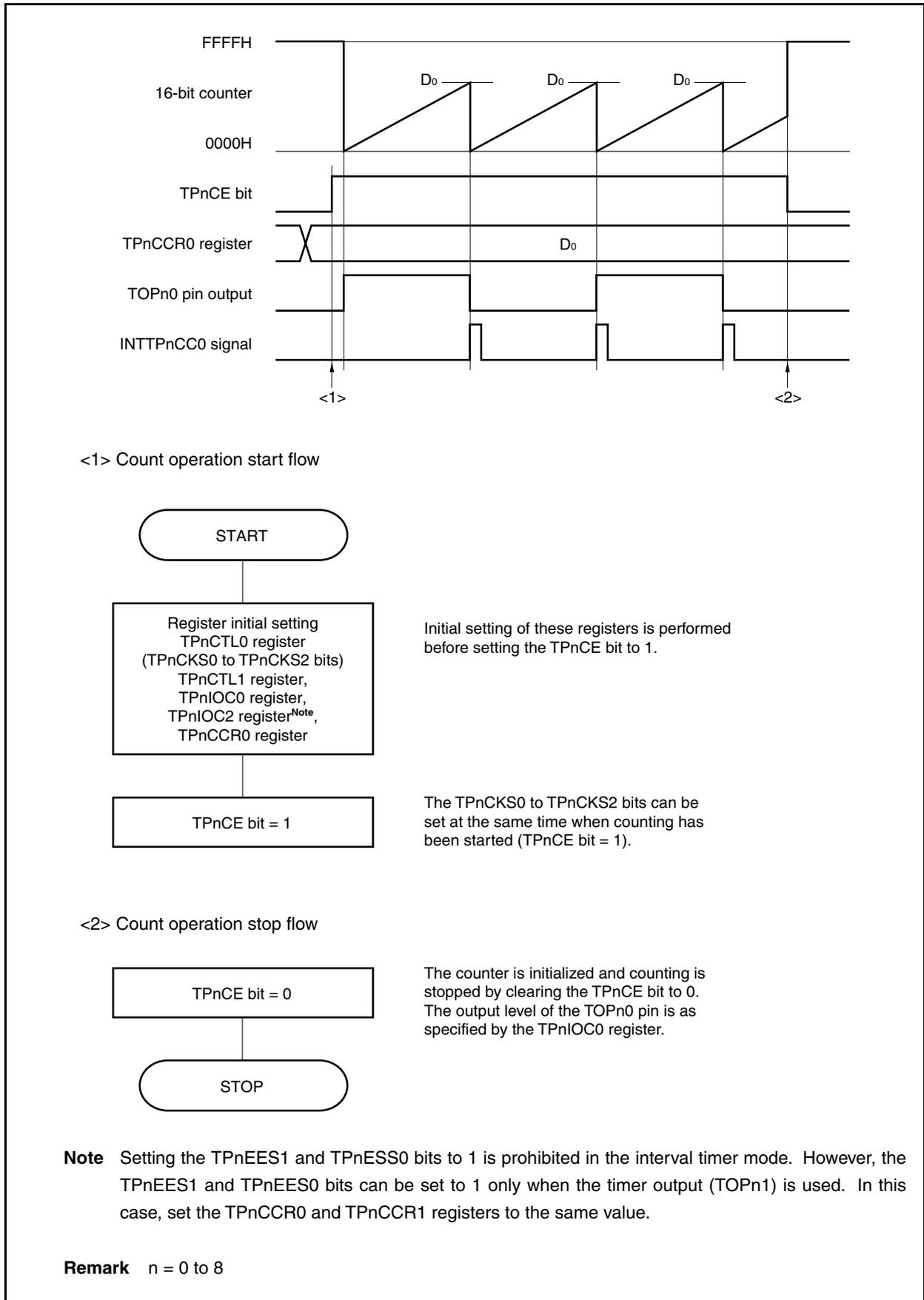
**(2) Interval timer mode operation timing****(a) Operation if TPnCCR0 register is set to 0000H**
