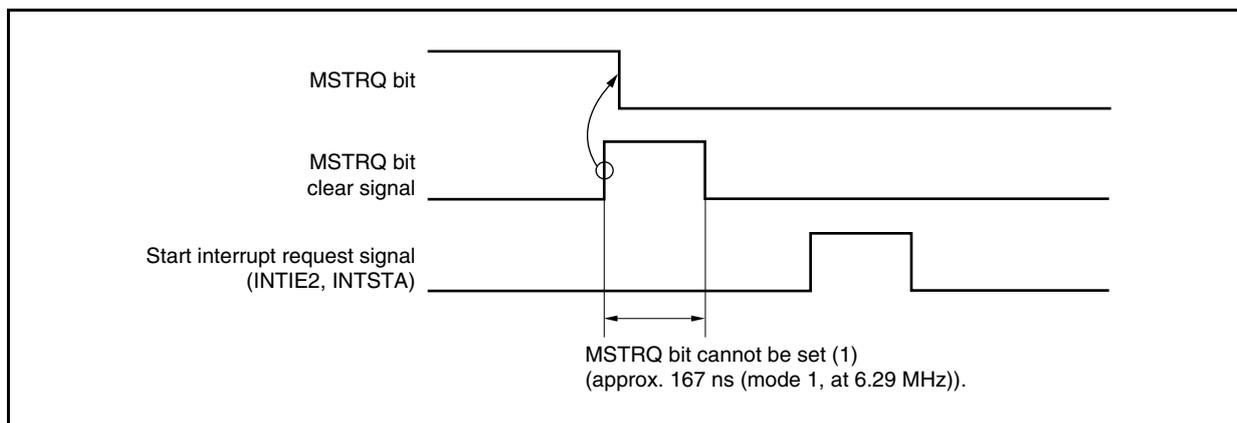
2. When a master request has been sent and bus mastership acquired, do not set the MSTRQ, ENSLVTX, or ENSLVRX bit until the end of communication (i.e. the communication end flag (ISR.ENDTRNS bit) or frame end flag (ISR.ENDFRAM bit) is set (1)) as setting these flags disables interrupt request signal generation. However, these flags can be set if communication has been aborted.
