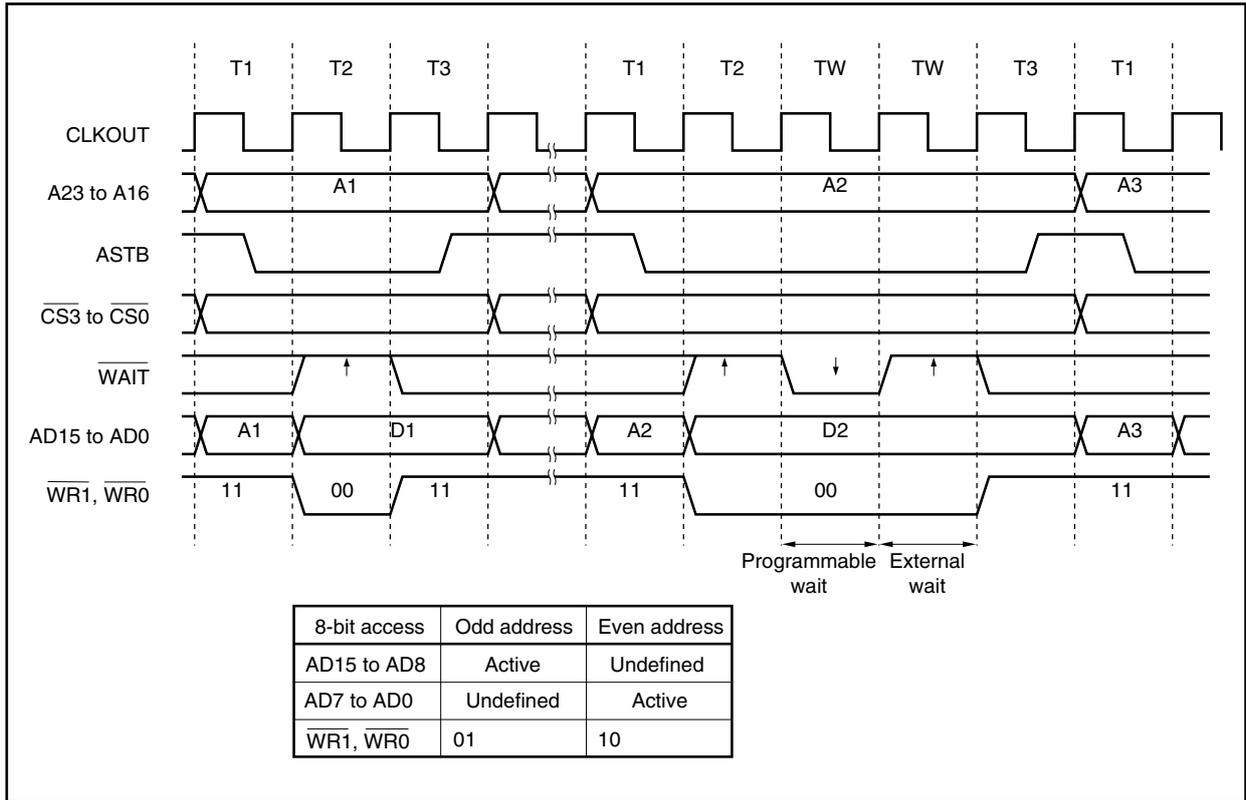
Figure 5-7. Multiplexed Bus Write Timing (Bus Size: 8 Bits)
