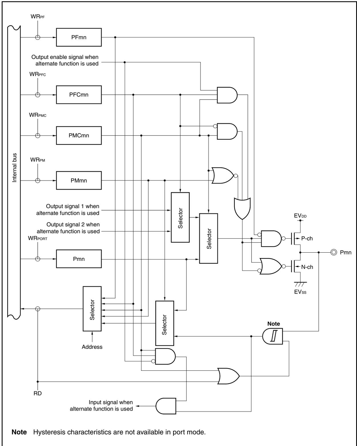
Figure 4-18. Block Diagram of Type G-6
