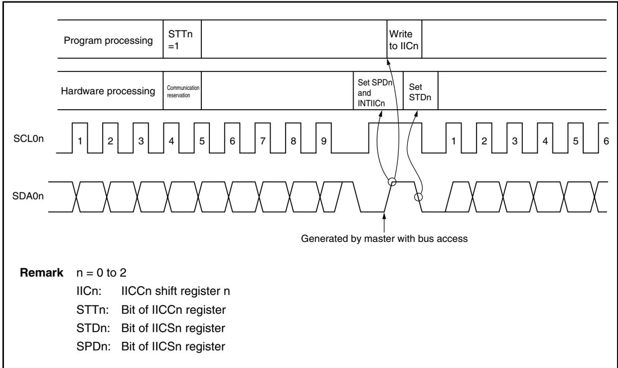
Communication reservations are accepted via the following timing. After the IICSn.STDn bit is set to 1, a communication reservation can be made by setting the IICn.STTn bit to 1 before a stop condition is detected (n = 0 to 2).
