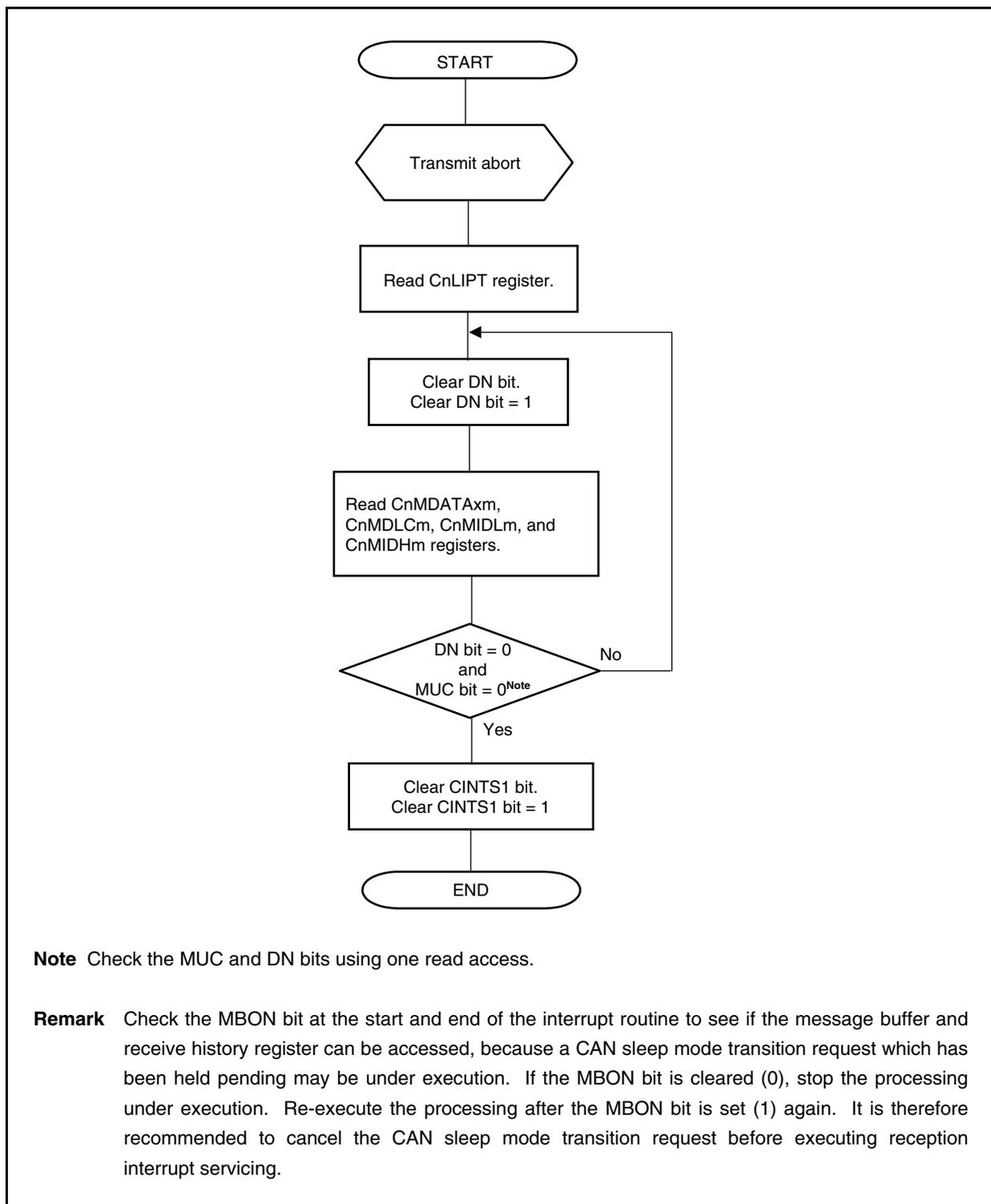
Figure 19-50. Reception via Interrupt (Using CnRGPT Register)
