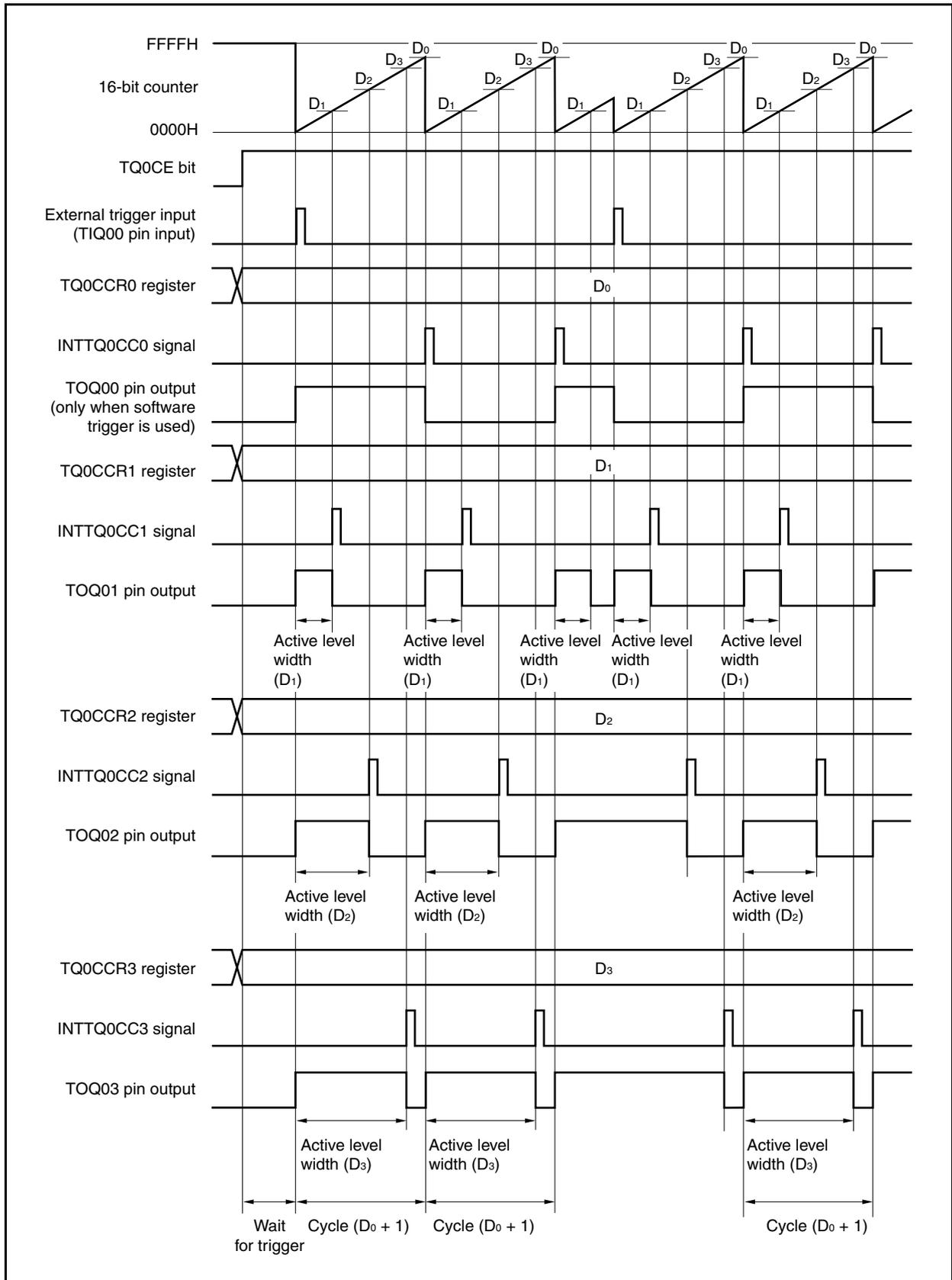
16-bit timer/event counter Q waits for a trigger when the TQ0CE bit is set to 1. When the trigger is generated, the 16-bit counter is cleared from FFFFH to 0000H, starts counting at the same time, and outputs a PWM waveform from the TOQ0k pin. If the trigger is generated again while the counter is operating, the counter is cleared to 0000H and restarted. (The output of the TOQ00 pin is inverted. The TOQ0k pin outputs a high-level regardless of the status (high/low) when a trigger occurs.)
