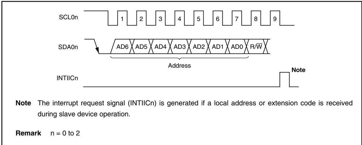
The slave address and the eighth bit, which specifies the transfer direction as described in **17.6.3 Transfer direction specification** below, are written together to IIC shift register n (IICn) and then output. Received addresses are written to the IICn register (n = 0 to 2).
