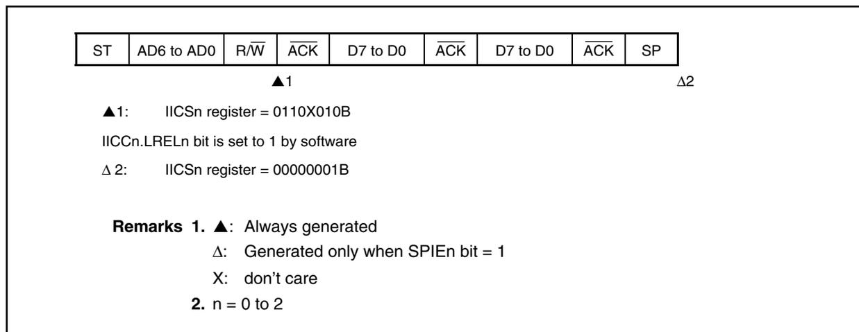
**(3) When arbitration loss occurs during data transfer****<1> When IICSn.WTIMn bit = 0**
