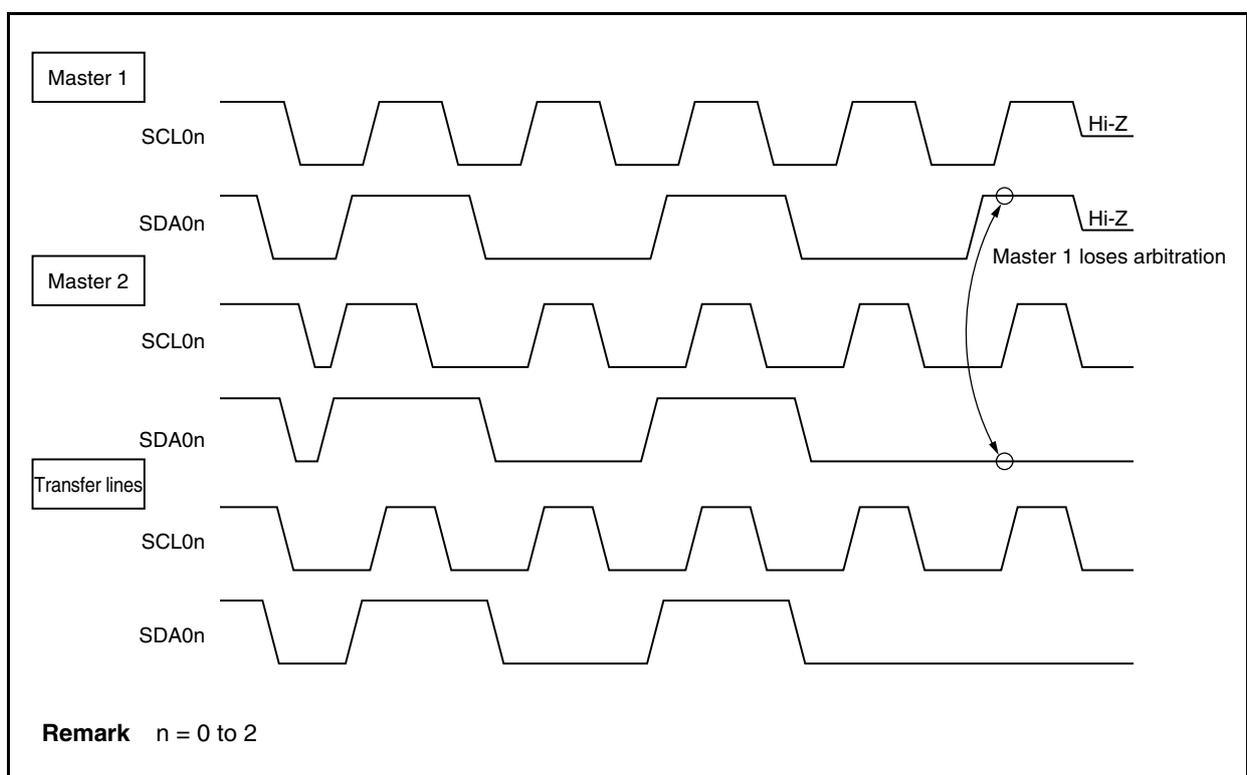
**Table 17-6. Status During Arbitration and Interrupt Request Signal Generation Timing**
