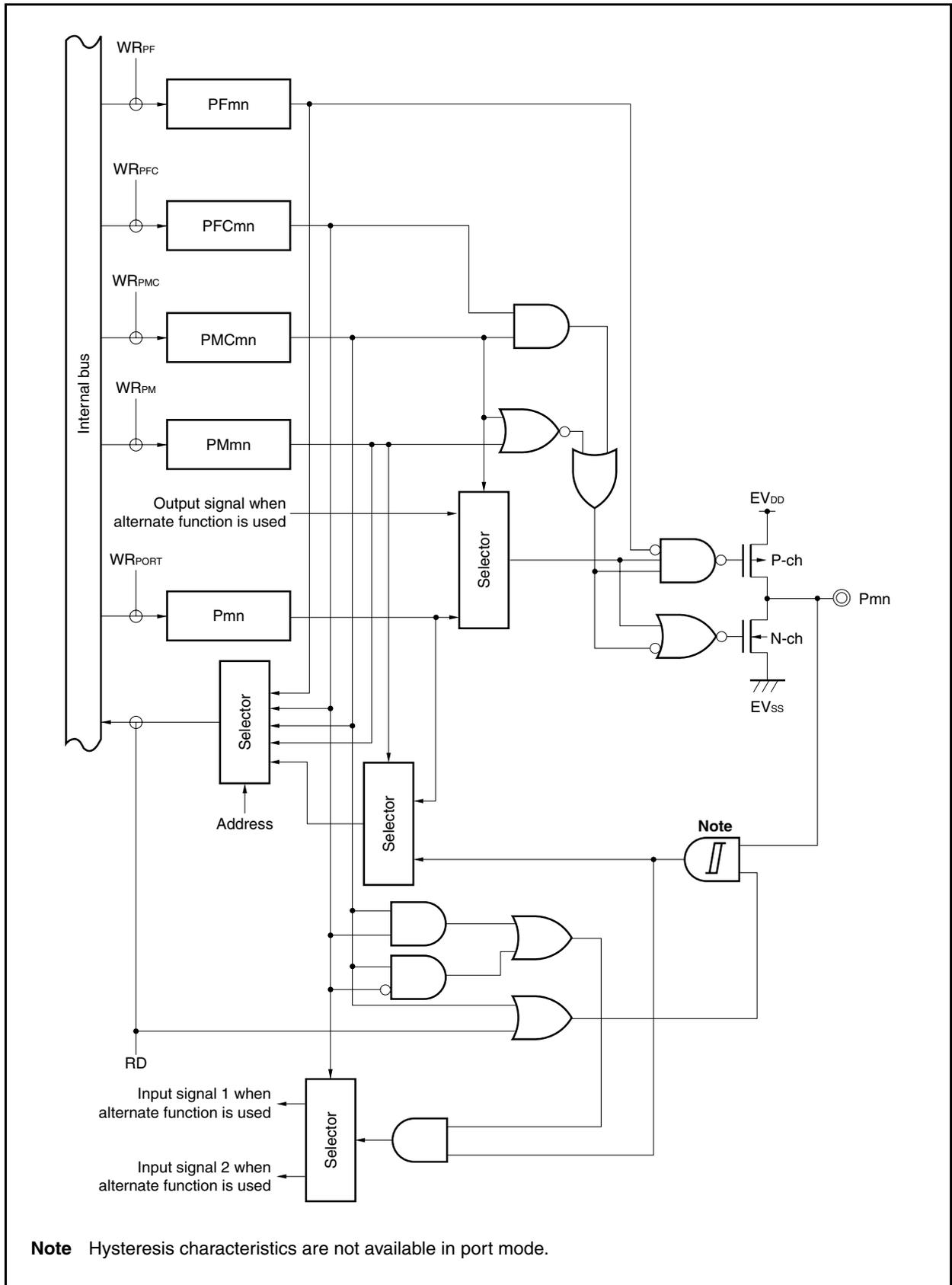
Figure 4-19. Block Diagram of Type G-12
