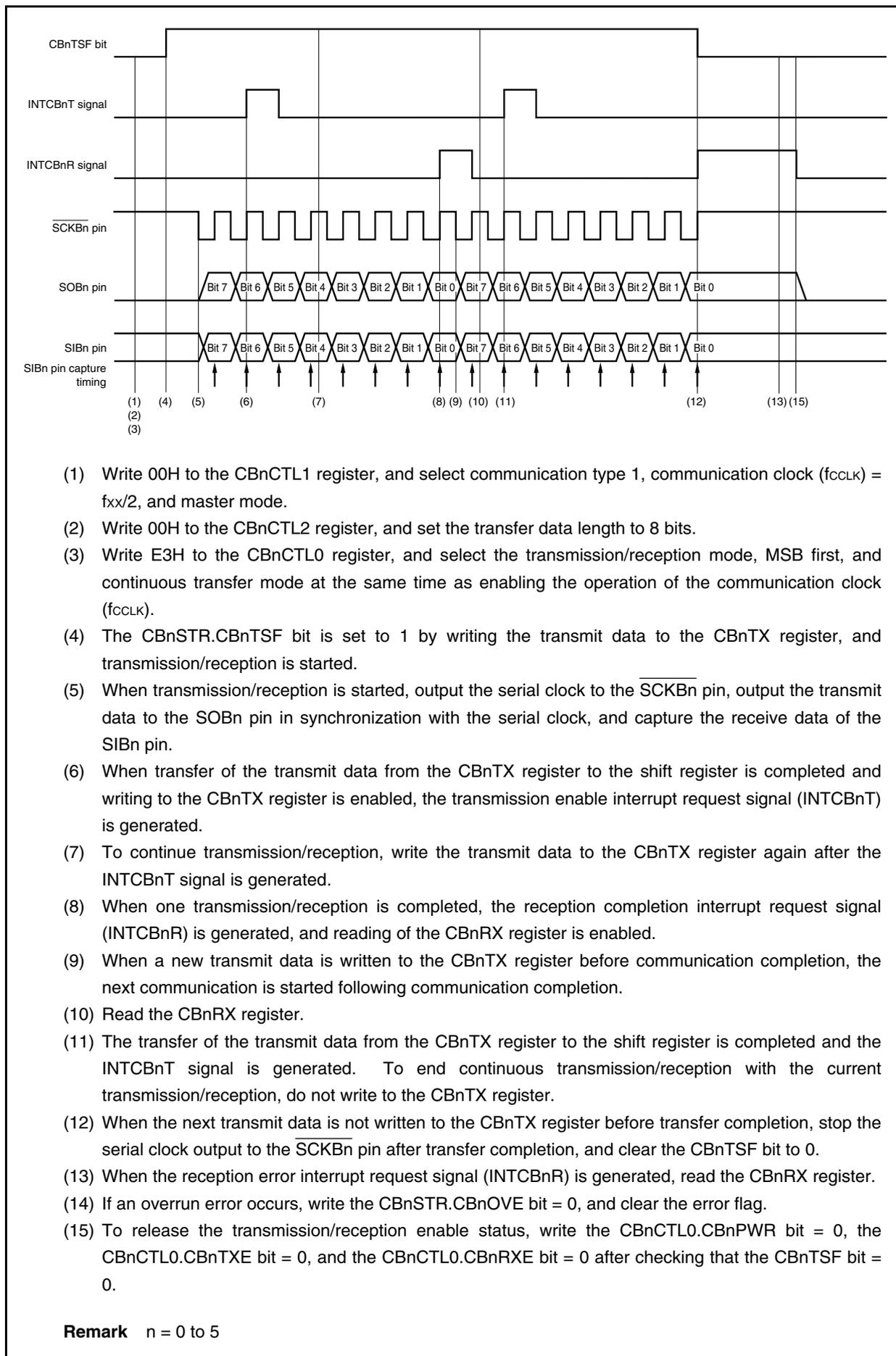
**16.6.10 Continuous transfer mode (slave mode, transmission mode)**
