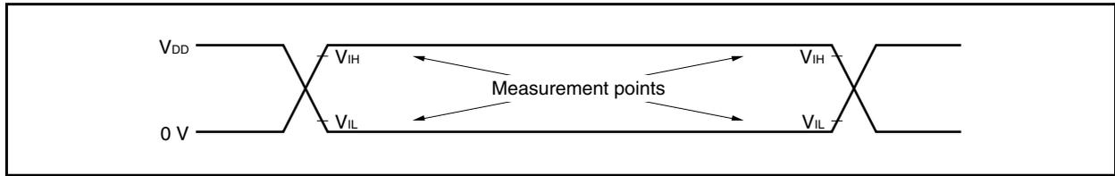
(2) AC Test Output Measurement Points
