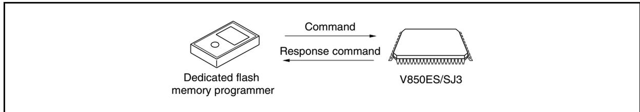
The following shows the commands for flash memory control in the V850ES/SJ3. All of these commands are issued from the dedicated flash memory programmer, and the V850ES/SJ3 performs the processing corresponding to the commands.
