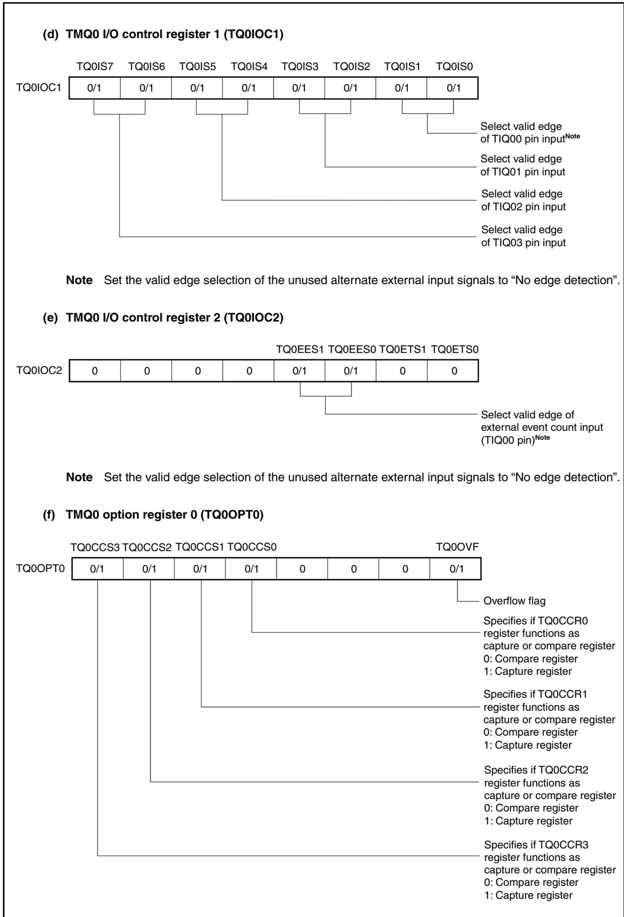
**Figure 8-35. Register Setting in Free-Running Timer Mode (3/3)****(g) TMQ0 counter read buffer register (TQ0CNT)**
