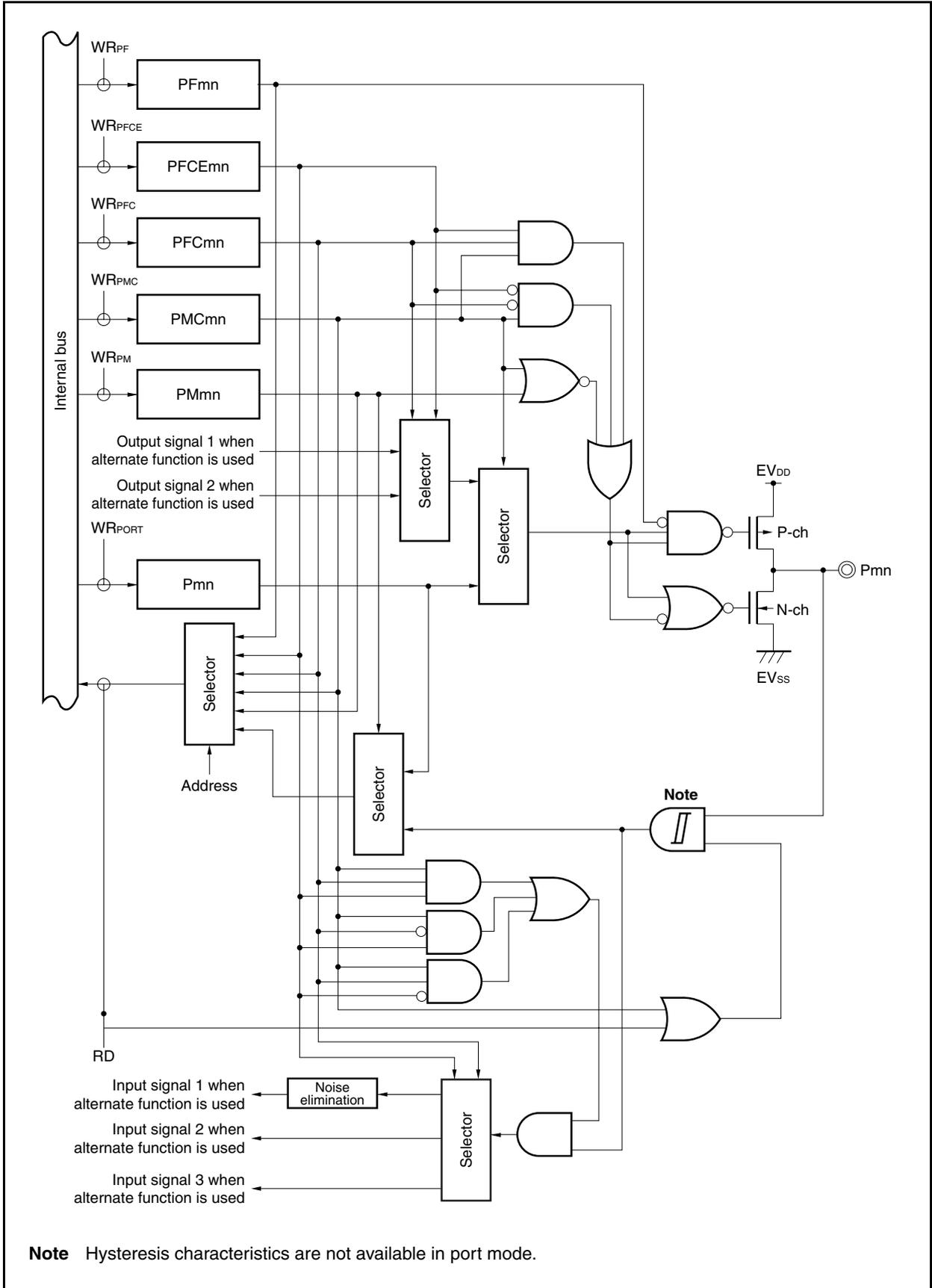
Figure 4-36. Block Diagram of Type U-12
