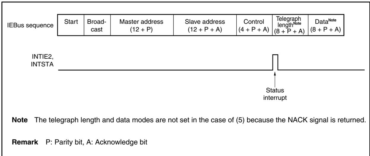
**Figure 18-19. Timing of INTIE2 and INTSTA Interrupt Request Signal Generation in Locked State (for (3))**
