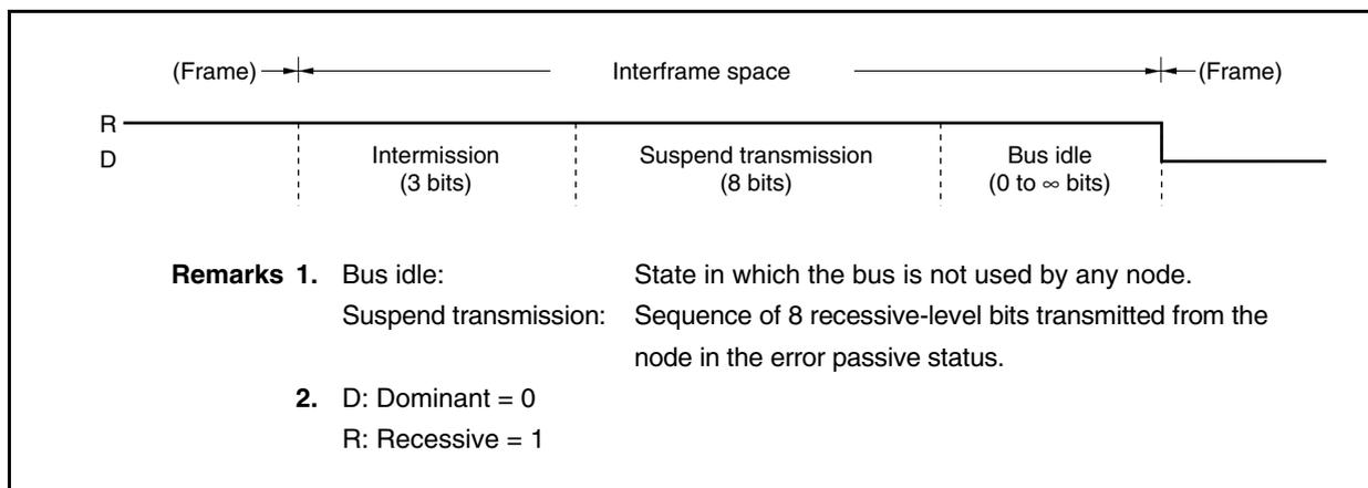
Usually, the intermission field is 3 bits. If the transmitting node detects a dominant level at the third bit of the intermission field, however, it executes transmission.
