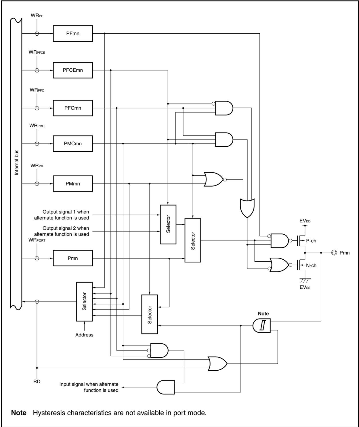
Figure 4-29. Block Diagram of Type U-5
