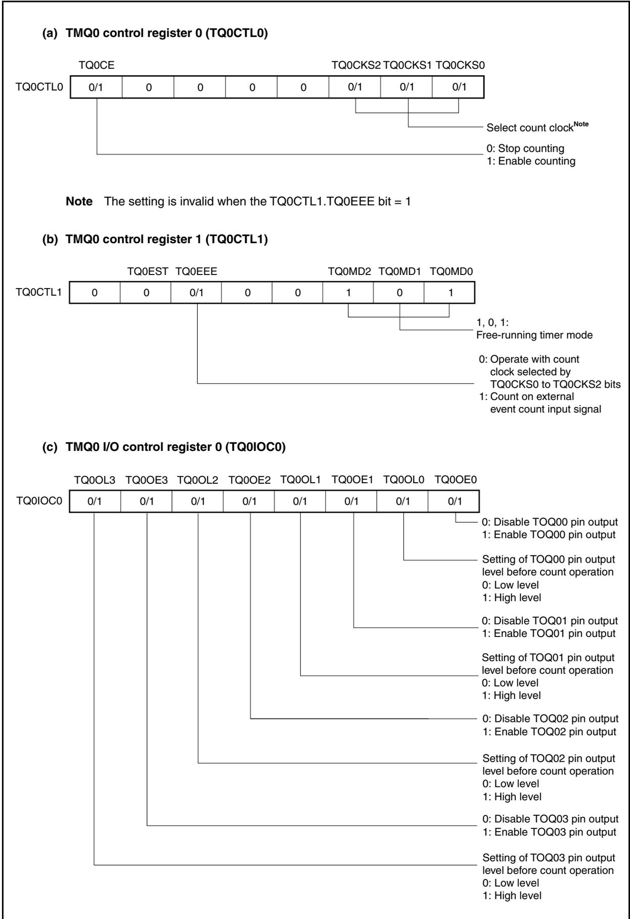
Figure 8-35. Register Setting in Free-Running Timer Mode (2/3)
