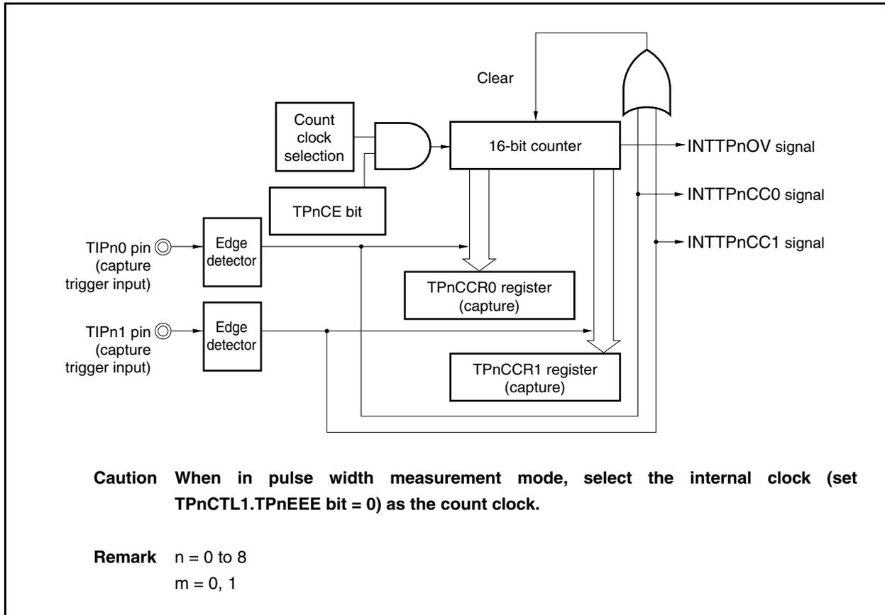
Figure 7-39. Basic Timing in Pulse Width Measurement Mode
