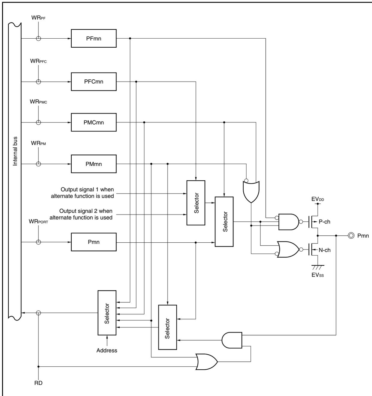
Figure 4-16. Block Diagram of Type G-4
