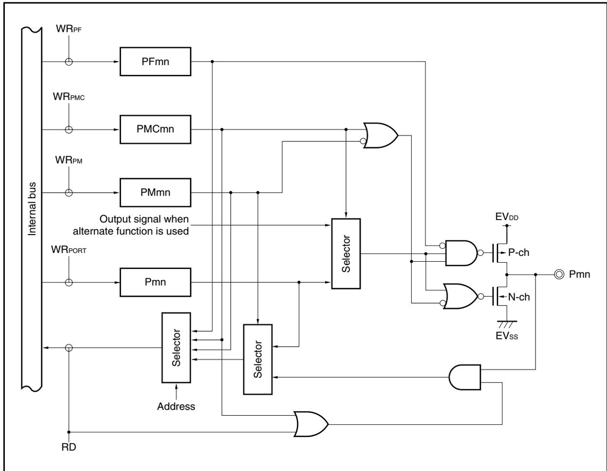
Figure 4-12. Block Diagram of Type E-3
