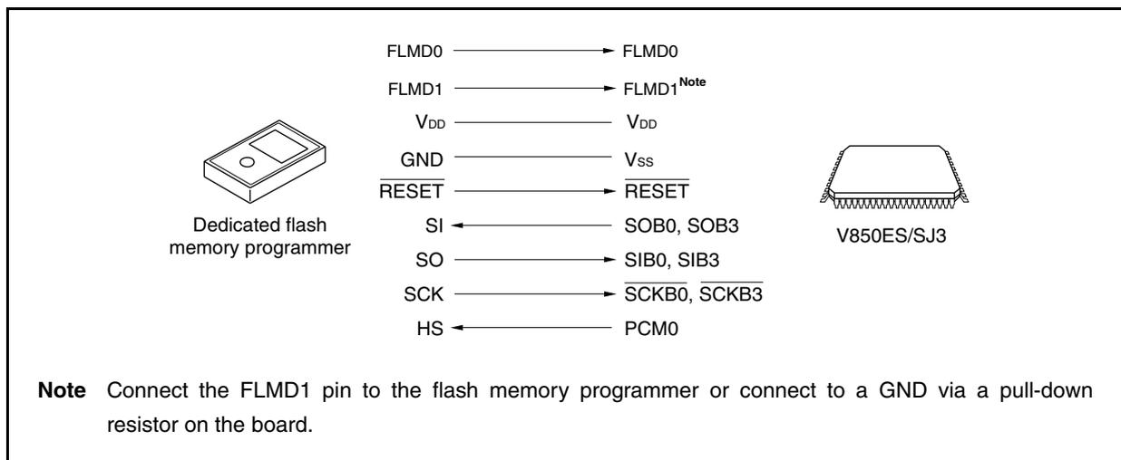
The dedicated flash memory programmer outputs the transfer clock, and the V850ES/SJ3 operates as a slave.
