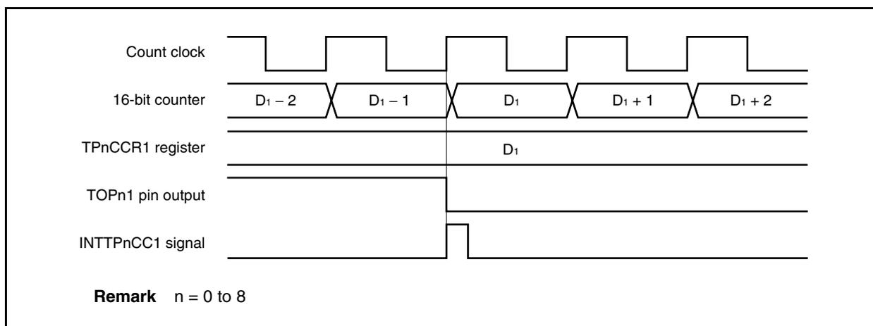
Usually, the INTTPnCC1 signal is generated in synchronization with the next count up, after the count value of the 16-bit counter matches the value of the TPnCCR1 register.
