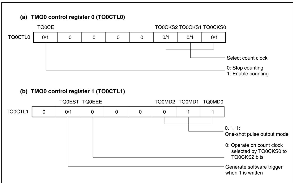
Figure 8-26. Register Setting in One-Shot Pulse Output Mode (2/3)
