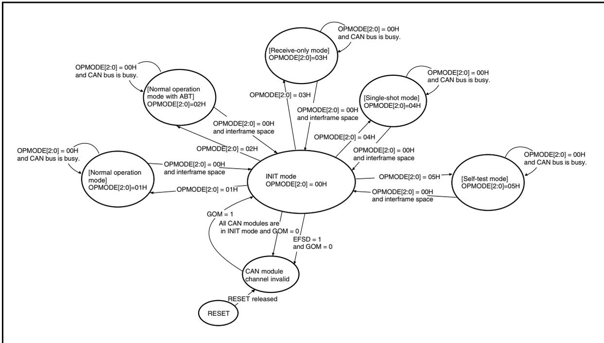
The transition from the initialization mode to an operation mode is controlled by the CnCTRL.OPMODE2 to CnCTRL.OPMODE0 bits.
