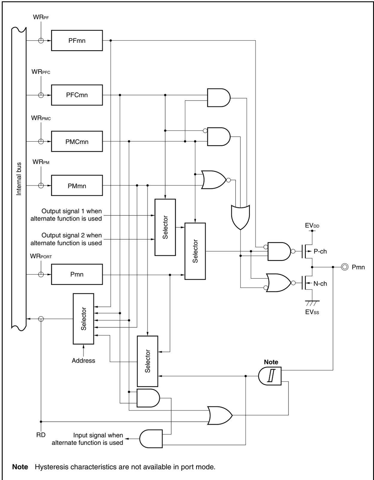
Figure 4-20. Block Diagram of Type L-1
