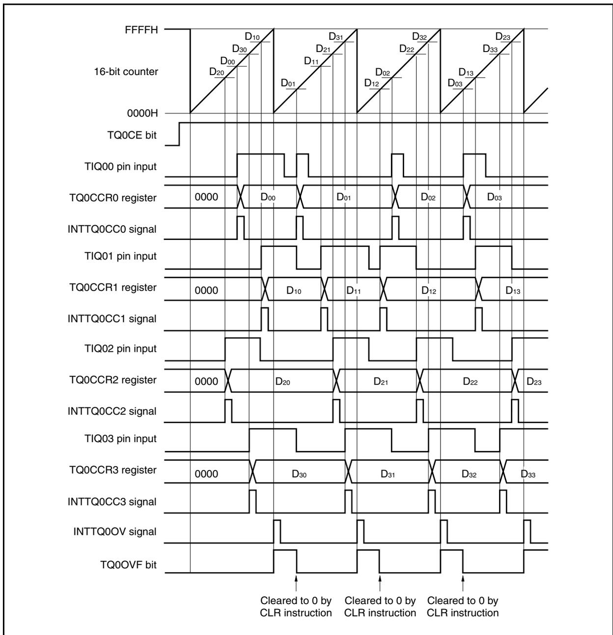
Figure 8-35. Register Setting in Free-Running Timer Mode (1/3)
