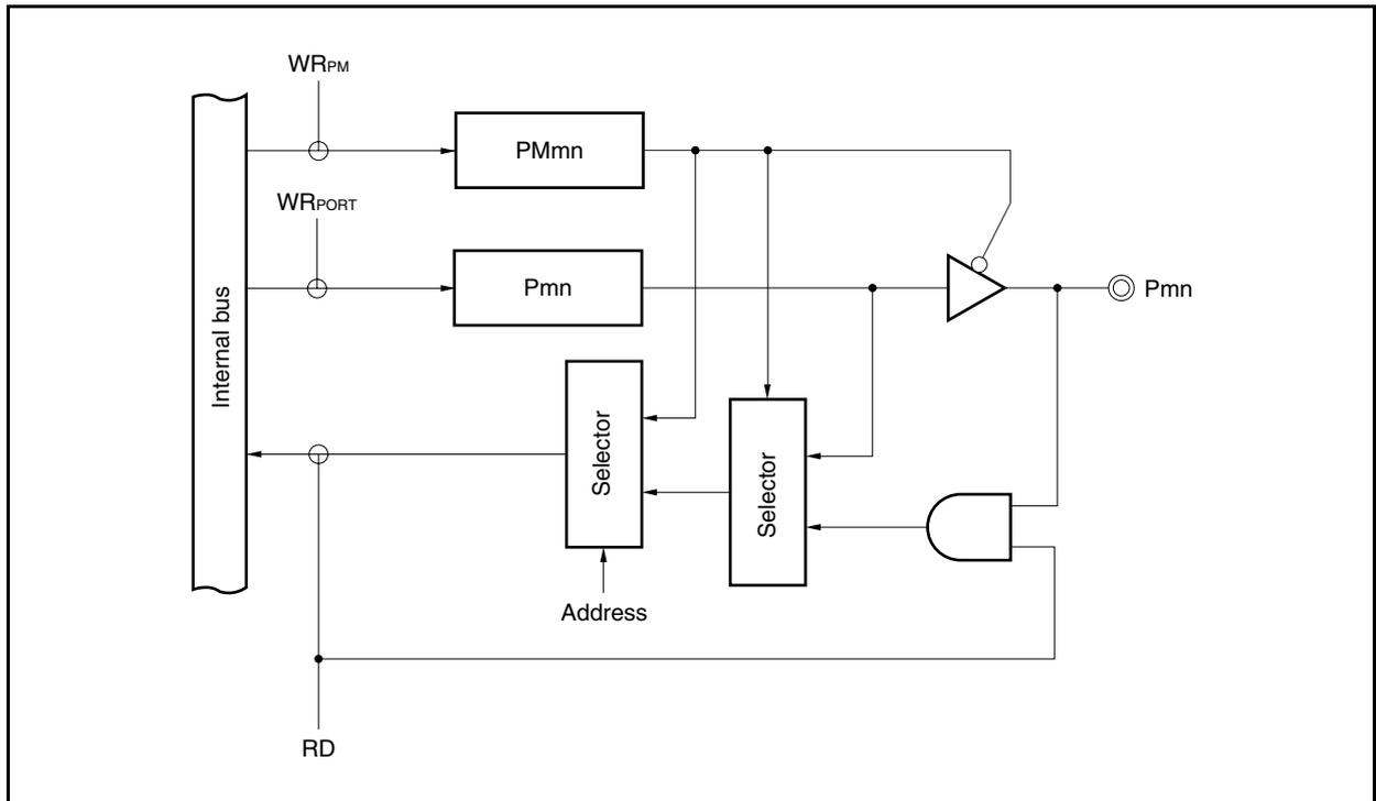
Figure 4-6. Block Diagram of Type C-1
