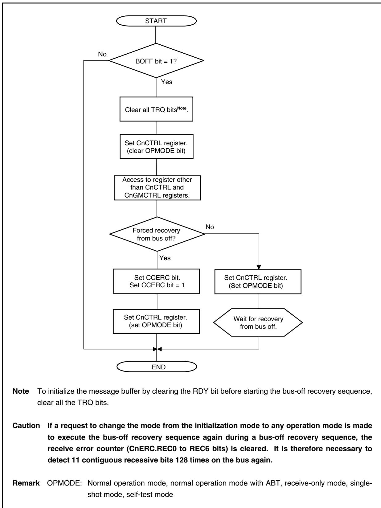
Figure 19-55. Bus-off Recovery (Normal Operation Mode with ABT)
