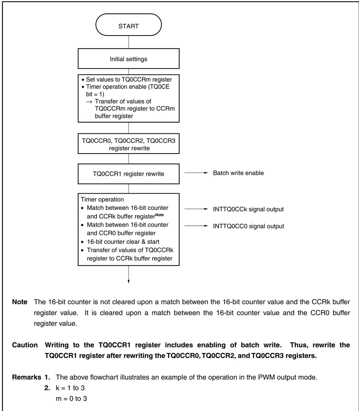
Figure 8-5. Timing of Batch Write
