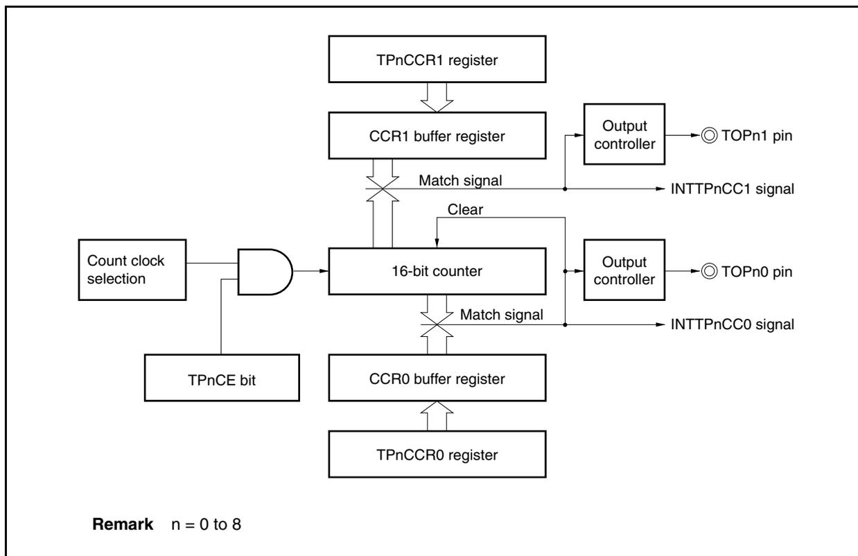
When the TPnCCR1 register is set to the same value as the TPnCCR0 register, the INTTPnCC1 signal is generated at the same timing as the INTTPnCC0 signal and the TOPn1 pin output is inverted. In other words, a square wave with a duty factor of 50% can be output from the TOPn1 pin.
