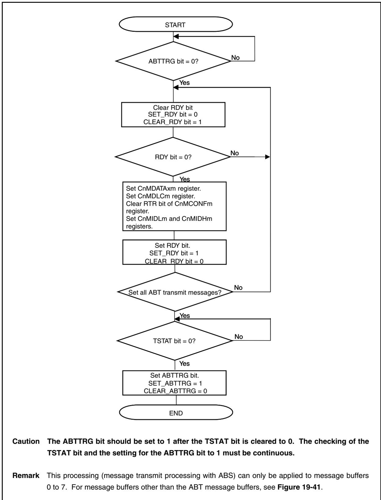
**Caution** The ABTTRG bit should be set to 1 after the TSTAT bit is cleared to 0. The checking of the TSTAT bit and the setting for the ABTTRG bit to 1 must be continuous.
