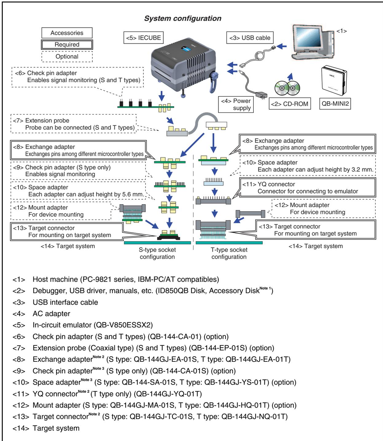
Figure A-3. System Configuration (QB-V850ESSX2 Used) (2/2)
