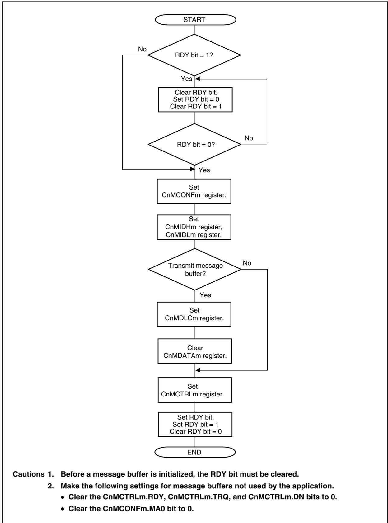
Figure 19-39 shows the processing for a receive message buffer (CnMCONFm.MT2 to CnMCONFm.MT0 bits = 001B to 101B).
