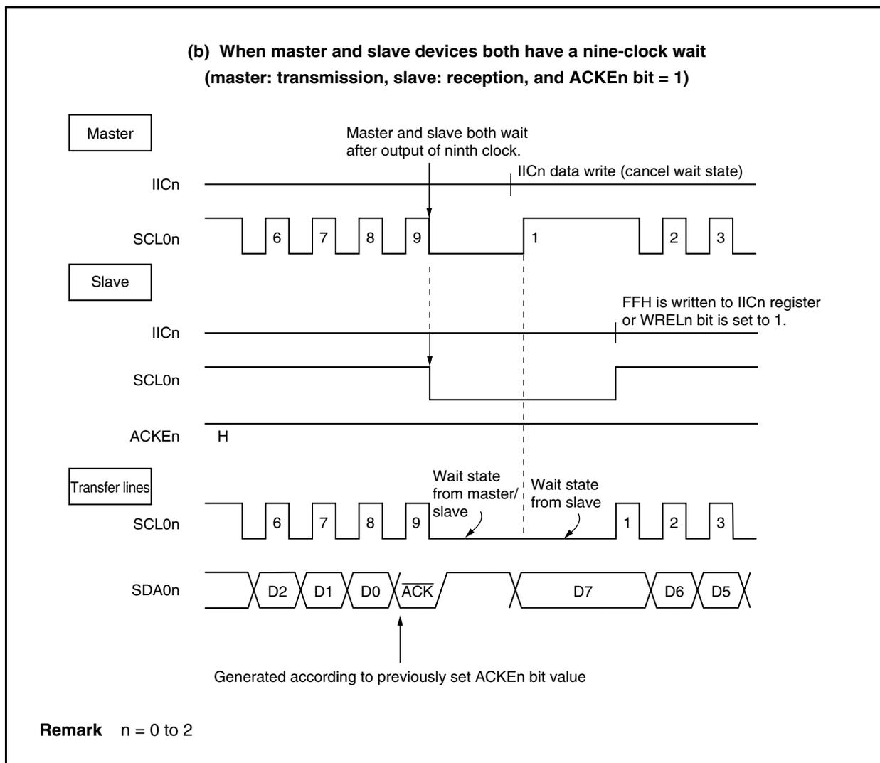
A wait state is automatically generated after generation of the start condition. A wait state is also automatically generated depending on the setting of the IICn.WTIMn bit (n = 0 to 2).
