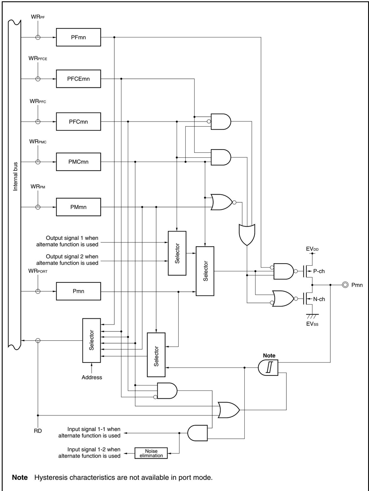
Figure 4-30. Block Diagram of Type U-6
