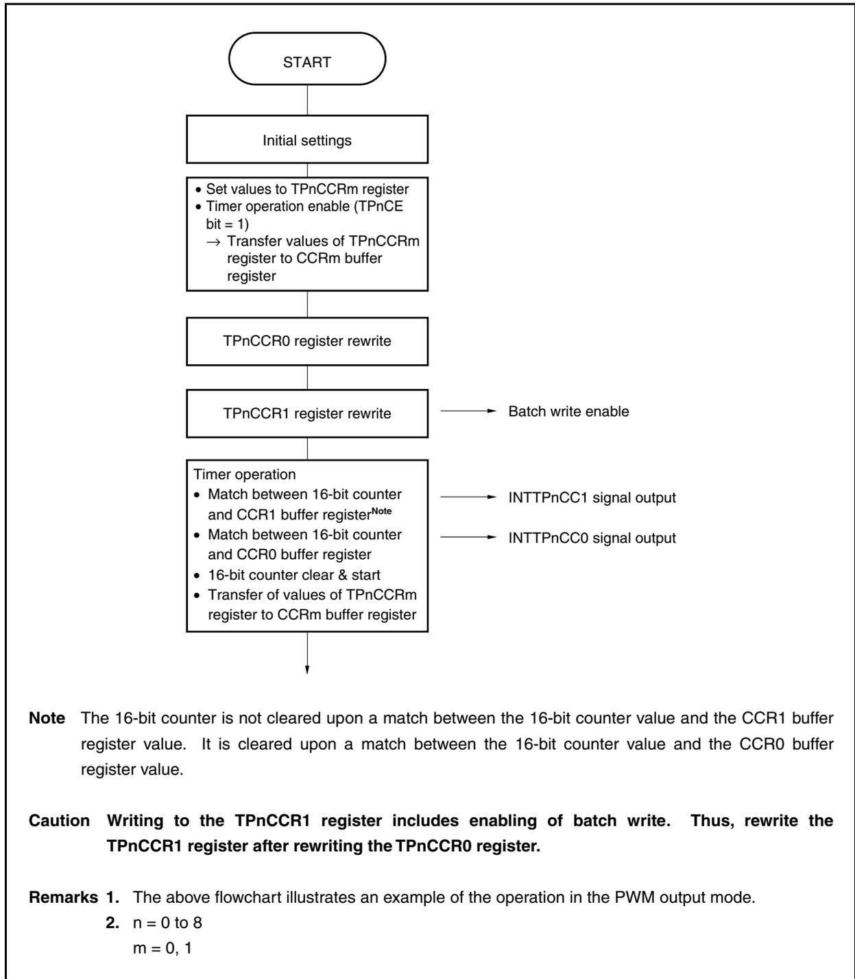
Figure 7-5. Timing of Batch Write
