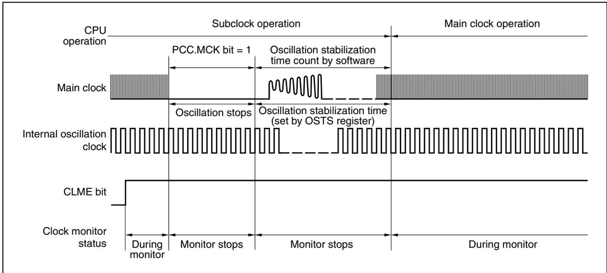
**(5) Operation while CPU is operating on internal oscillation clock (CCLS.CCLSF bit = 1)**
