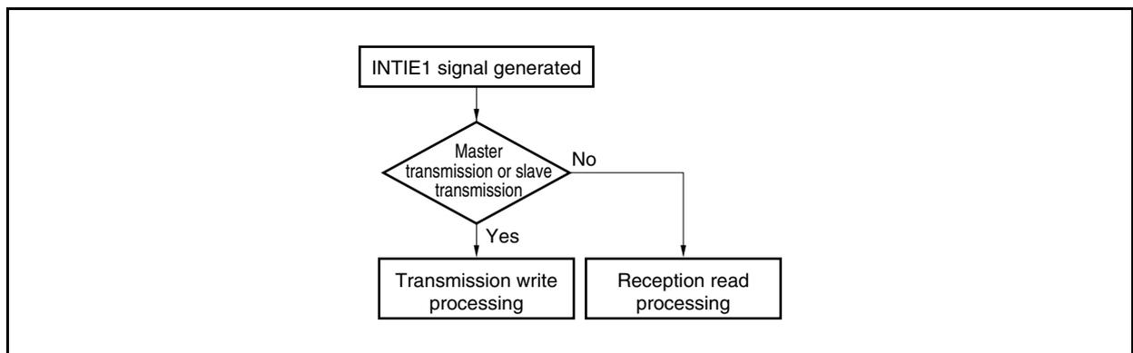
**Figure 18-22. Example of Identifying INTERR Signal Interrupt
