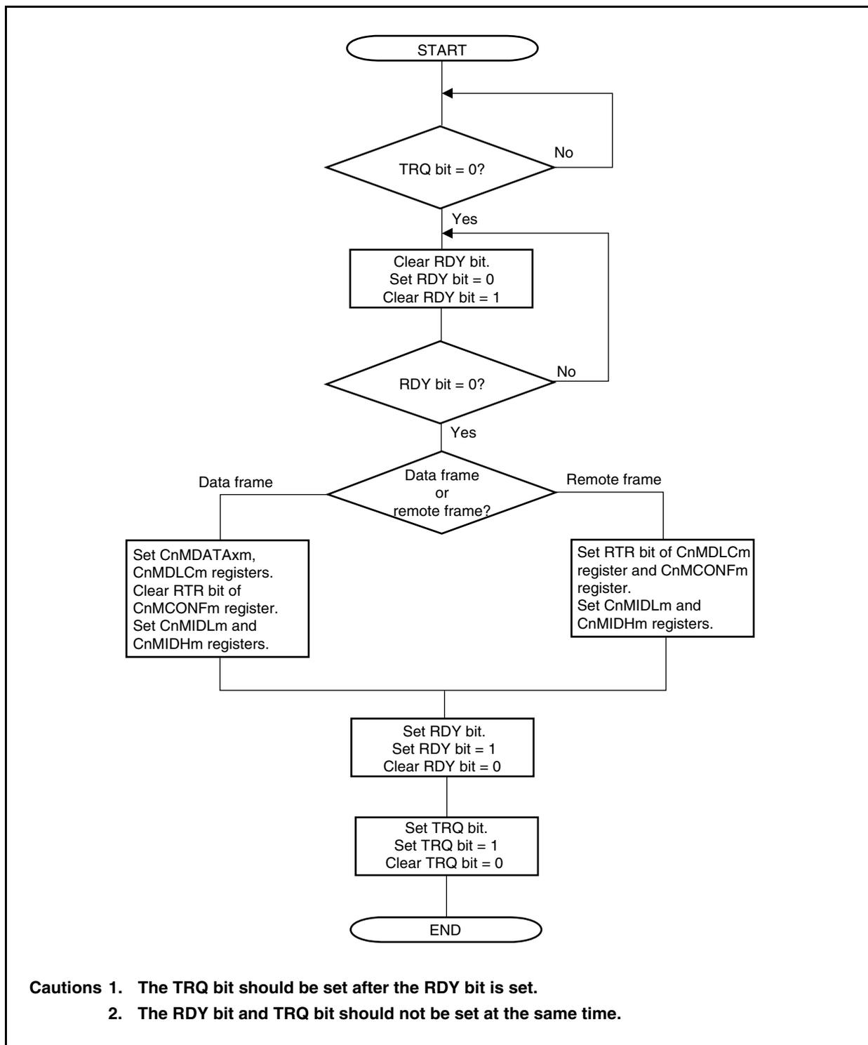
Figure 19-42 shows the processing for a transmit message buffer (CnMCONFm.MT2 to CnMCONFm.MT0 bits = 000B).
