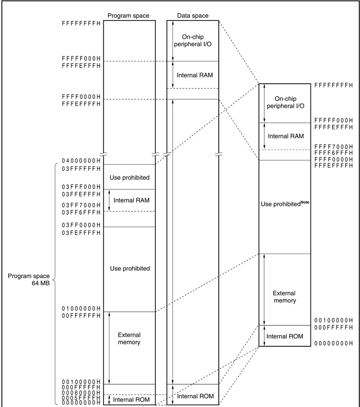
**Note** In the CAN controller versions, the data space of addresses 03FEC000H to 03FEEFFFH is assigned as the programmable peripheral I/O area. Only the programmable peripheral I/O area is seen as images of 256 MB each in the 4 GB address space.
