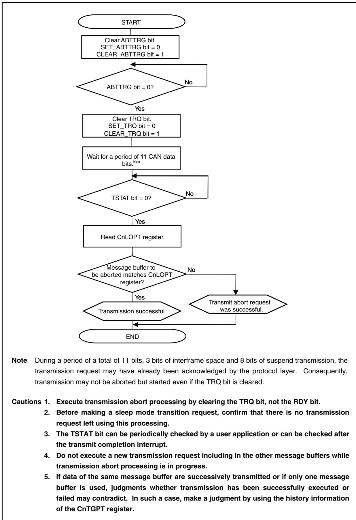
**Note** During a period of a total of 11 bits, 3 bits of interframe space and 8 bits of suspend transmission, the transmission request may have already been acknowledged by the protocol layer. Consequently, transmission may not be aborted but started even if the TRQ bit is cleared.
