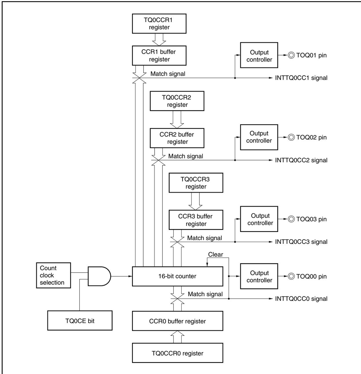
If the same value as the set value of the TQ0CCR0 register is set to the TQ0CCRk register, the INTTQ0CCk signal is generated together with the INTTQ0CC0 signal, and the output of the TOQ0k pin is inverted. This means that a square wave with a duty factor of 50% can be output from the TOQ0k pin. If a value different from the set value of the TQ0CCR0 register is set to the TQ0CCRk register, the operation is as follows.
