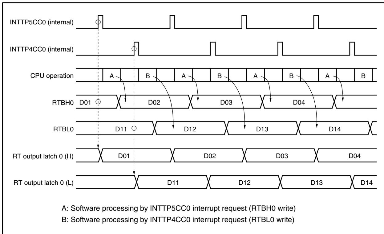
**Figure 12-2. Example of Operation Timing and Software Processing of RTO0
