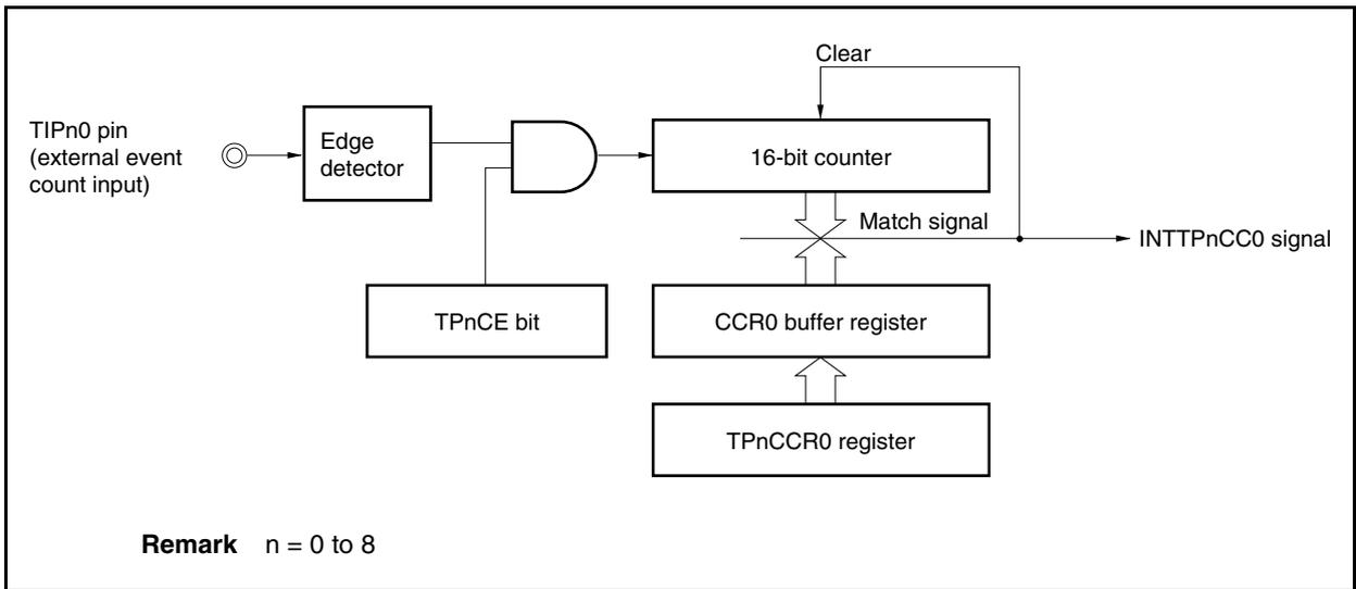
**Figure 7-14. Basic Timing in External Event Count Mode**
