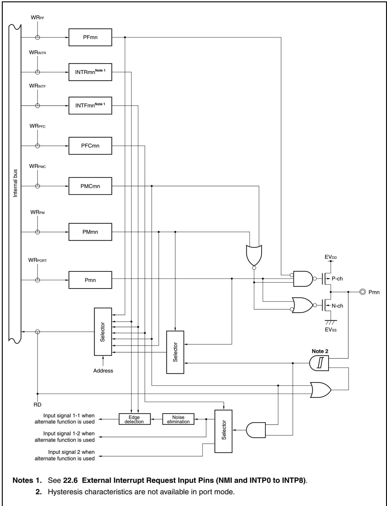
Figure 4-25. Block Diagram of Type U-1
