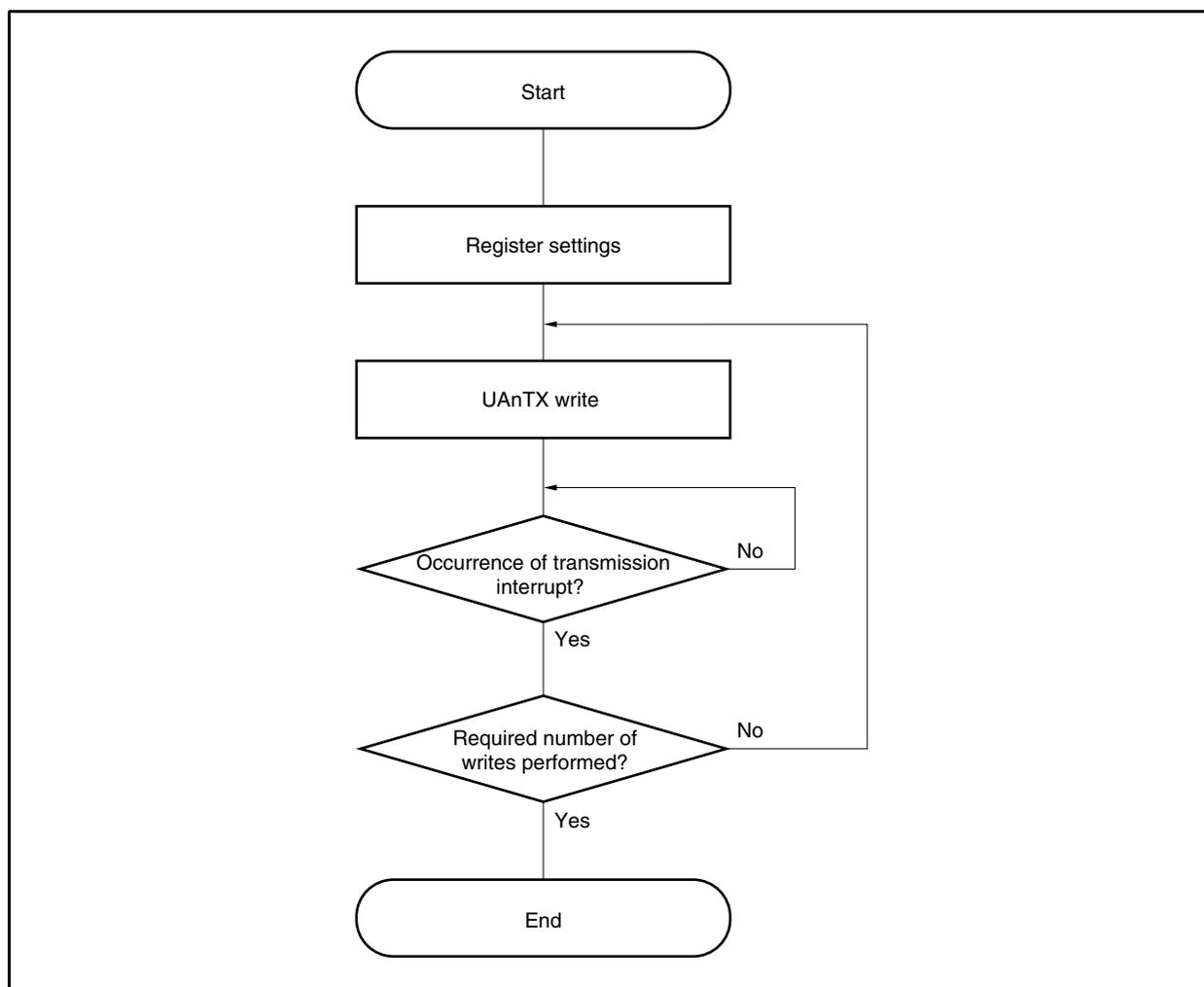
Figure 15-10. Continuous Transmission Operation Timing
