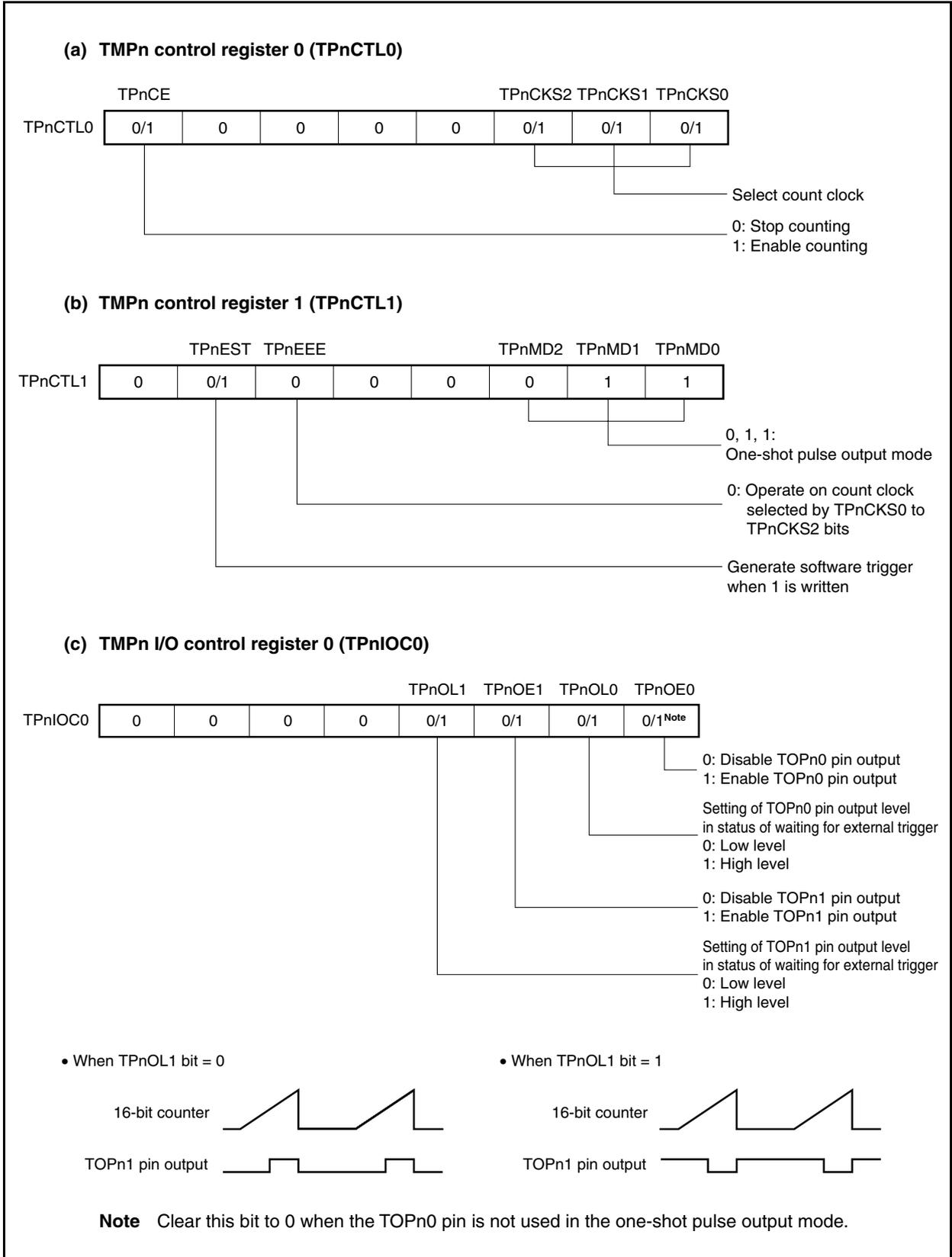
Figure 7-26. Setting of Registers in One-Shot Pulse Output Mode (2/2)
