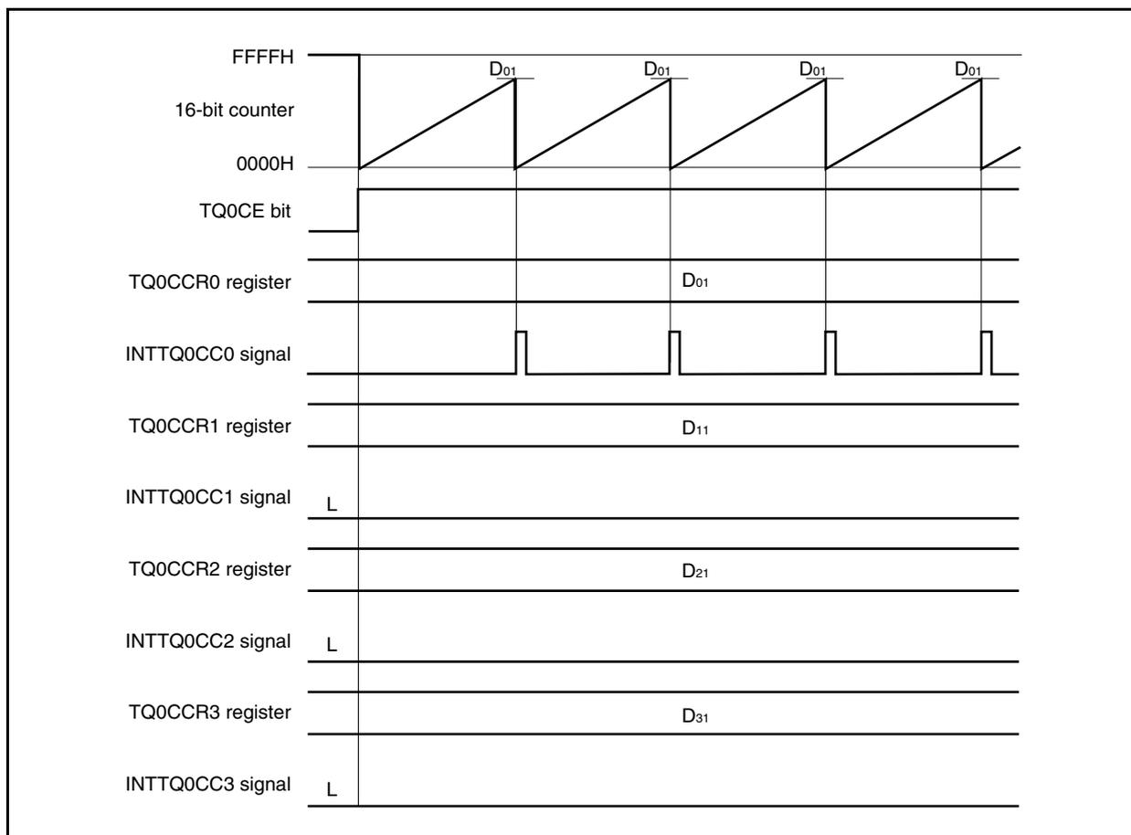
**8.6.3 External trigger pulse output mode (TQ0MD2 to TQ0MD0 bits = 010)**
