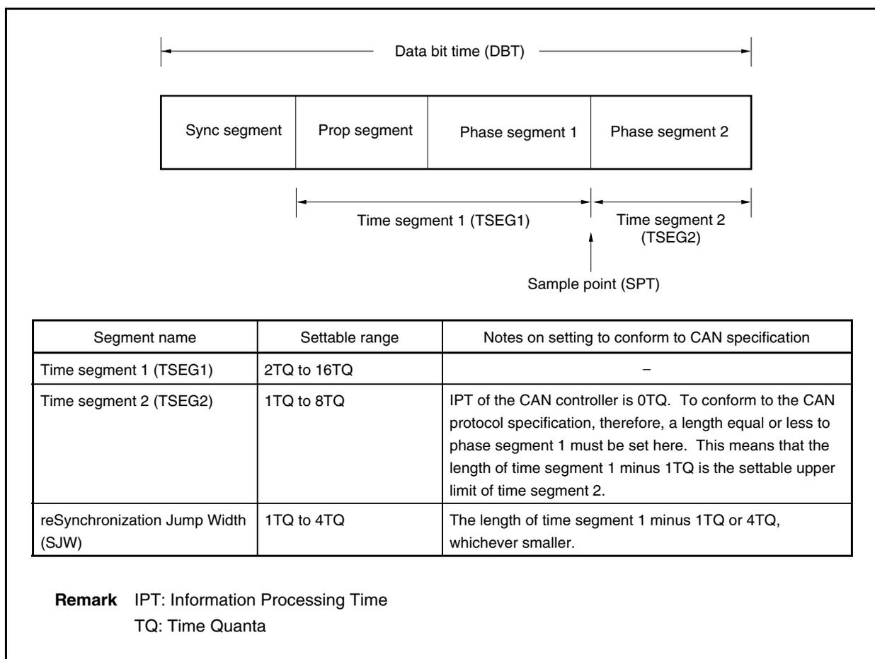
**Remark** The CAN protocol specification defines the segments constituting the data bit time as shown in Figure 19-19.
