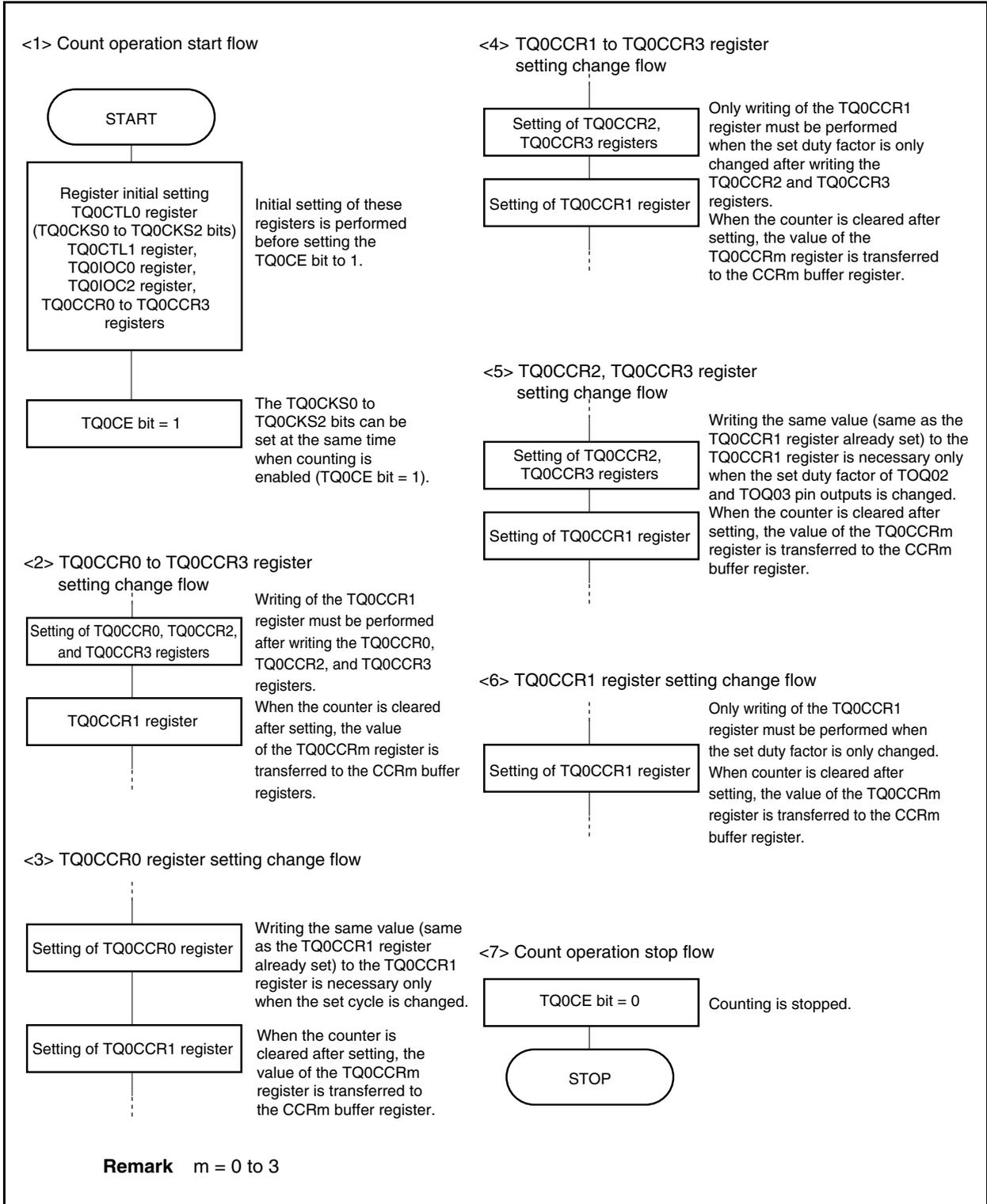
**(2) PWM output mode operation timing****(a) Changing pulse width during operation**
