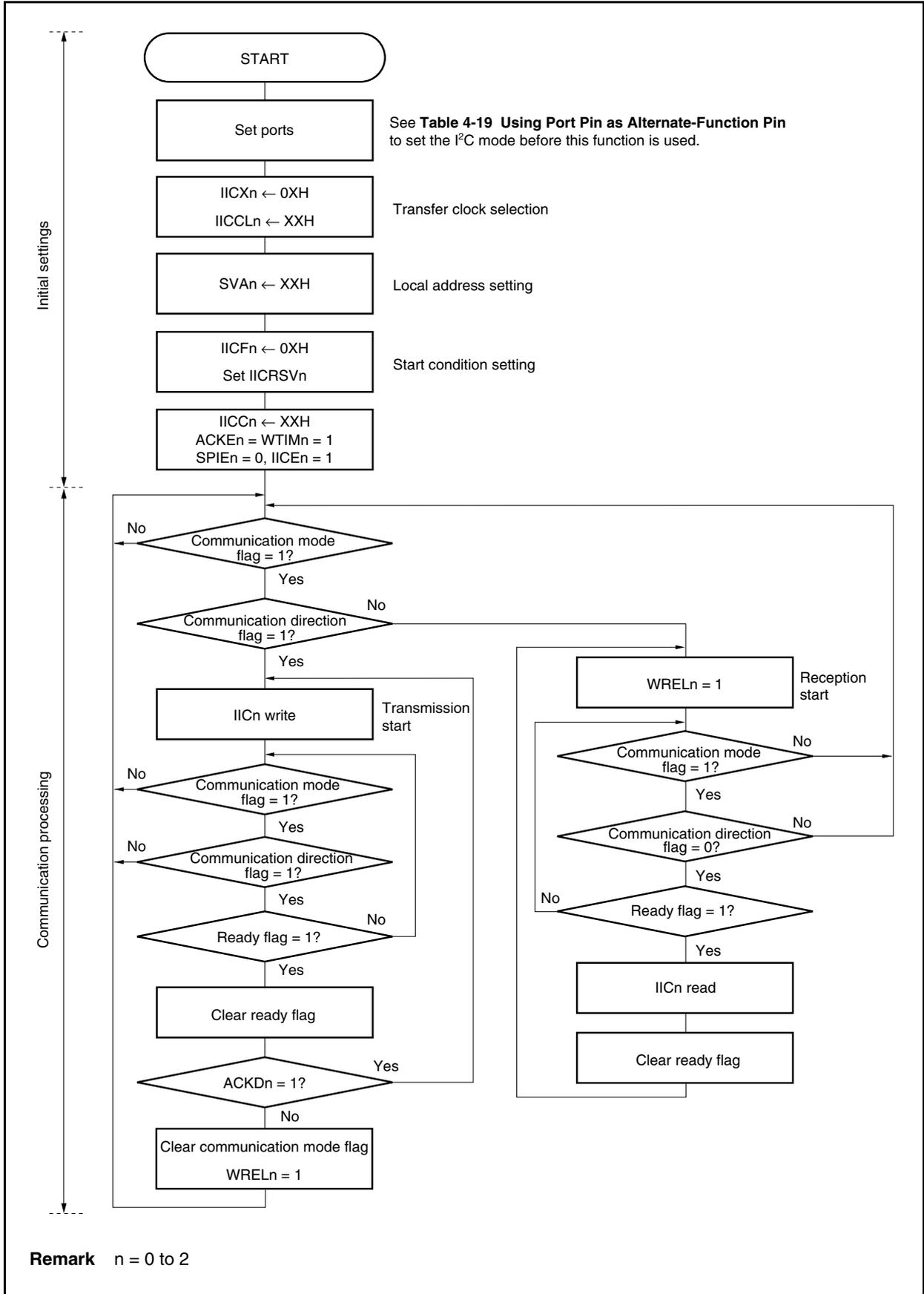
The following shows an example of the processing of the slave device by an INTIICn interrupt (it is assumed that no extension codes are used here). During an INTIICn interrupt, the status is confirmed and the following steps are executed.
