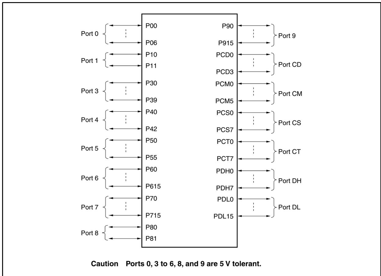
Table 4-1. I/O Buffer Power Supplies for Pins
