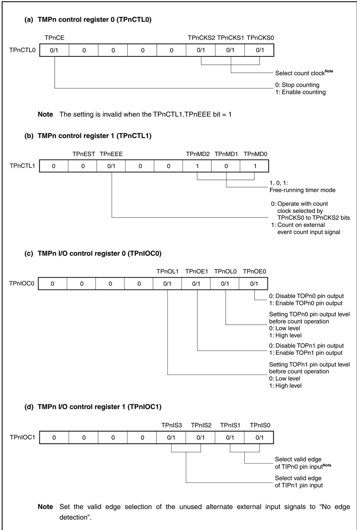
Figure 7-35. Register Setting in Free-Running Timer Mode (2/2)
