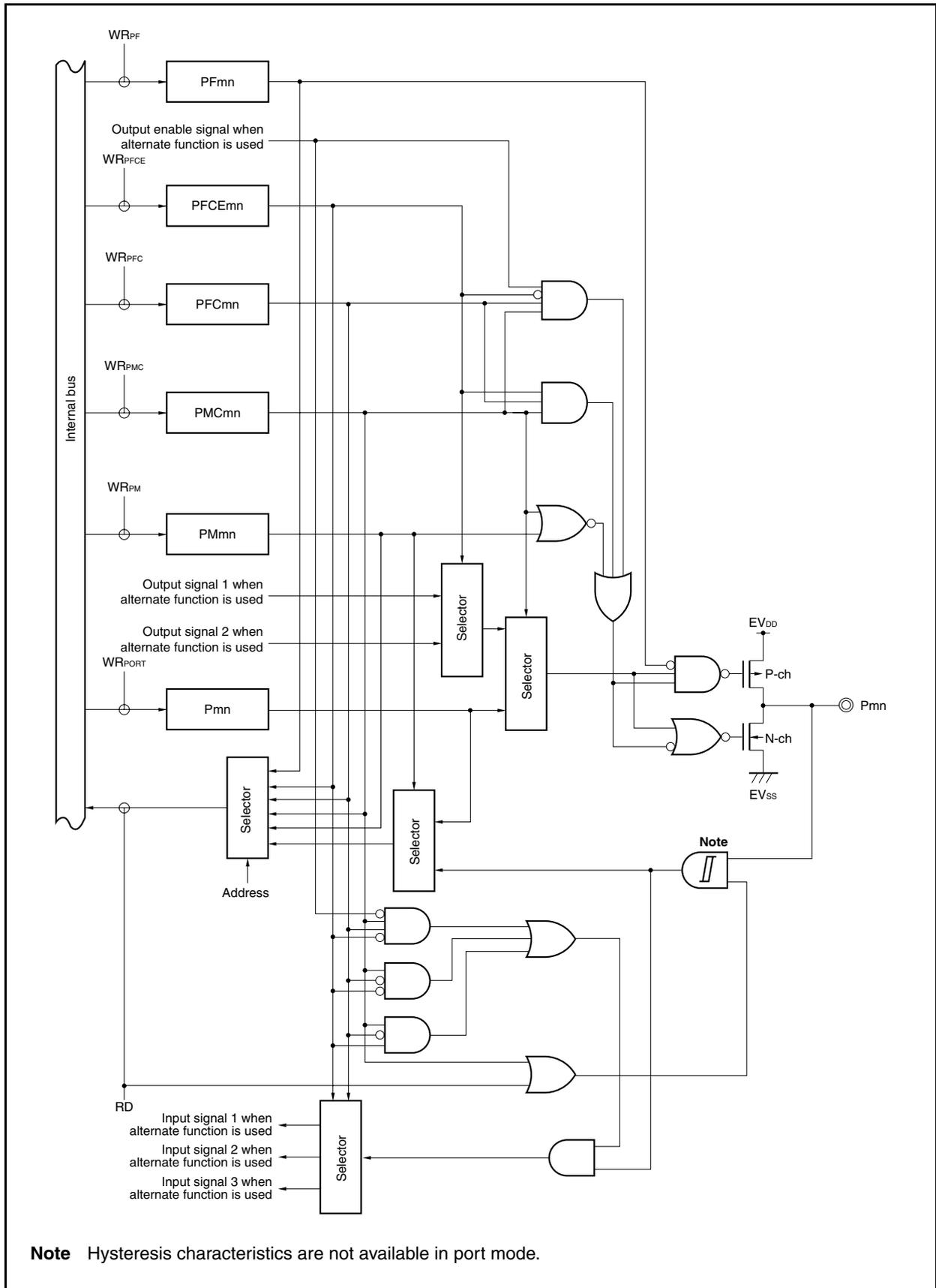
Figure 4-26. Block Diagram of Type U-2
