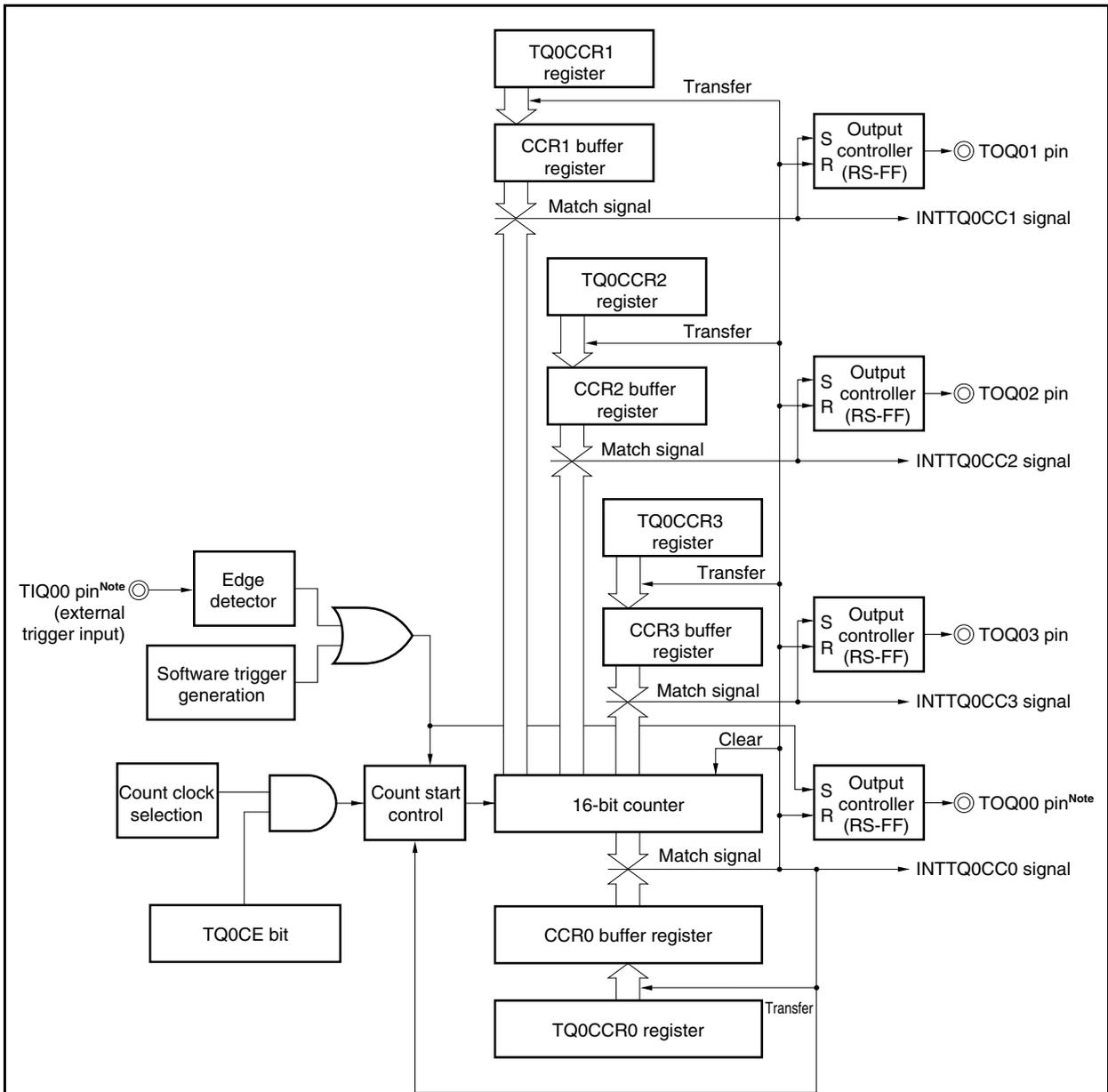
**Note** Because the external trigger input pin (TIQ00) and timer output pin (TOQ00) share the same alternate-function pin, two functions cannot be used at the same time.
