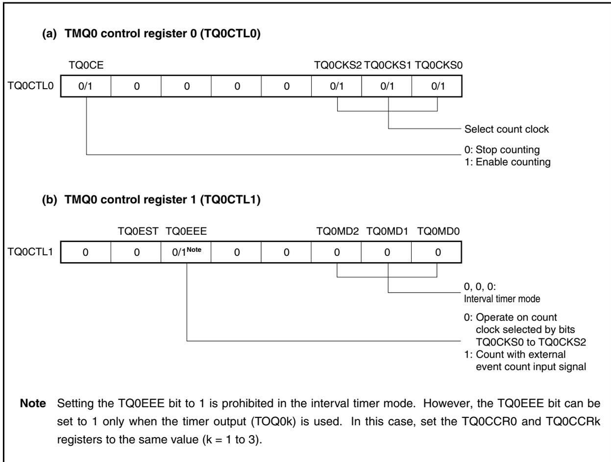
Figure 8-8. Register Setting for Interval Timer Mode Operation (2/3)
