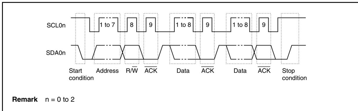
The master device generates the start condition, slave address, and stop condition.
