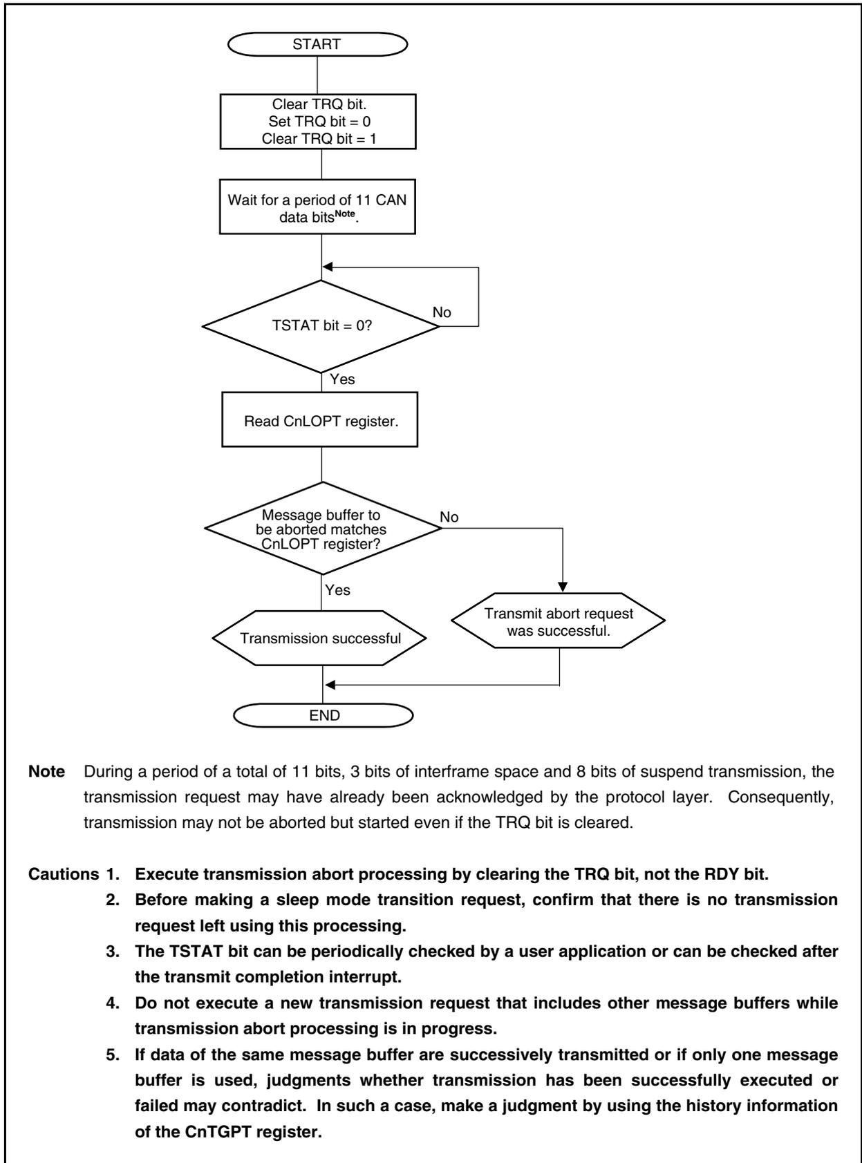
**Figure 19-47. Transmission Abort Processing Except for ABT Transmission
