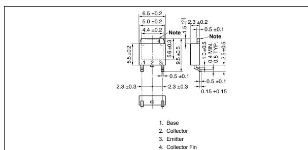
**Note** The depth of notch at the top of the fin is from 0 to 0.2 mm.
