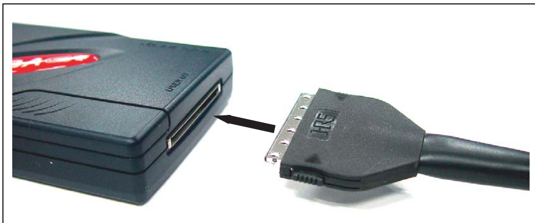
Figure 2.2 Connecting the E10A-USB Emulator to the User System Interface Cable
