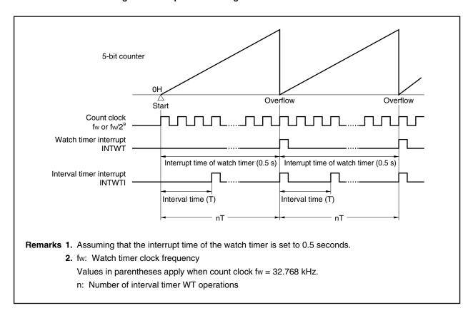
Figure 11-3. Operation Timing of Watch Timer/Interval Timer
