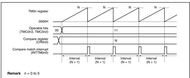
Figure 8-4. Example of Register Settings for Interval Timer Operation
