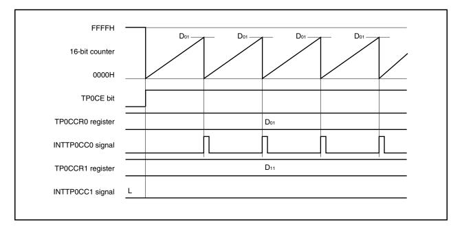
Figure 7-15. Timing Chart When D<sub>01</sub> < D<sub>11</sub>
