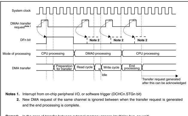
Figure 20-3. Period in Which DMA Transfer Request Is Ignored (1)
