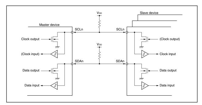
Figure 19-4. Pin Configuration Diagram
