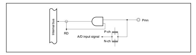
Figure 4-3. Block Diagram of Type C-N
