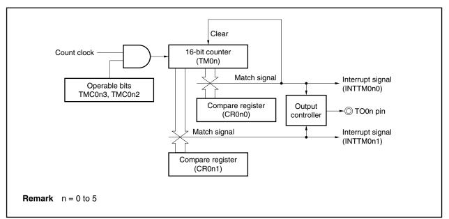
Figure 8-31. Block Diagram of PPG Output Operation
