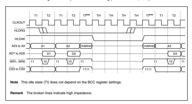
Figure 5-13. Separate Bus Hold Timing (Bus Size: 8 Bits, Write)
