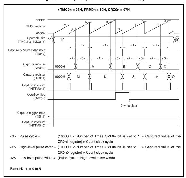
Figure 8-41. Timing Example of Pulse Width Measurement (3)
