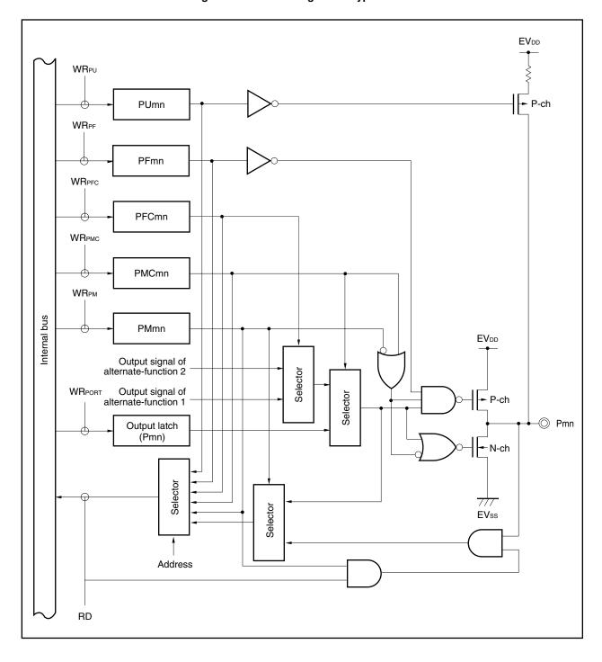
Figure 4-19. Block Diagram of Type E00-UF
