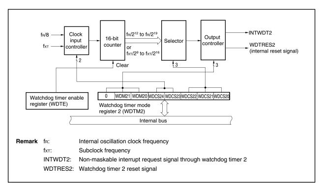
Figure 12-2. Block Diagram of Watchdog Timer 2
