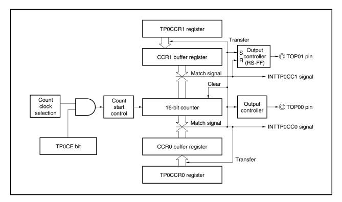
Figure 7-24. Configuration in PWM Output Mode
