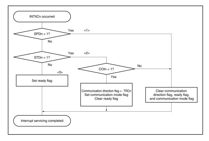
Figure 19-20. Slave Operation Flowchart (2)
