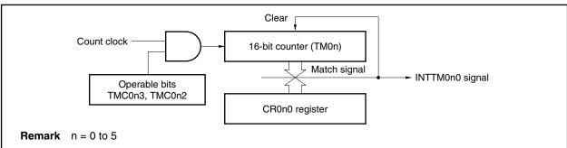
Figure 8-2. Block Diagram of Interval Timer Operation
