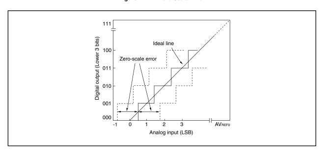
Figure 14-14. Zero-Scale Error
