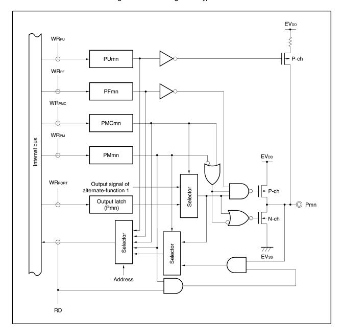
Figure 4-7. Block Diagram of Type D0-UF
