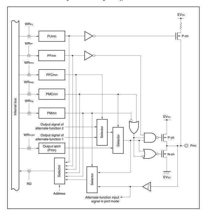
Figure 4-15. Block Diagram of Type E00-SUFT
