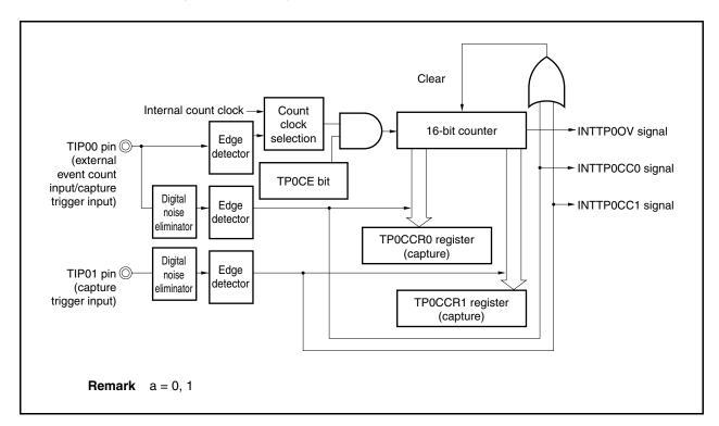
Figure 7-34. Configuration in Pulse Width Measurement Mode
