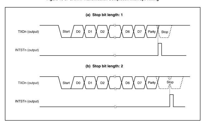
Figure 16-5. UARTn Transmission Completion Interrupt Timing
