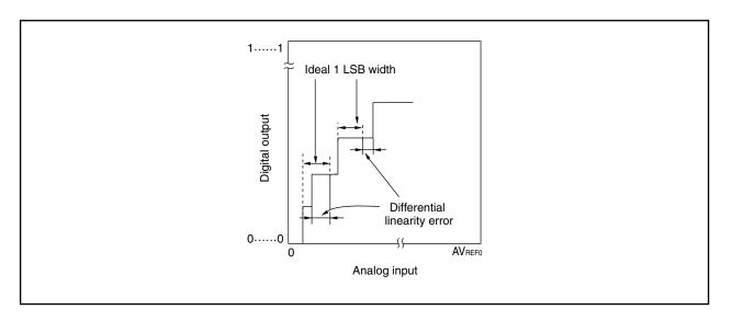
Figure 14-16. Differential Linearity Error
