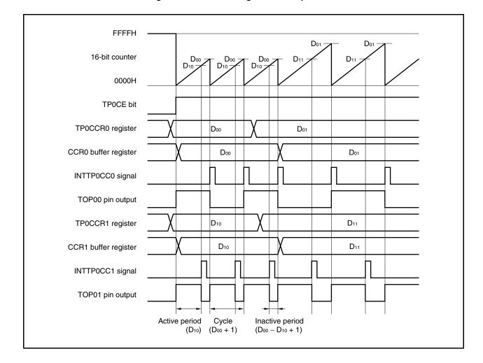
Figure 7-25. Basic Timing in PWM Output Mode
