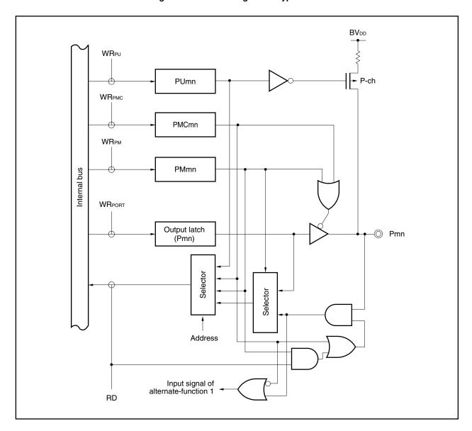
Figure 4-11. Block Diagram of Type D1-UH
