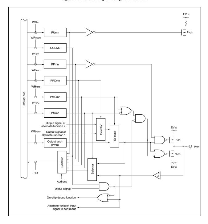
Figure 4-34. Block Diagram of Type OE001-SUFT
