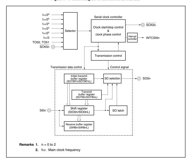
Figure 17-1. Block Diagram of Clocked Serial Interface
