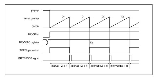
When the TP0CE bit is set to 1, the value of the 16-bit counter is cleared from FFFFH to 0000H in synchronization with the count clock, and the counter starts counting. At this time, the output of the TOP00 pin is inverted. Additionally, the set value of the TP0CCR0 register is transferred to the CCR0 buffer register.
