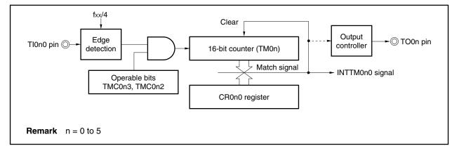
Figure 8-10. Block Diagram of External Event Counter Operation
