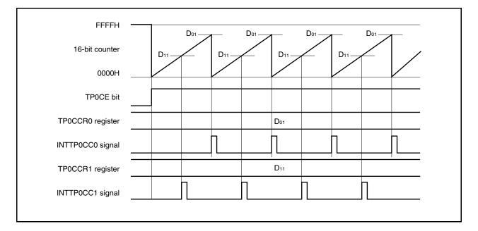
Figure 7-14. Timing Chart When D<sub>01</sub> ≥ D<sub>11</sub>
