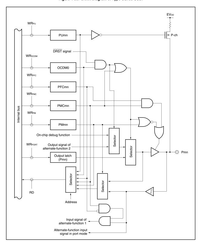
Figure 4-36. Block Diagram of Type OE100-SULT
