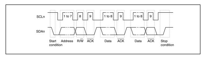
Figure 19-5. I<sup>2</sup>C Bus's Serial Data Transfer Timing
