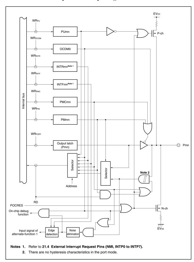
Figure 4-33. Block Diagram of Type OD11-SUIL
