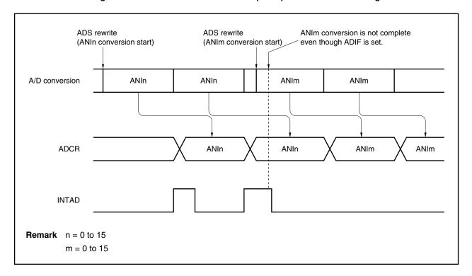
Figure 14-9. A/D Conversion End Interrupt Request Occurrence Timing
