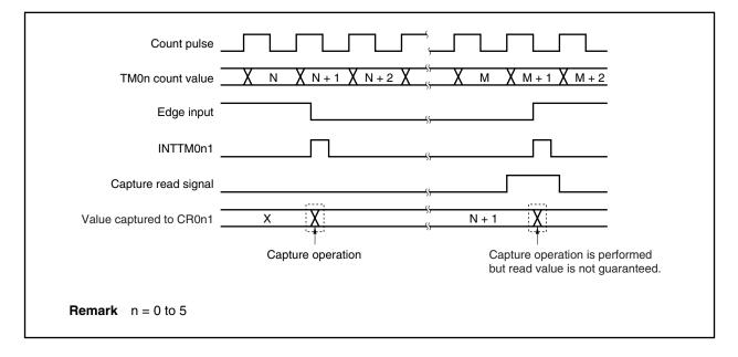
Figure 8-47. Data Hold Timing of Capture Register
