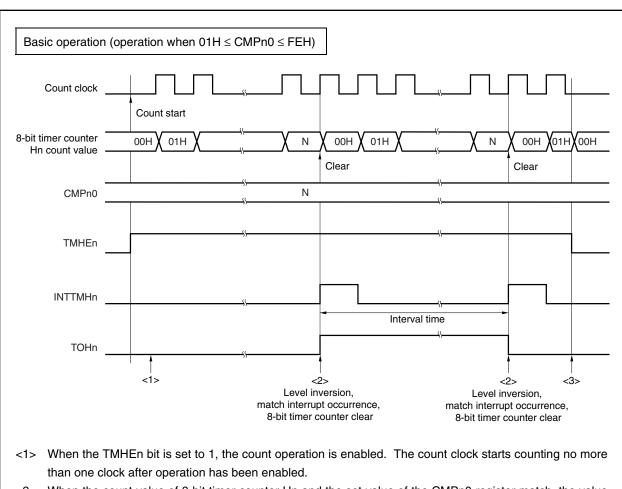
Figure 10-3. Timing of Interval Timer/Square Wave Output Operation (1/2)
