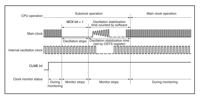
Figure 25-3. Operation When Main Clock Is Stopped (Arbitrary)
