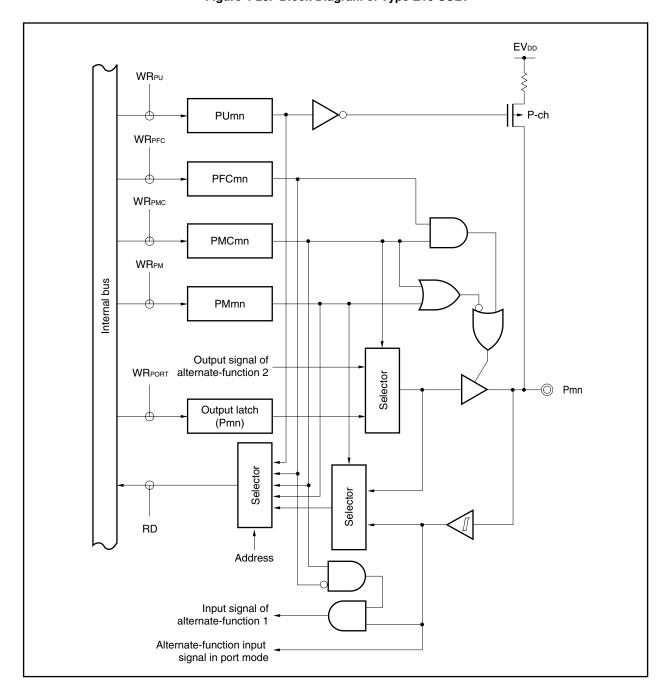
Figure 4-28. Block Diagram of Type E10-SULT
