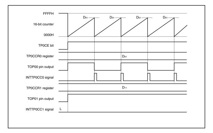
Figure 7-8. Timing Chart When D<sub>01</sub> < D<sub>11</sub>
