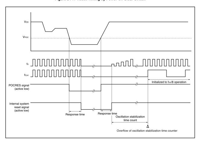
Figure 24-7. Reset Timing by Power-on-Clear Circuit
