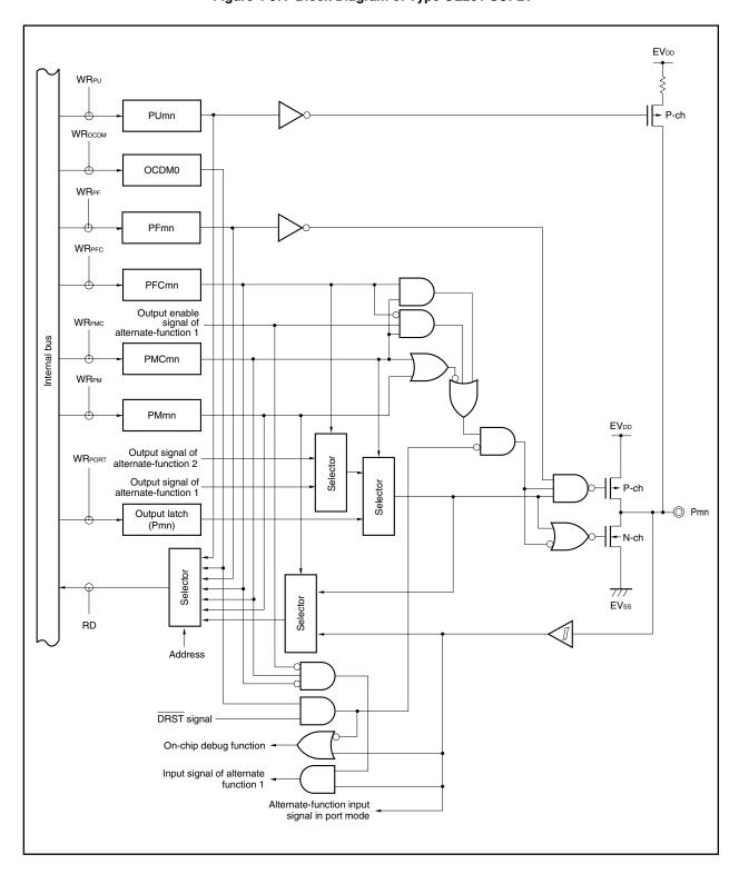
Figure 4-37. Block Diagram of Type OE201-SUFLT
