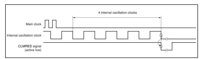
Figure 25-1. When Oscillation of Main Clock Is Stopped
