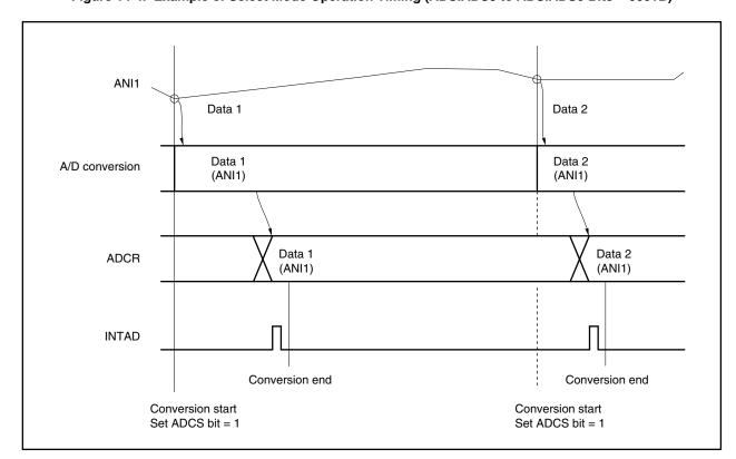
Figure 14-4. Example of Select Mode Operation Timing (ADS.ADS3 to ADS.ADS0 Bits = 0001B)
