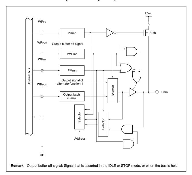
Figure 4-8. Block Diagram of Type D0-UZ
