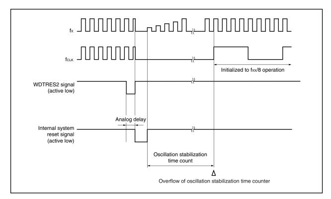
Figure 24-6. Timing of Reset Operation by Watchdog Timer 2
