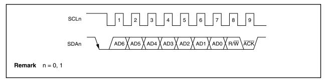
When the local address is received,  $\overline{ACK}$  is automatically generated regardless of the value of the ACKEn bit. No  $\overline{ACK}$  is generated if the received address is not a local address (NACK).
