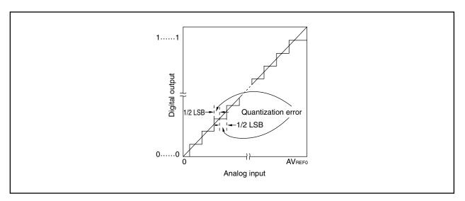
Figure 14-13. Quantization Error
