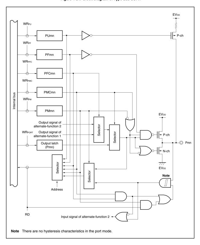
Figure 4-24. Block Diagram of Type E02-SUFH
