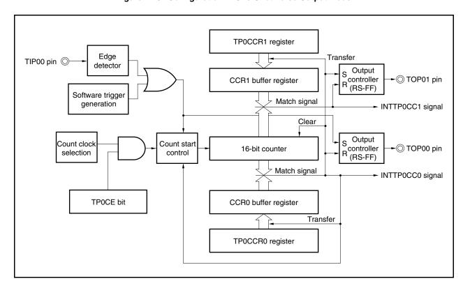
Figure 7-20. Configuration in One-Shot Pulse Output Mode
