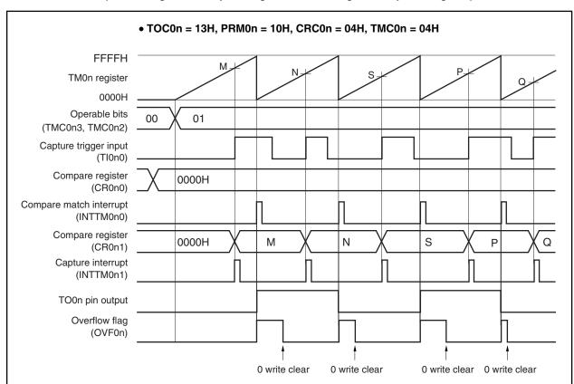
Figure 8-26. Timing Example of Free-Running Timer Mode (CR0n0 Register: Compare Register, CR0n1 Register: Capture Register)
