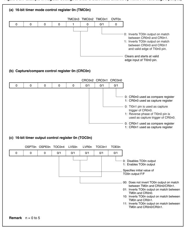
Figure 8-21. Example of Register Settings in Clear & Start Mode Entered by Tl0n0 Pin Valid Edge Input (2/2)
