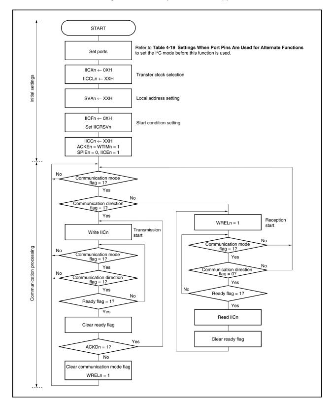
Figure 19-19. Slave Operation Flowchart (1)
