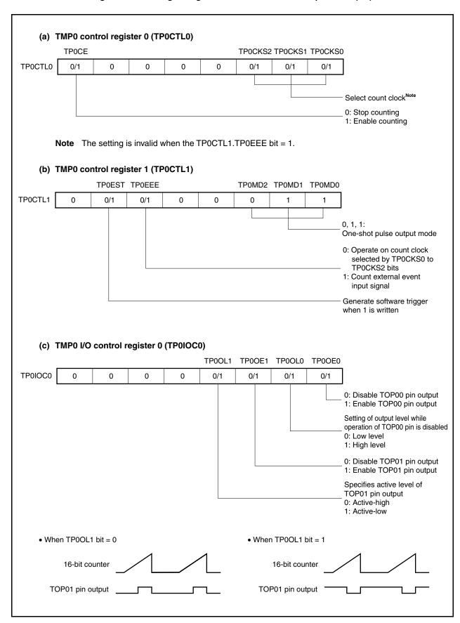
Figure 7-22. Setting of Registers in One-Shot Pulse Output Mode (2/2)
