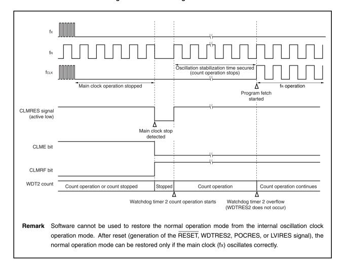
Figure 25-4. Reset Timing of Clock Monitor
