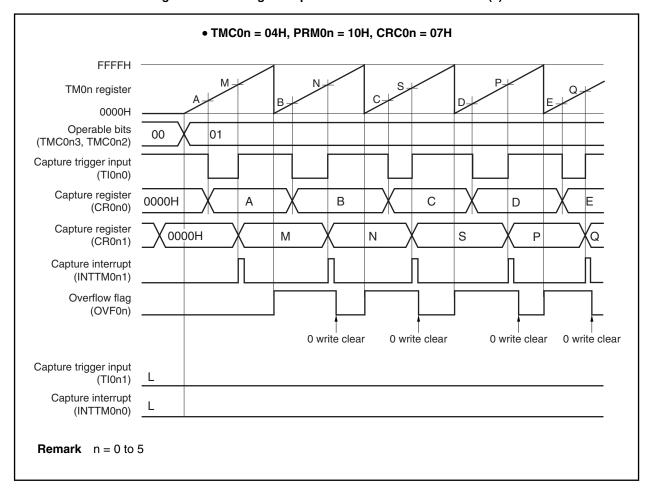
Figure 8-40. Timing Example of Pulse Width Measurement (2)
