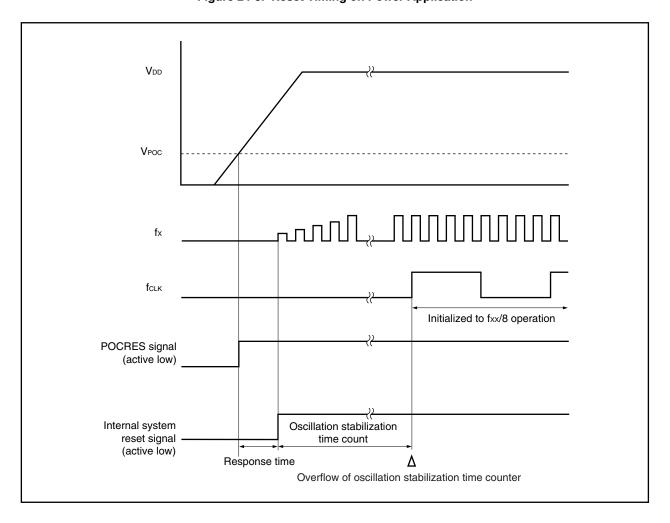
Figure 24-8. Reset Timing on Power Application
