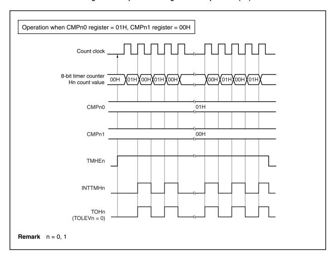
Figure 10-5. Operation Timing in PWM Output Mode (3/4)
