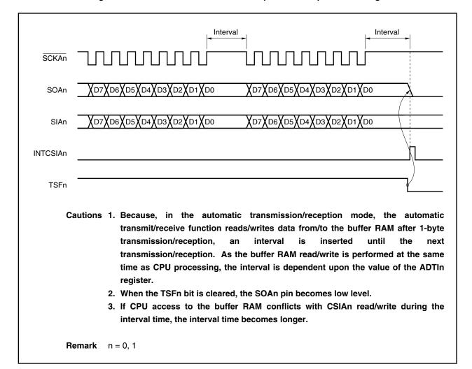
Figure 18-5. Automatic Transmission/Reception Mode Operation Timings
