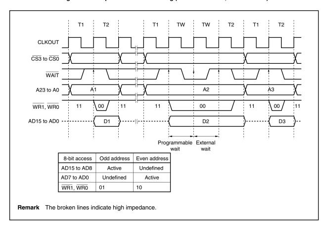
Figure 5-11. Separate Bus Write Timing (Bus Size: 16 Bits, 16-bit Access)
