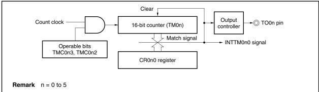
Figure 8-6. Block Diagram of Square Wave Output Operation
