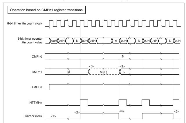
Figure 10-8. Carrier Generator Mode (3/3)
