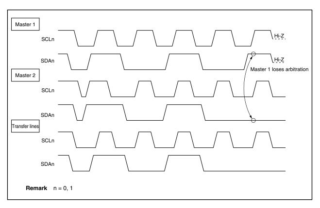
Figure 19-12. Arbitration Timing Example
