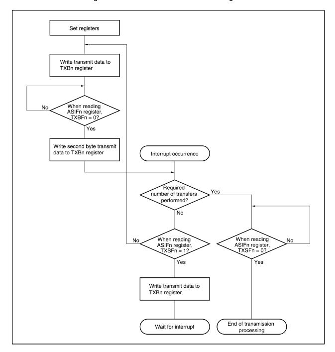
Figure 16-6. Continuous Transmission Processing Flow
