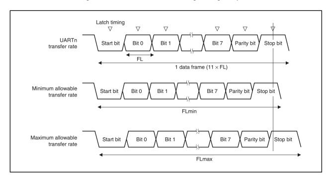
Figure 16-19. Allowable Baud Rate Range During Reception
