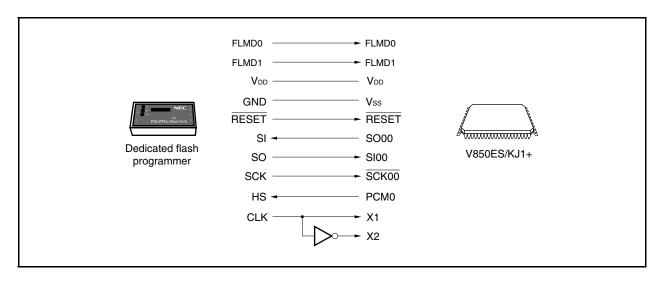
The dedicated flash programmer outputs the transfer clock, and the V850ES/KJ1+ operates as a slave.
