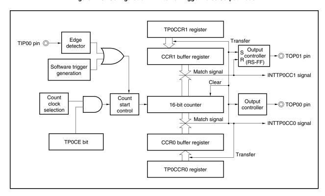
Figure 7-16. Configuration in External Trigger Pulse Output Mode
