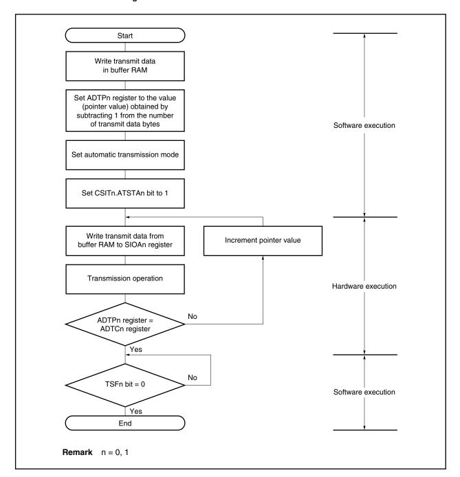
Figure 18-9. Automatic Transmission Mode Flowchart
