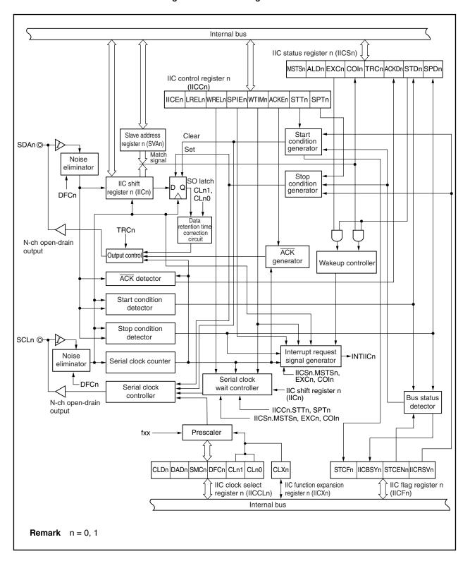
Figure 19-2. Block Diagram of I<sup>2</sup>Cn
