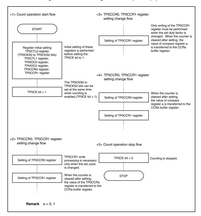
Figure 7-27. Software Processing Flow in PWM Output Mode (2/2)
