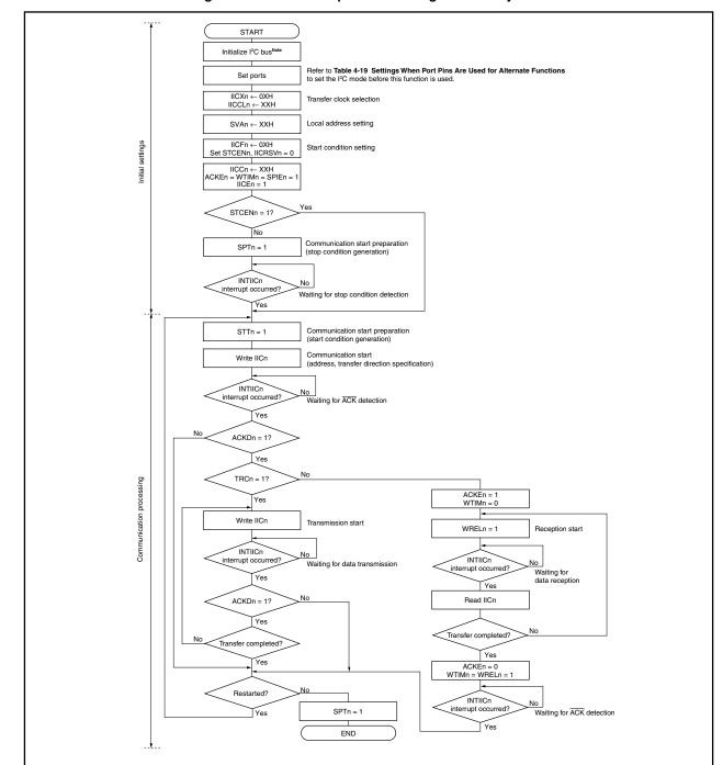
Figure 19-16. Master Operation in Single Master System
