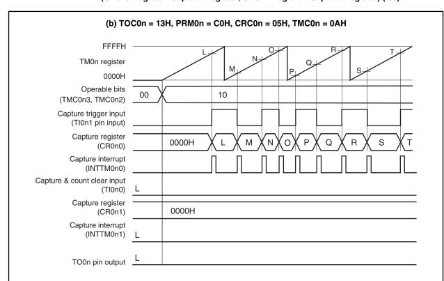
Figure 8-20. Timing Example of Clear & Start Mode Entered by Tl0n0 Pin Valid Edge Input (CR0n0 Register: Capture Register, CR0n1 Register: Capture Register) (2/3)
