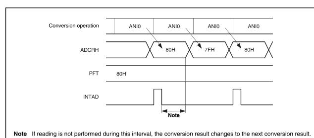
Figure 14-6. Power Fail Detection Function (PFCM Bit = 0)
