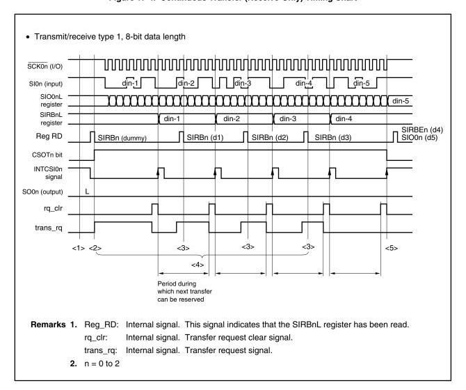
Figure 17-4. Continuous Transfer (Receive-Only) Timing Chart
