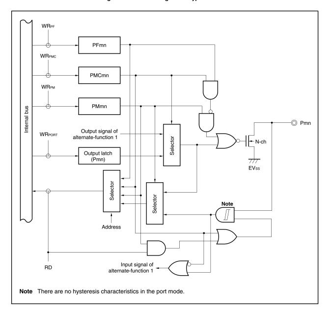
Figure 4-12. Block Diagram of Type D2-SNFH
