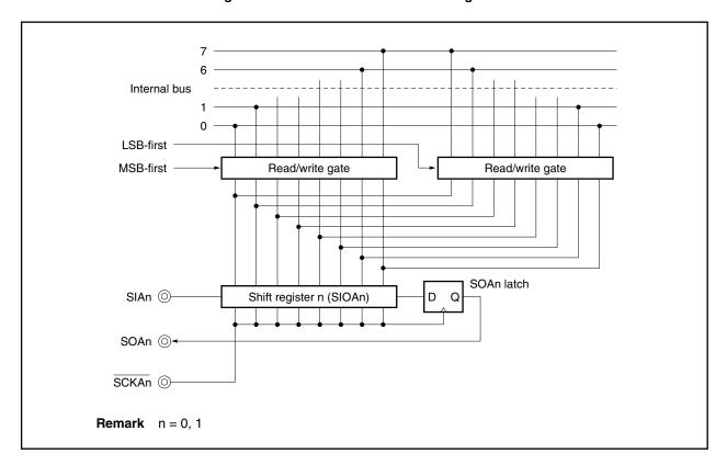
Figure 18-4. Transfer Bit Order Switching Circuit
