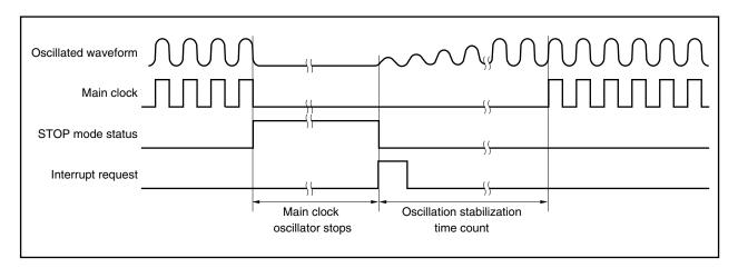
Figure 23-2. Oscillation Stabilization Time
