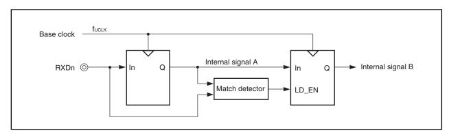
Figure 16-12. Noise Filter Circuit
