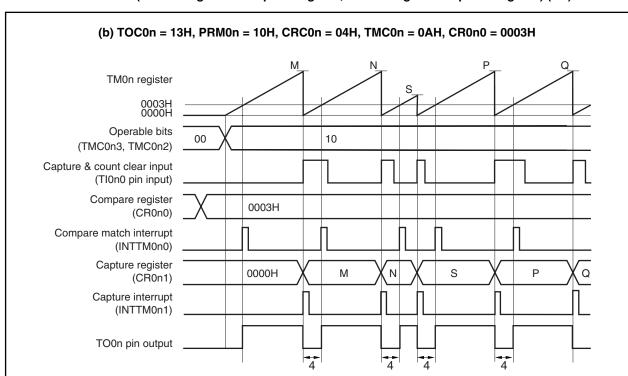
Figure 8-16. Timing Example of Clear & Start Mode Entered by Tl0n0 Pin Valid Edge Input (CR0n0 Register: Compare Register, CR0n1 Register: Capture Register) (2/2)
