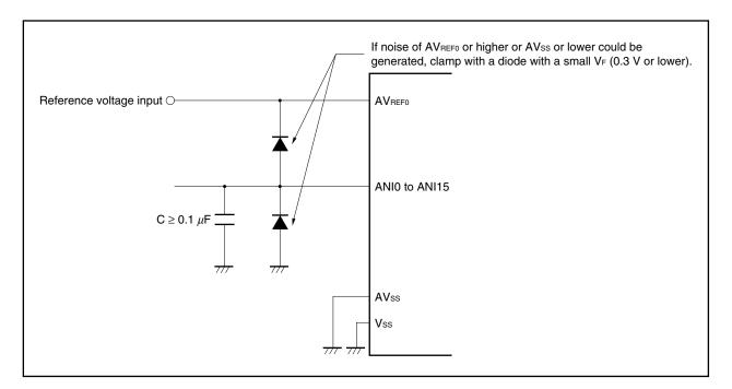
Figure 14-8. Handling of Analog Input Pins
