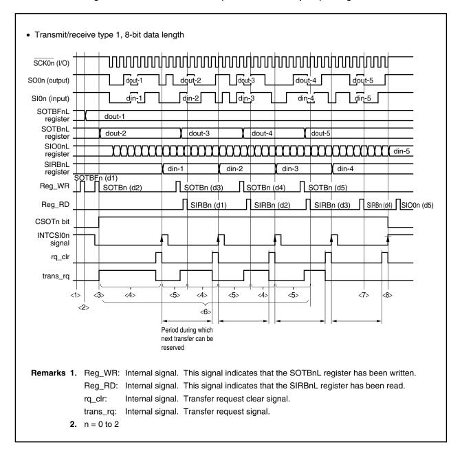
Figure 17-5. Continuous Transfer (Transmission/Reception) Timing Chart
