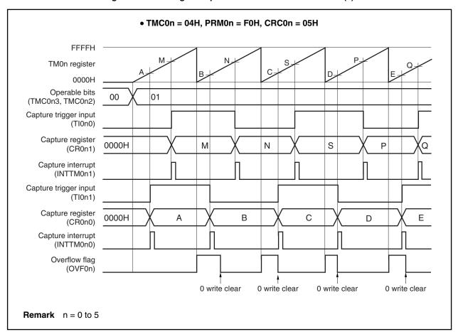
Figure 8-39. Timing Example of Pulse Width Measurement (1)
