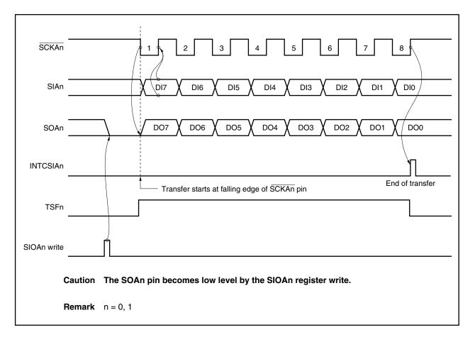
Figure 18-2. 3-Wire Serial I/O Mode Timing
