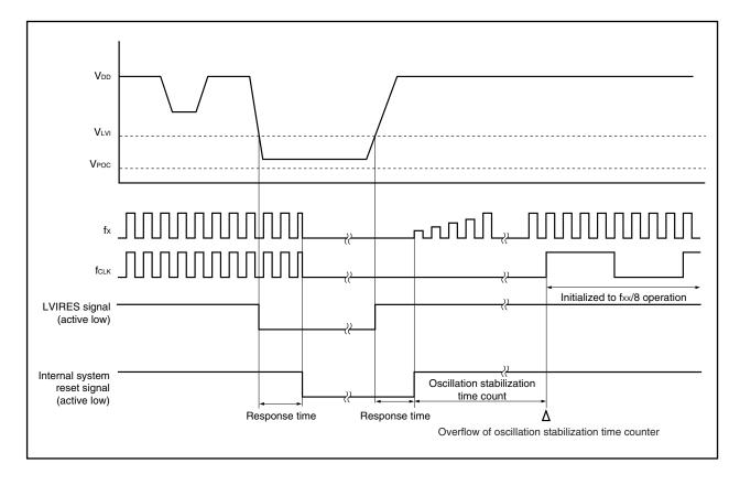
Figure 24-9. Reset Timing by Low-Voltage Detector
