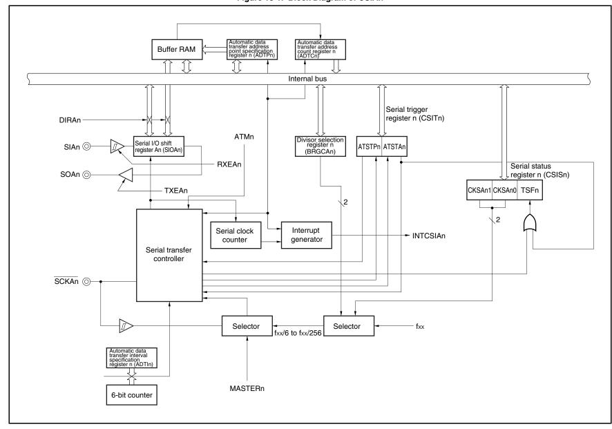
Figure 18-1. Block Diagram of CSIAn
