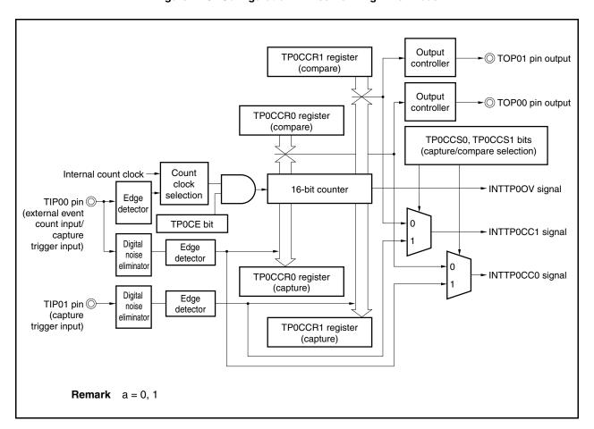
Figure 7-28. Configuration in Free-Running Timer Mode
