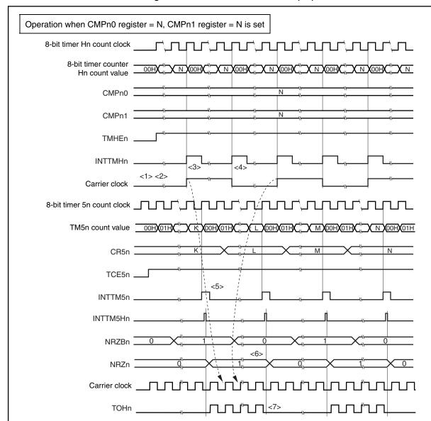
Figure 10-8. Carrier Generator Mode (1/3)
