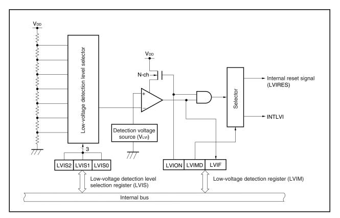
Figure 26-1. Block Diagram of Low-Voltage Detector
