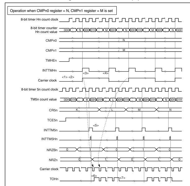
Figure 10-8. Carrier Generator Mode (2/3)
