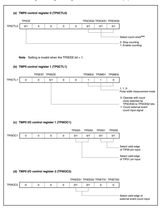
Figure 7-36. Register Setting in Pulse Width Measurement Mode (2/2)
