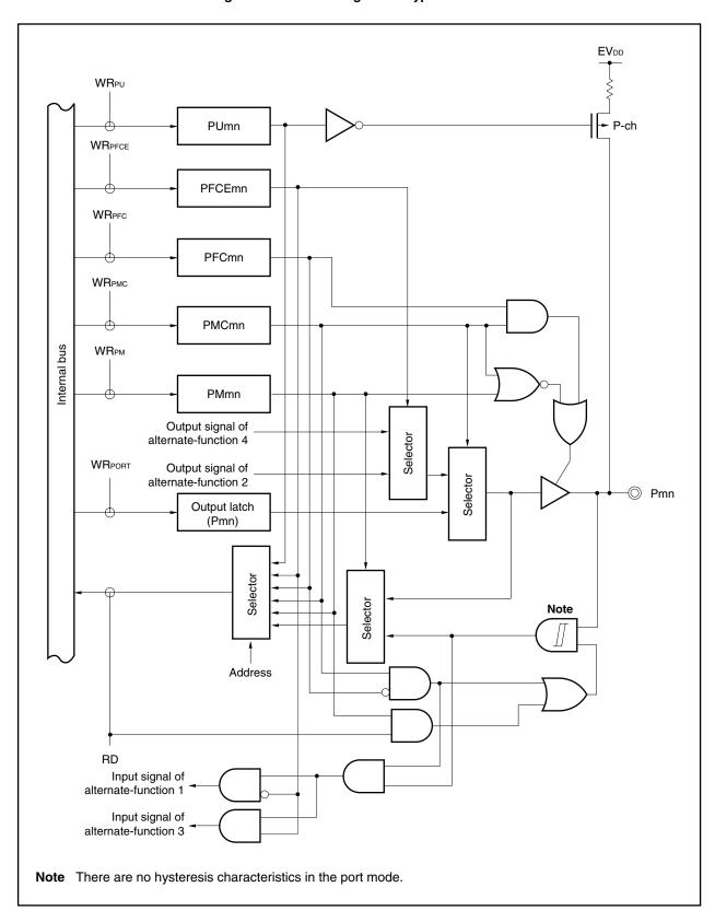
Figure 4-32. Block Diagram of Type G1010-SUL
