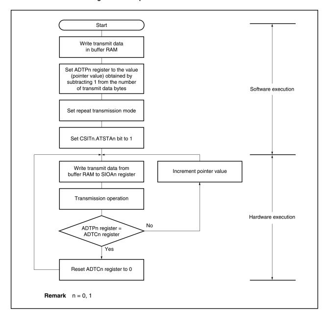
Figure 18-12. Repeat Transmission Mode Flowchart
