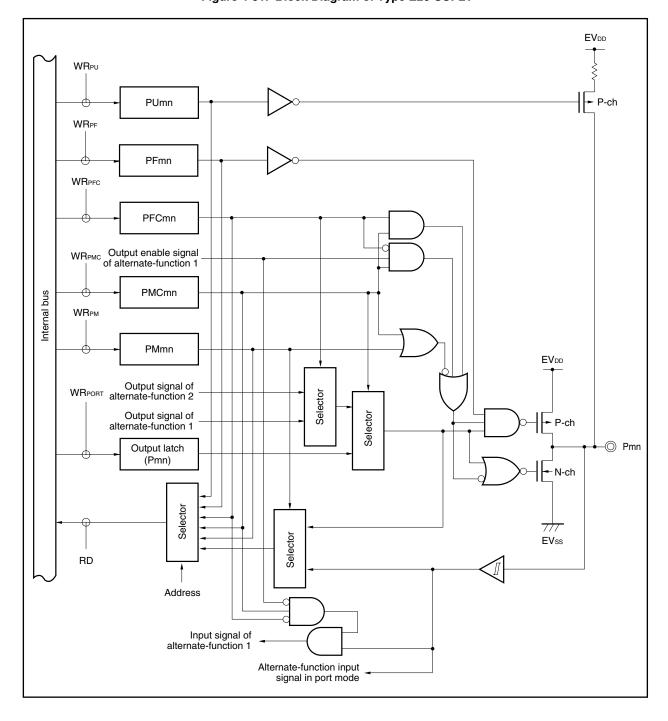
Figure 4-31. Block Diagram of Type E20-SUFLT
