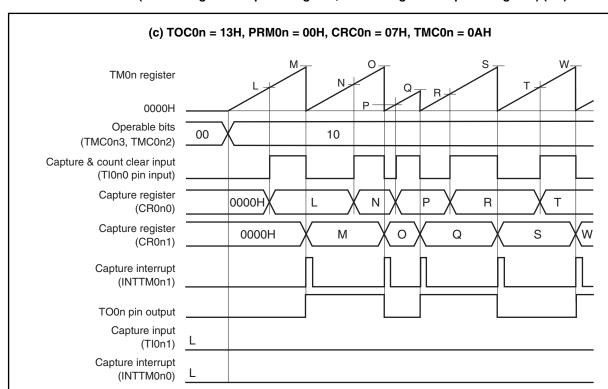
Figure 8-20. Timing Example of Clear & Start Mode Entered by Tl0n0 Pin Valid Edge Input (CR0n0 Register: Capture Register, CR0n1 Register: Capture Register) (3/3)
