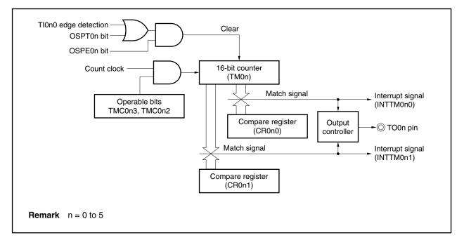
Figure 8-34. Block Diagram of One-Shot Pulse Output Operation
