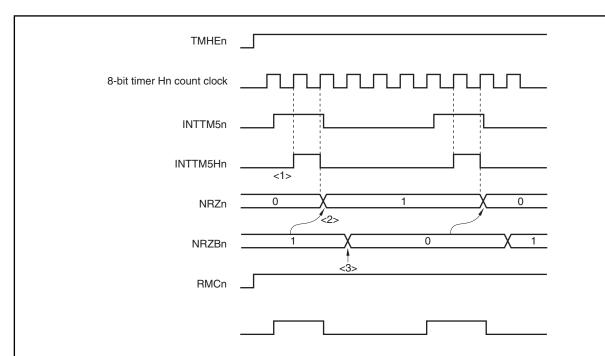
Figure 10-6. Transfer Timing
