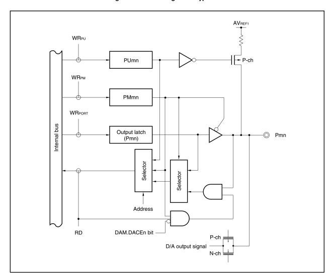
Figure 4-5. Block Diagram of Type C-UA
