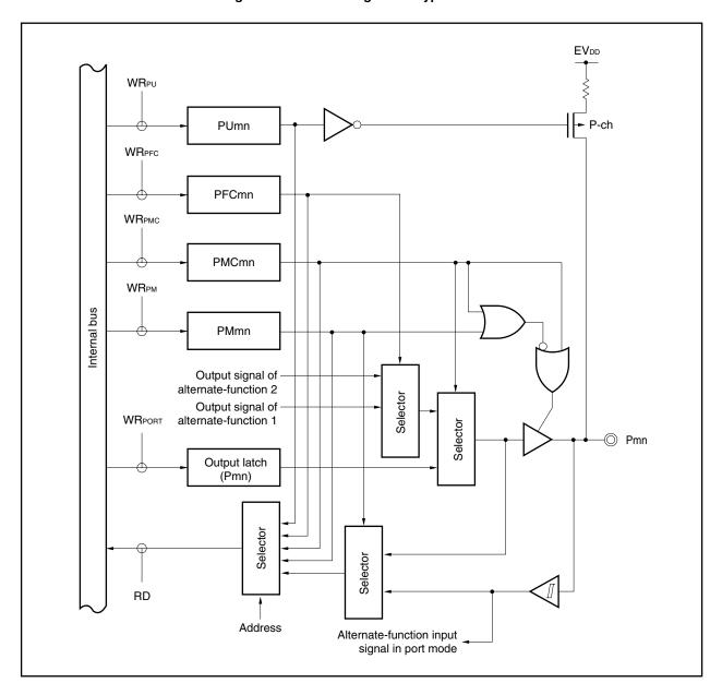
Figure 4-16. Block Diagram of Type E00-SUT
