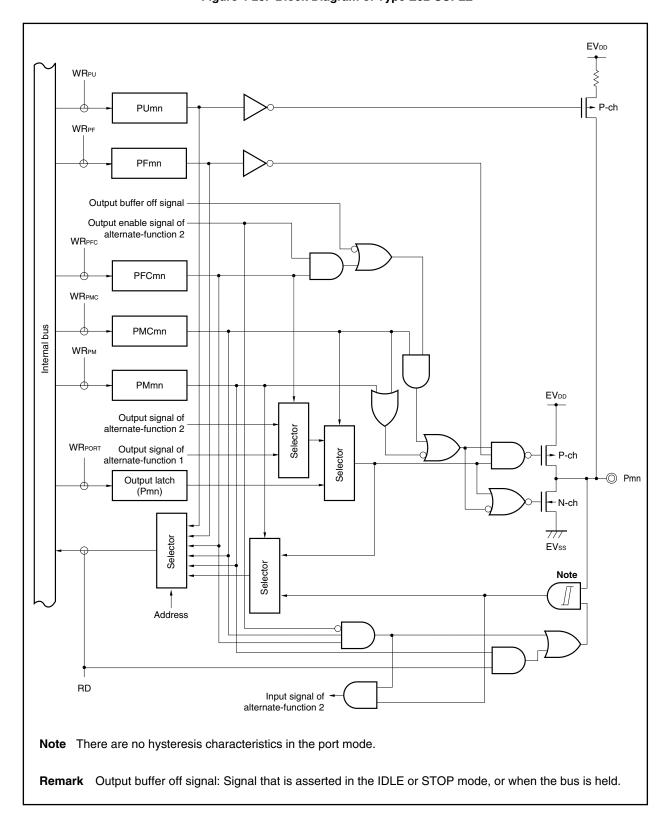
Figure 4-25. Block Diagram of Type E02-SUFLZ
