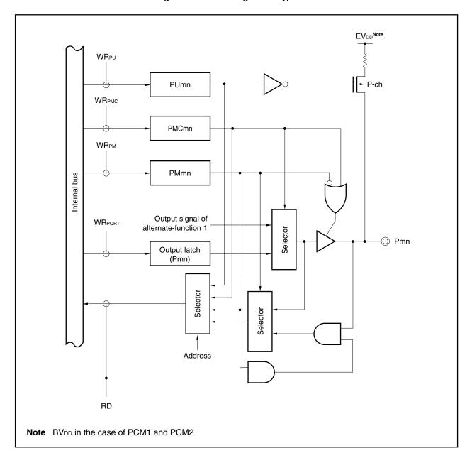
Figure 4-6. Block Diagram of Type D0-U
