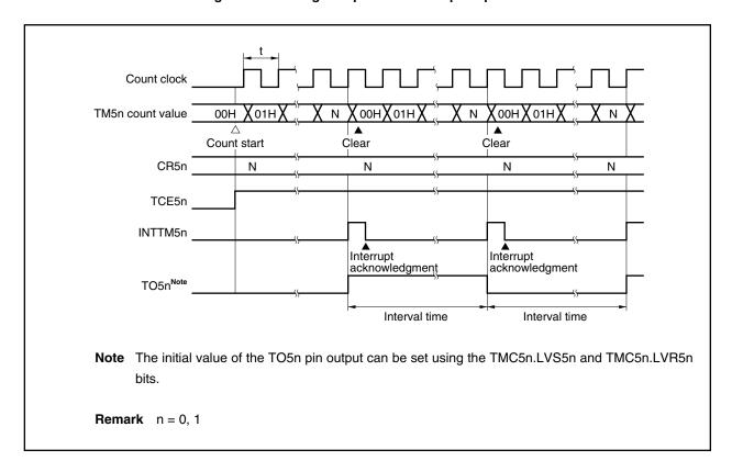
Figure 9-4. Timing of Square-Wave Output Operation
