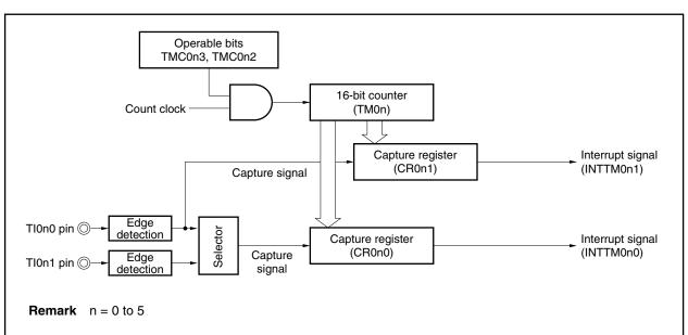
Figure 8-37. Block Diagram of Pulse Width Measurement (Free-Running Timer Mode)
