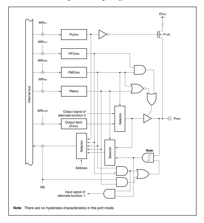
Figure 4-27. Block Diagram of Type E10-SUL
