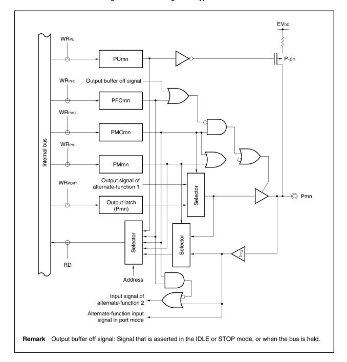
Figure 4-21. Block Diagram of Type E01-SUHTZ
