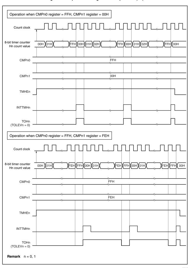
Figure 10-5. Operation Timing in PWM Output Mode (2/4)
