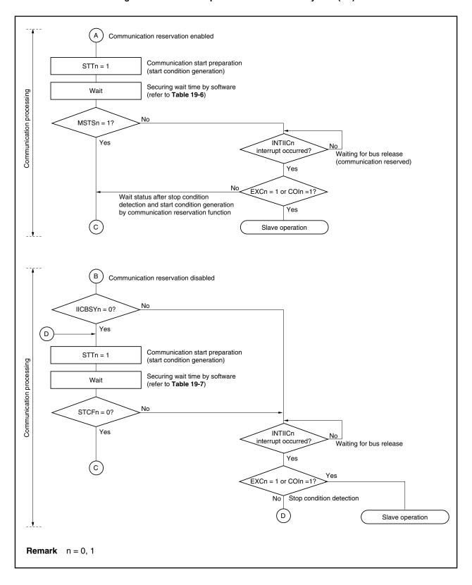
Figure 19-17. Master Operation in Multimaster System (2/3)
