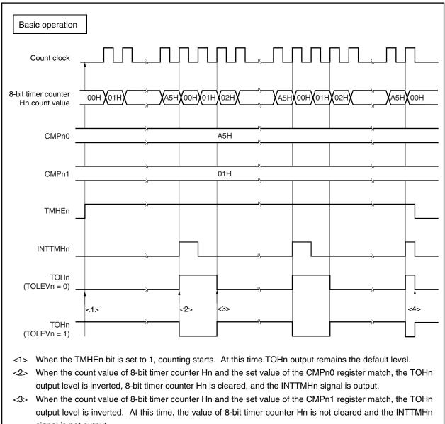
Figure 10-5. Operation Timing in PWM Output Mode (1/4)
