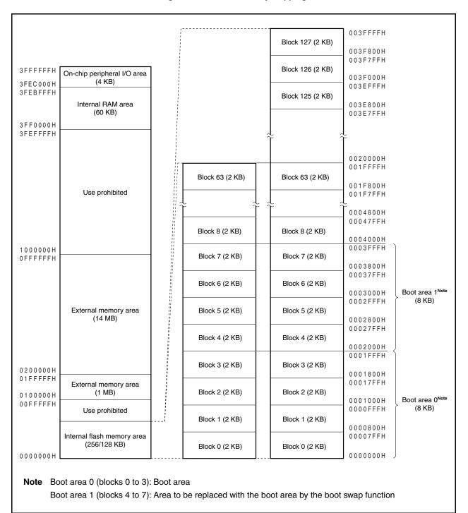
Figure 30-1. Flash Memory Mapping
