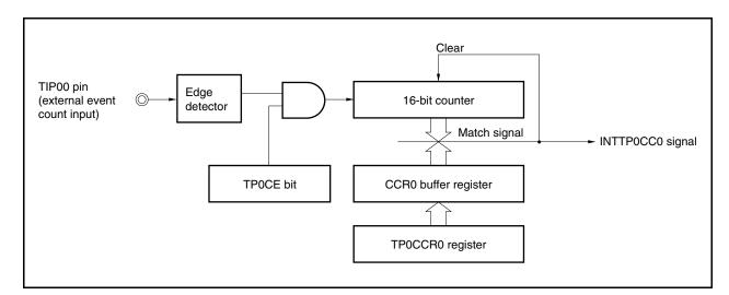
Figure 7-9. Configuration in External Event Count Mode
