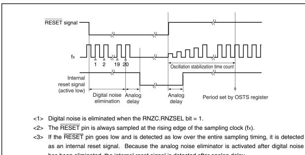
Figure 24-4. Sampling Operation Timing (20 Times)
