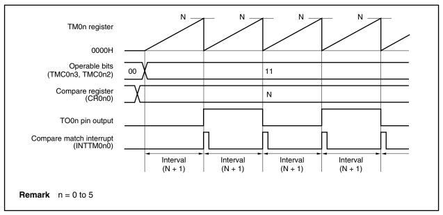
Figure 8-8. Example of Register Settings for Square Wave Output Operation
