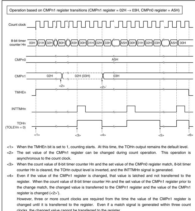
Figure 10-5. Operation Timing in PWM Output Mode (4/4)
