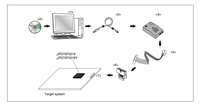
Figure A-3. Example of On-Chip Emulation System Configuration
