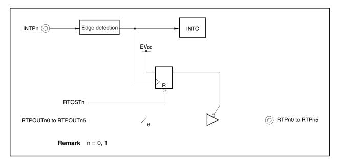
Figure 13-3. Block Diagram of Security Function
