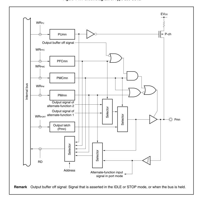
Figure 4-17. Block Diagram of Type E00-SUTZ
