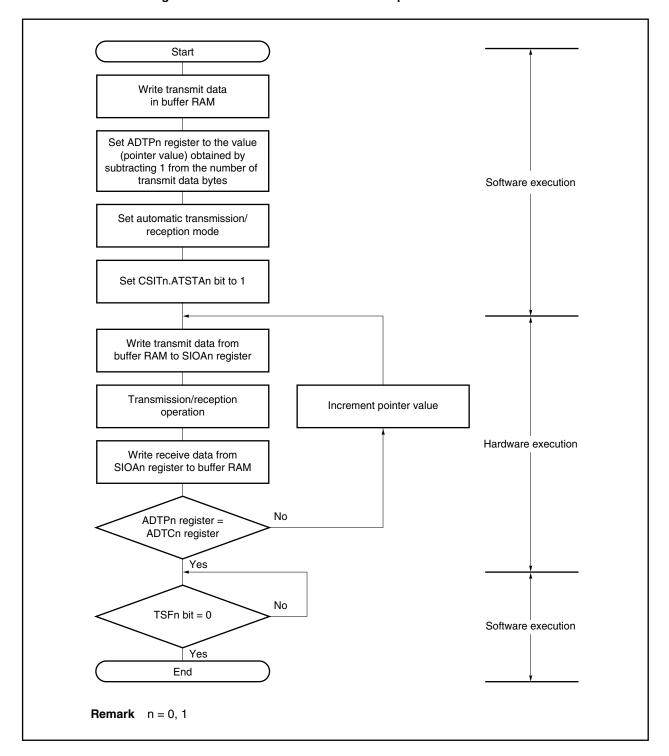
Figure 18-6. Automatic Transmission/Reception Mode Flowchart
