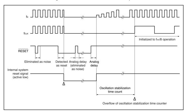
Figure 24-2. Hardware Status on RESET Pin Input
