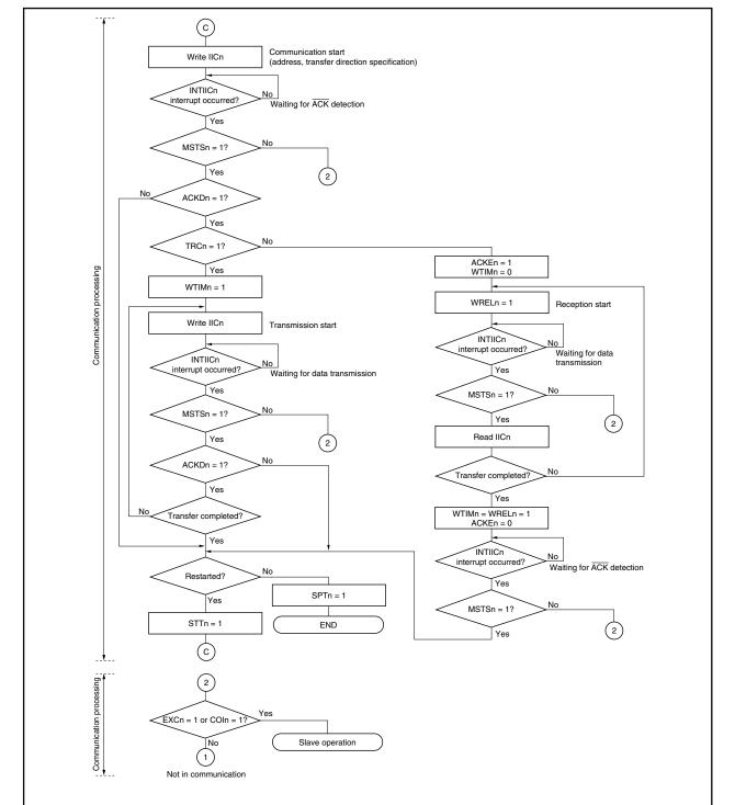
Figure 19-17. Master Operation in Multimaster System (3/3)
