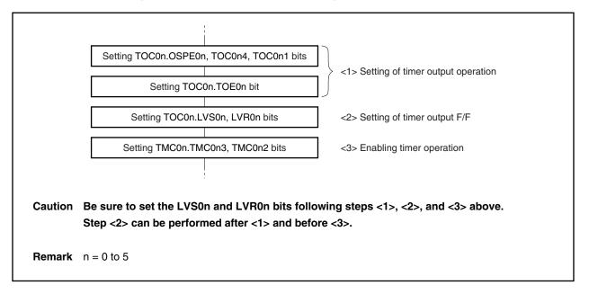
Figure 8-45. Timing Example of LVR0n and LVS0n Bits
