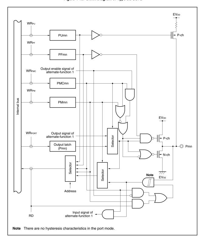
Figure 4-13. Block Diagram of Type D2-SUFL
