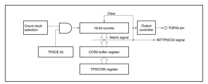
Figure 7-2. Configuration of Interval Timer
