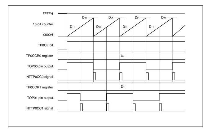
Figure 7-7. Timing Chart When D<sub>01</sub> ≥ D<sub>11</sub>
