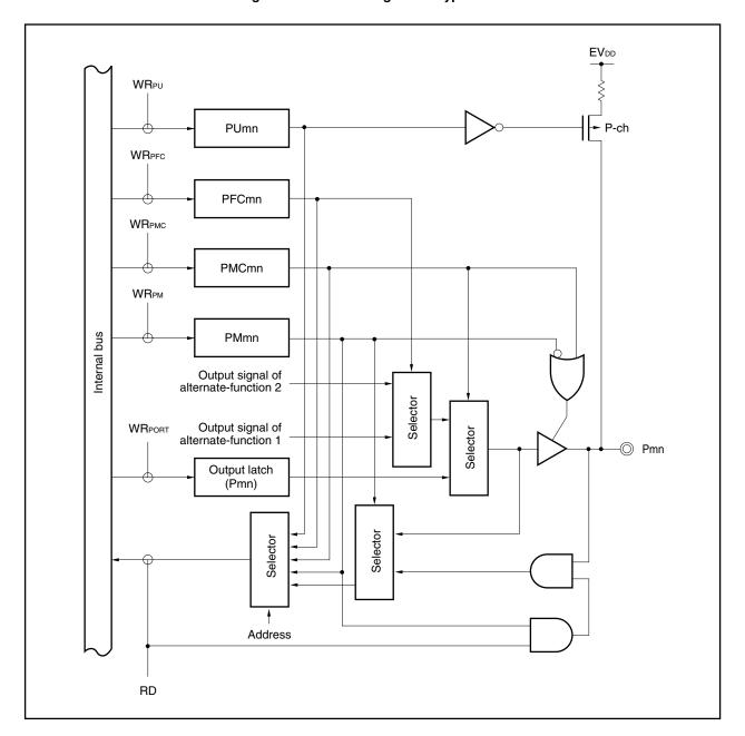
Figure 4-18. Block Diagram of Type E00-U
