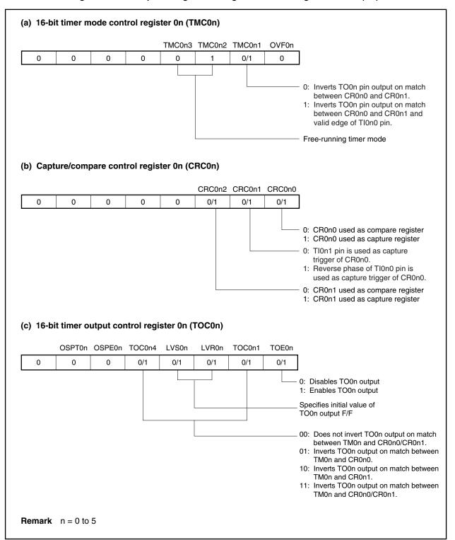
Figure 8-29. Example of Register Settings in Free-Running Timer Mode (2/2)
