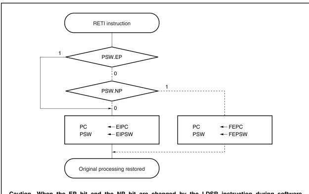
Caution When the EP bit and the NP bit are changed by the LDSR instruction during software exception processing, in order to restore the PC and PSW correctly during restoring by the RETI instruction, it is necessary to set the EP bit back to 1 using the LDSR instruction immediately before the RETI instruction.
