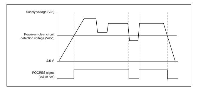
Figure 27-2. Operation of Power-on-Clear Circuit
