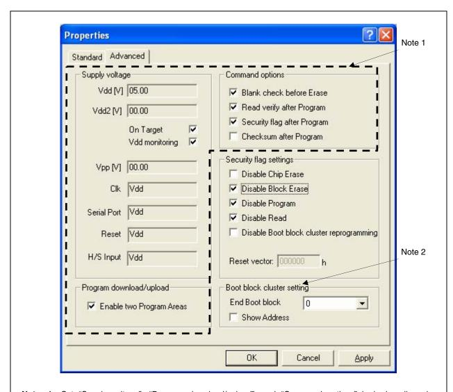
**Notes 1.** Set "Supply voltage", "Program download/upload", and "Command options" in broken lines in accordance with the use conditions.
