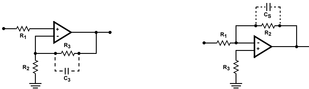
FIGURE 3. SUGGESTED OFFSET VOLTAGE ADJUSTMENT
