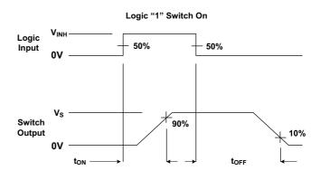
Figure 4. Switching Test Circuit Waveform
