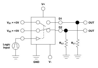
Figure 5. Break-Before-Make Test Circuit
