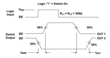
Figure 6. Break-Before-Make Test Circuit Waveforms
