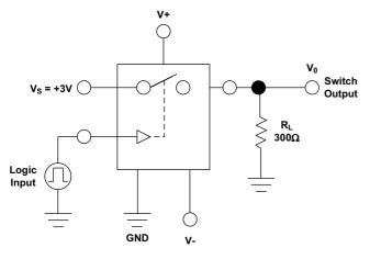
Figure 3. Switching Test Circuit
