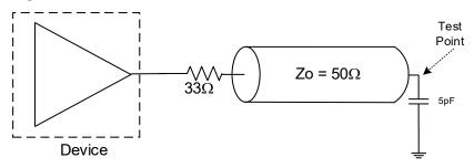
Figure 3. HCSL/LPHCSL Test Load
