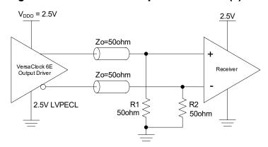
Figure 17. 2.5V LVPECL Output Termination (3)
