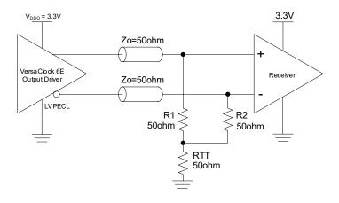
Figure 15. 2.5V LVPECL Output Termination (1)
