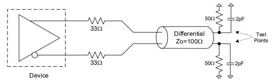
Figure 4. LVDS Test Load
