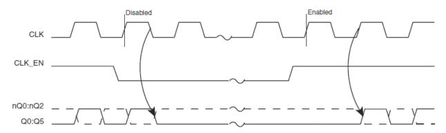
FIGURE 1. CLK\_EN TIMING DIAGRAM
