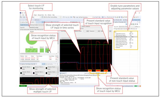
Figure 5 Monitoring and Parameter Adjustment
