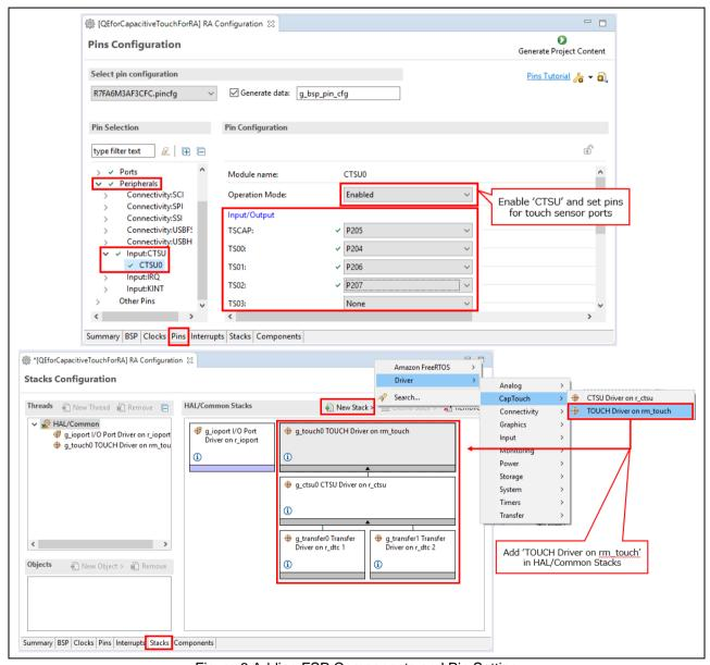
Figure 6 Adding FSP Components and Pin Setting
