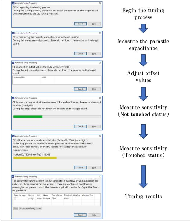
Figure 3 Initial Tuning Process
