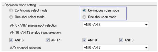
(2) The analog pin setting is three or fewer pins in [ANI0 - ANIn analog input selection] (n = 2 to 23).
