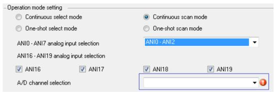
(3) The [Resolution setting], [Trigger mode setting], or [Conversion time setting] (parts framed by red rectangles below) is changed, while the pull-down menu of the above A/D channel selection has become empty and the icon (framed by a blue rectangle below) is displayed.
