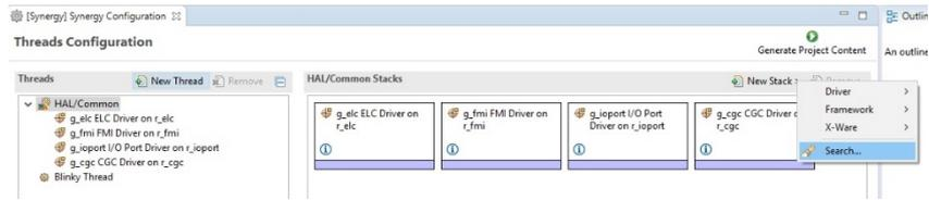
Clicking this menu item then opens a dialog allowing you to search and filter on the available SSP modules. In the example below, we have entered SPI and this is the result:
