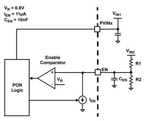
Figure 26. Enable Circuit
