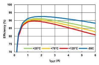
Figure 9. 3.3V V<sub>IN</sub> Efficiency, 1.2V V<sub>OUT</sub> Over Temperature
