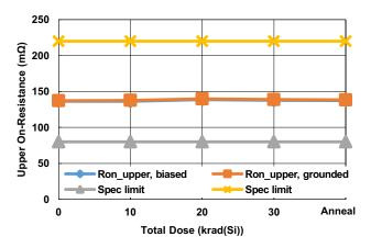
Figure 35. Upper  $r_{DS(ON)}$  vs TID
