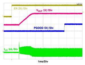
Figure 14. 0.5V Prebiased Start-Up to 2.5V  $V_{OUT}$  Waveforms  $I_{O} = 0A$
