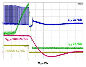
**Figure 18. Into Overcurrent Waveforms**
