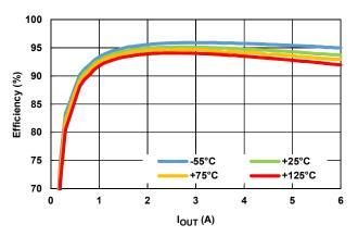
Figure 8. 5V  $V_{IN}$  Efficiency, 3.3V  $V_{OUT}$  Over Temperature
