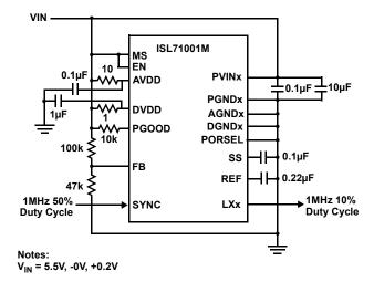
Figure 30. Irradiation Bias Configuration for the IS71001M
