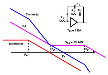
Figure 28. Feedback Loop Compensation
