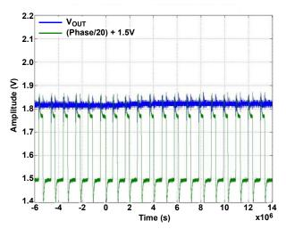
Figure 36. Set Response with 5.5V Input, ∆V<sub>OUT</sub> <1%
