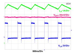
Figure 11. LX,  $V_{OUT}$  and Inductor Current Waveforms,  $I_{O}$  = 6A
