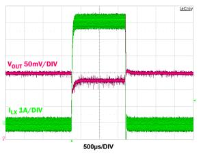
Figure 17. Load Transient 0 to 6A
