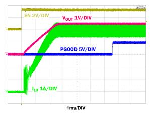
Figure 16. Start-Up to 2.5V  $V_{OUT}$  Waveforms  $I_O$  = 5A
