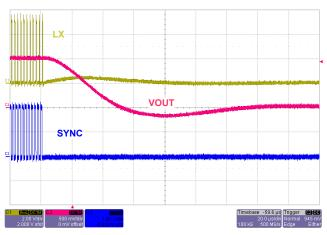
Figure 25. SYNC Loss Showing LX Pulled Low
