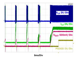
Figure 19. Out of Overcurrent Recovery Waveforms
