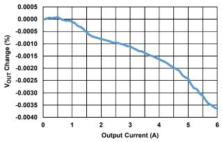
Figure 21.  $V_{IN}$  Line Regulation,  $V_{OUT} = 2.5V (5V_{IN} - 3.3V_{IN})$
