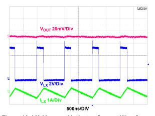
Figure 10. LX,  $V_{OUT}$  and Inductor Current Waveforms,  $I_{O}$  = 0A
