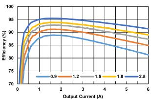
Figure 7. 3.3V  $V_{IN}$  Efficiency for Multiple  $V_{OUT}$  Levels
