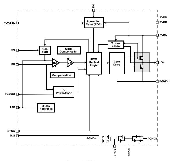
Figure 5. Block Diagram
