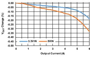
Figure 20. V<sub>IN</sub> Load Regulation 1.2V V<sub>OUT</sub>
