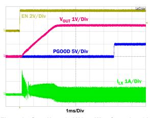
Figure 15. Start-Up to 2.5V  $V_{OUT}$  Waveforms  $I_{O}$  = 0A
