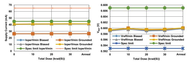
Figure 31. Operating Supply Current vs TID
