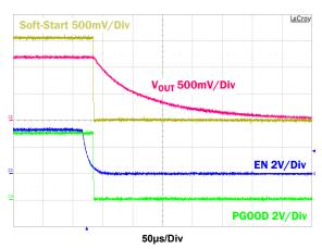
Figure 13. Disabled Turn-Off Waveforms
