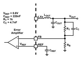
Figure 24. Output Voltage Selection
