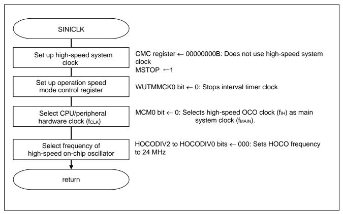
Figure 5.5 Clock Generation Circuit Setup
