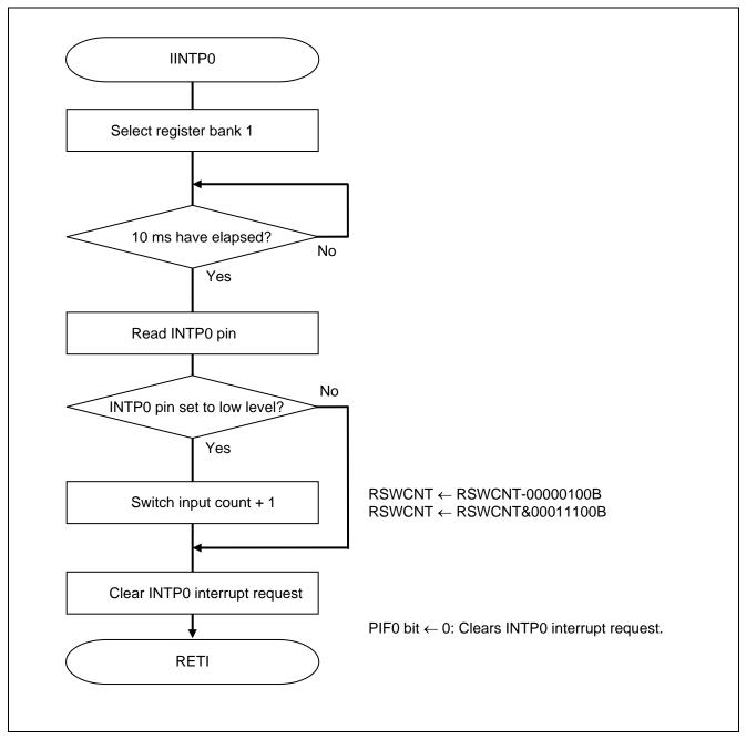
Figure 5.8 INTP0 Interrupt Processing
