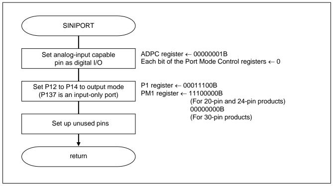
Figure 5.4 I/O Port Setup
