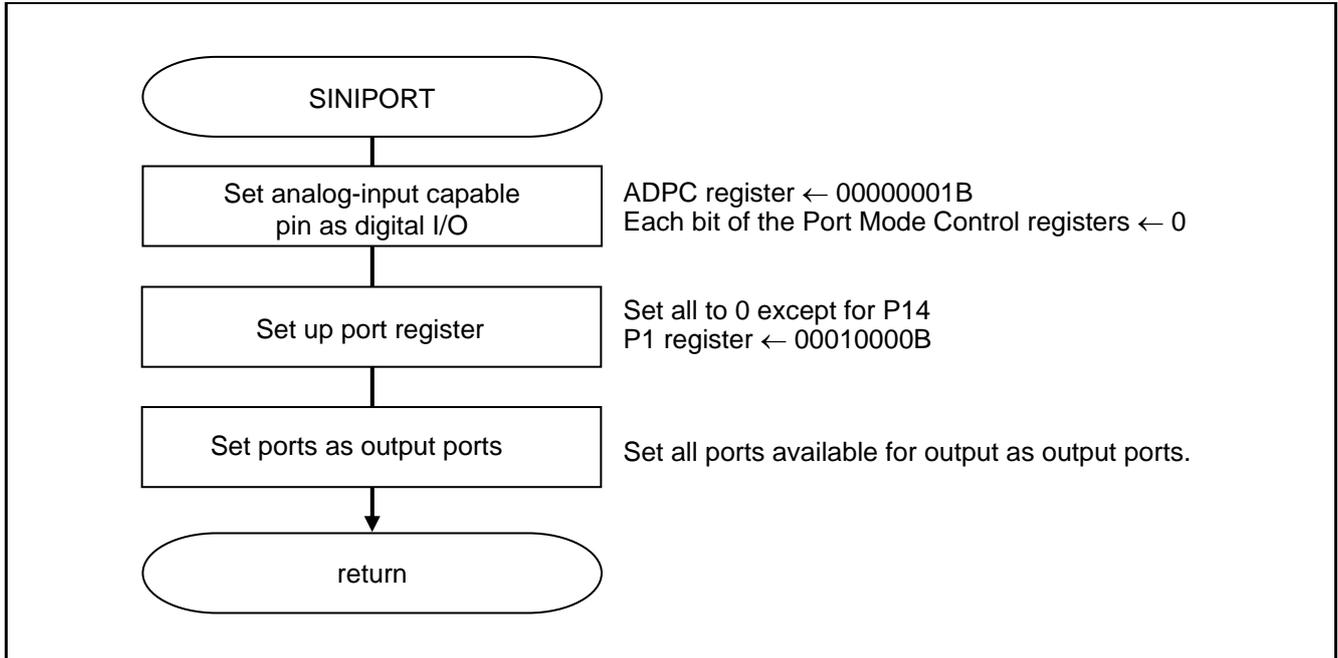
Figure 5.3 I/O Port Setup
