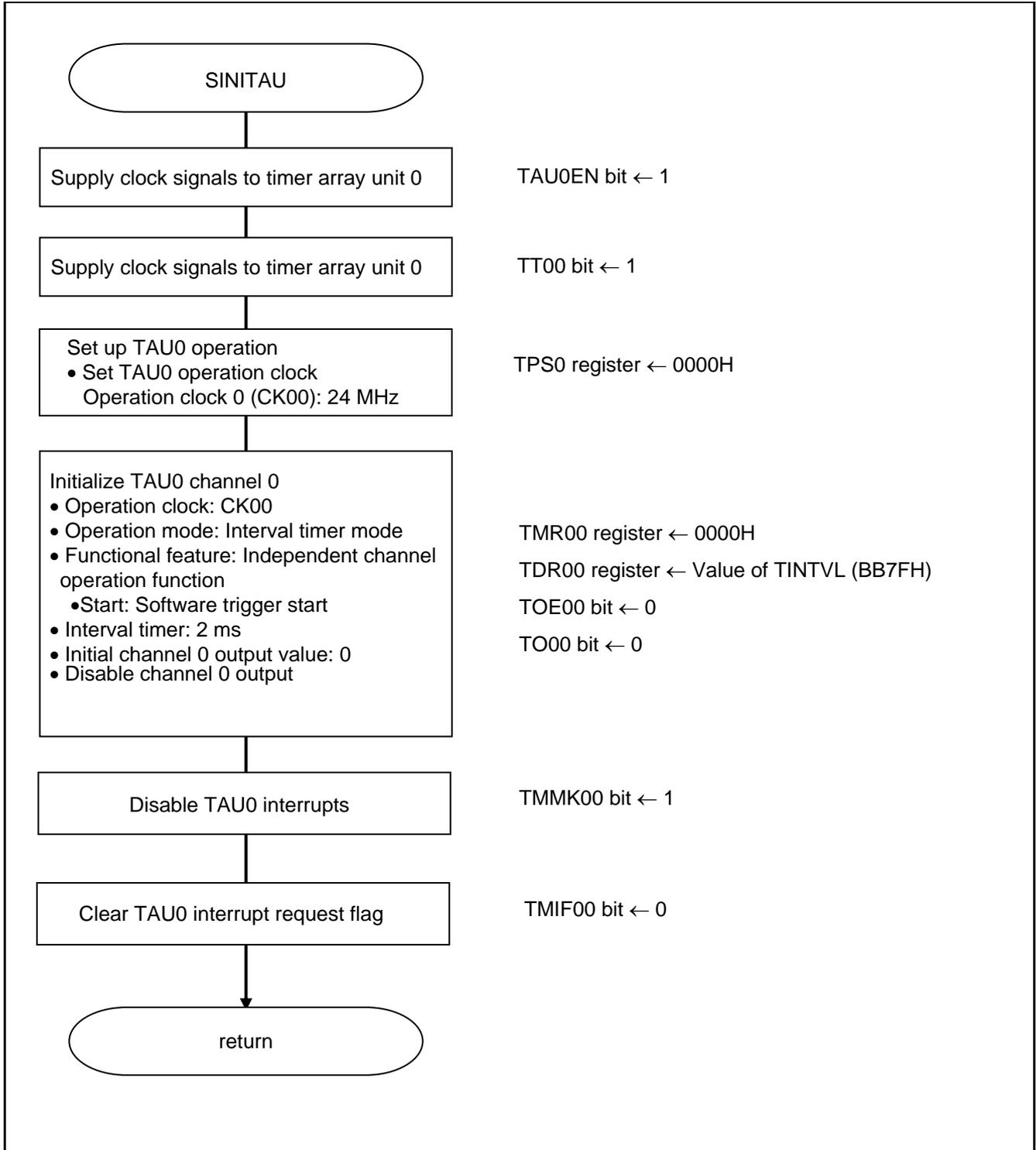
Figure 5.5 Timer Array Unit Setup
