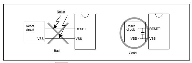
Figure 1.1 Wiring for the RESET Pin
