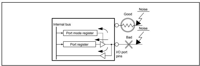
Figure 1.7 Setup for I/O Ports
