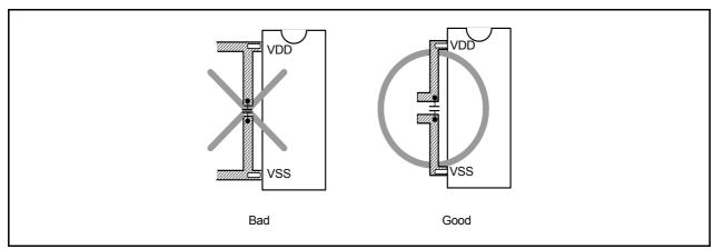
Figure 1.3 Bypass Capacitor Across the Vss Line and VDD Line
