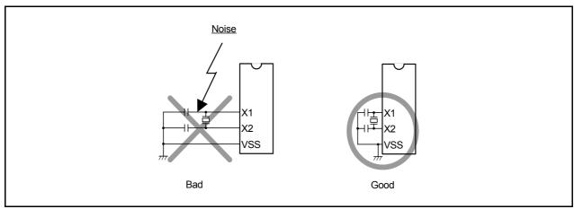
Figure 1.2 Wiring for Clock Input/Output Pins
