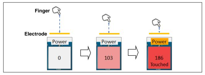
Figure 3.1 Button detection display
