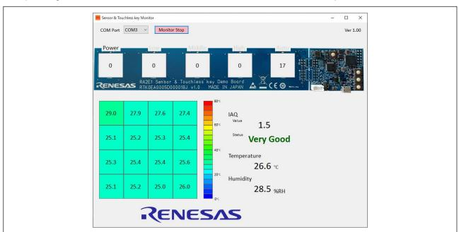
After pressing "Monitor Start", it will show measurements of each sensor and capacitive touch electrode.
