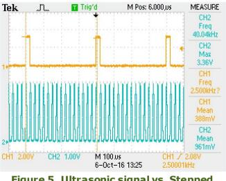
Figure 5. Ultrasonic signal vs. Stepped down Frequency
