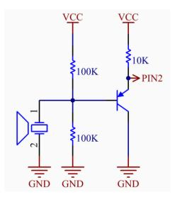
Figure 19. Ultrasonic detection
