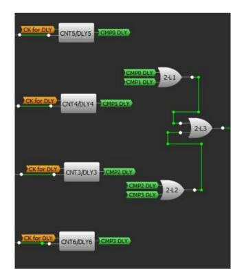
Figure 12. Delay devices-OR network
