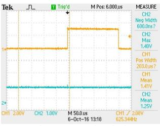
Figure 17. Pin6>1200 mV (CH2) Dly=0.200 ms (CH1)
