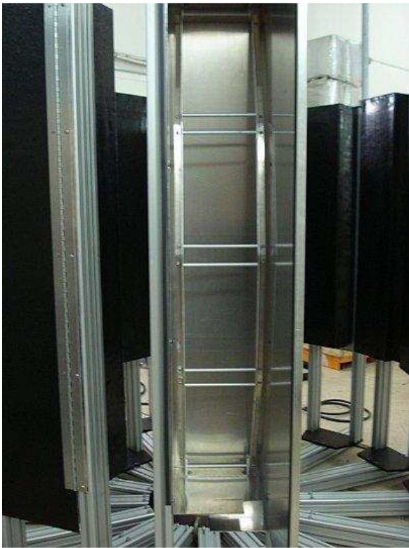
Fig. 8: Internal view of a PbAl box and enclosed DUT board rack. The curvature of the test rack can be clearly seen; this curvature combines with the circular arrangement of the racks to generate an approximately spherical isodose profile at the DUT boards.
