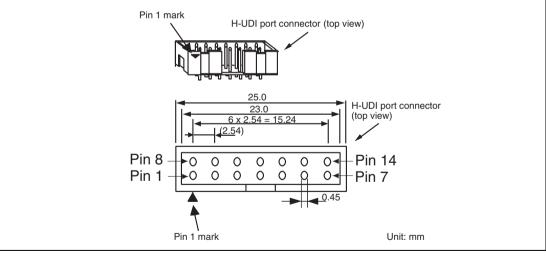
Figure 1.1 Pin Assignments of the H-UDI Port Connector (14 Pins)
