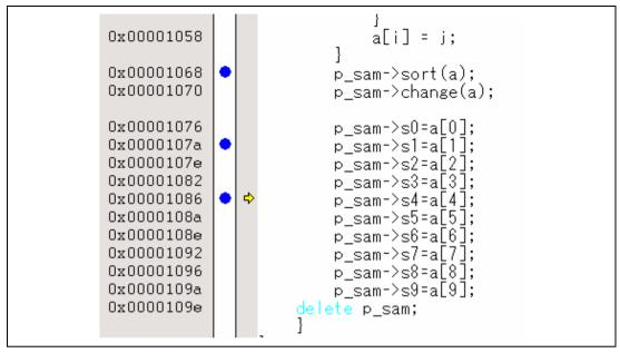
Figure 2.1 [Source] Window at Execution Halted (Sequential Break)
