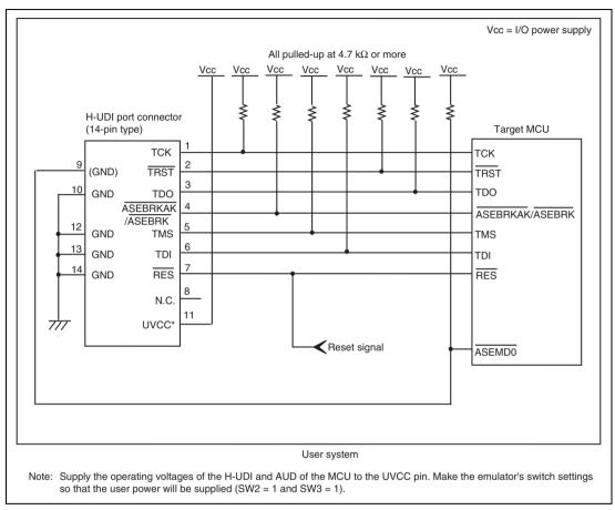
Figure 1.2 Recommended Circuit for Connection between the H-UDI Port Connector and MCU when the Emulator is in Use (14-Pin Type)
