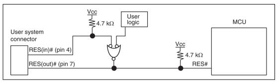
Figure 1.6 Connection of Pin RES#
