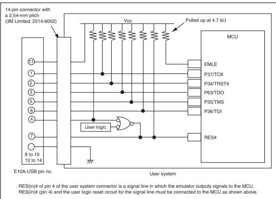
• RES(out)# of pin 7 of the user system connector is a signal line in which the emulator monitors the RES# signal of the MCU. The RES# must be pulled up before it is connected to pin 7 of the user system connector.
