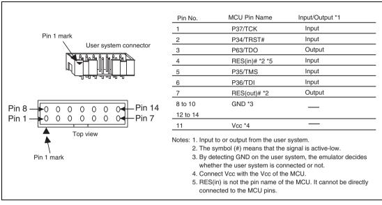
Figure 1.2 Pin Assignments of the User System Connector
