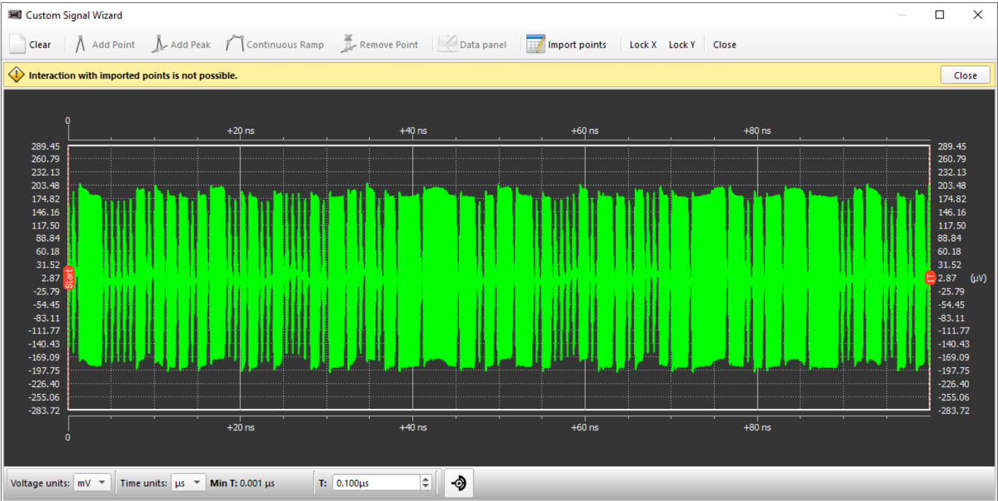
An imported waveform with a large number of points (above 1000)
