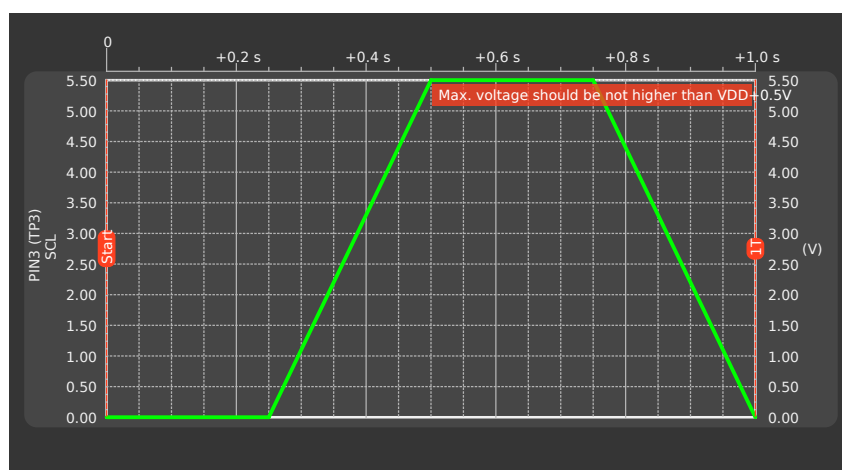
Configuration options of Signal Generator, type Trapezoid (Triangle, Sawtooth)
