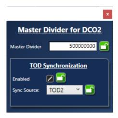
Figure 4. PTP Master Divider Configuration
