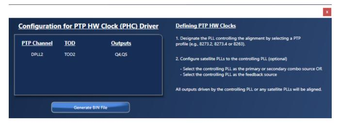
Figure 6. Generate Configuration for PHC Driver (.bin file)
