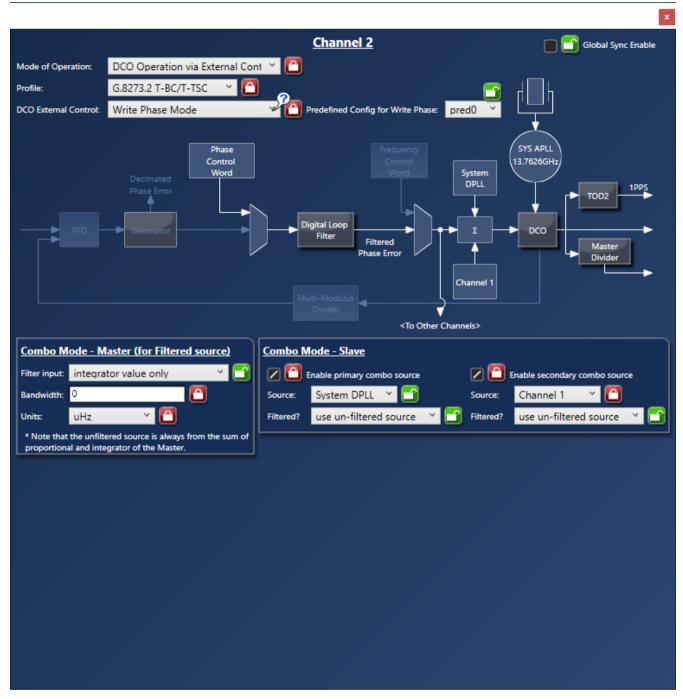
Figure 3. PTP (DCO) Channel Configuration
