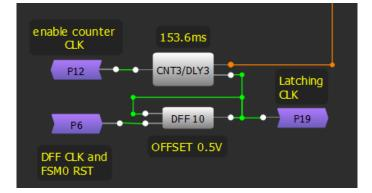
Figure 18. Offset circuit
