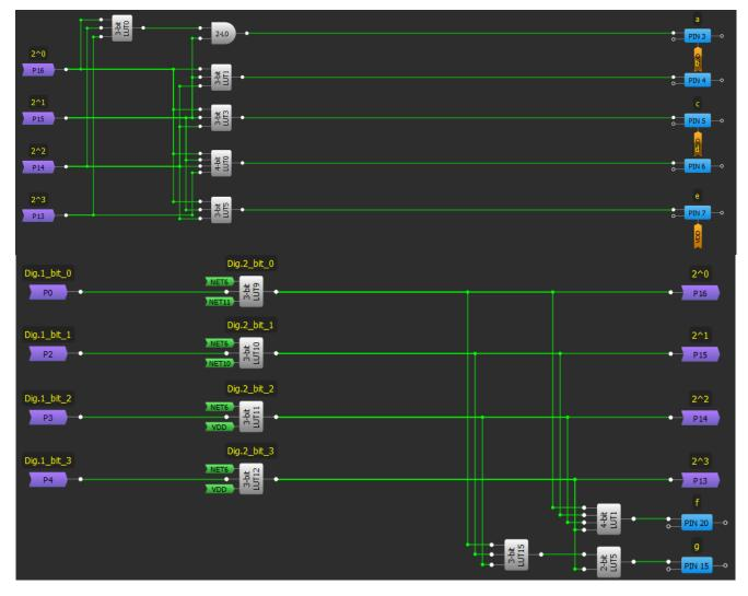
Figure 15. Decoder SLG46620V implementation
