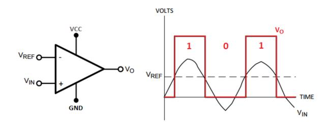
Figure 5. Analog comparator
