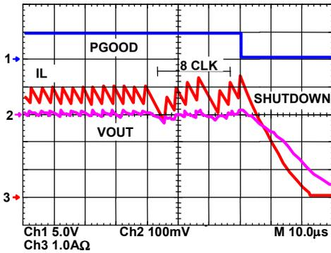
FIGURE 10. OVERCURRENT PROTECTION
