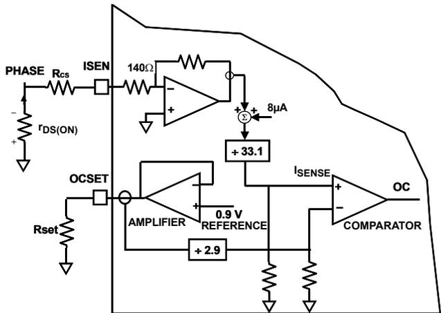
FIGURE 12. EQUIVALENT CIRCUIT FOR OC SIGNAL GENERATOR
