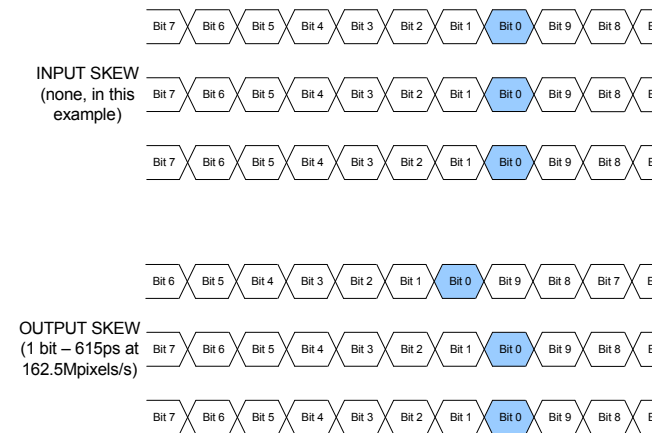
FIGURE 2. MAXIMUM ADDITIONAL INTERCHANNEL SKEW FOR INPUTS WITH NO OR LITTLE SKEW
