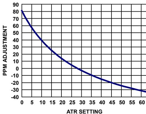
FIGURE 16. ATR SETTING vs OSCILLATOR FREQUENCY ADJUSTMENT
