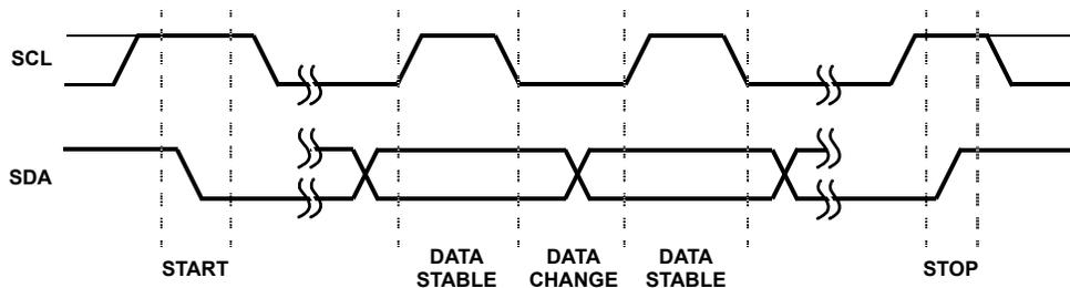
FIGURE 10. VALID DATA CHANGES, START, AND STOP CONDITIONS
