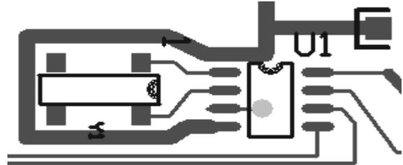
FIGURE 17. SUGGESTED LAYOUT FOR ISL12008 AND CRYSTAL
