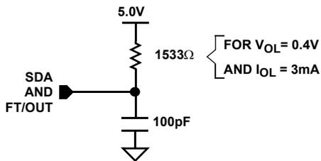
FIGURE 5. STANDARD OUTPUT LOAD FOR TESTING THE DEVICE WITH V<sub>DD</sub> = 5.0V
