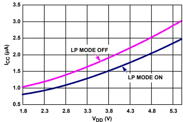
FIGURE 4. I<sub>DD1</sub> vs V<sub>DD</sub> WITH LPMODE ON AND OFF
