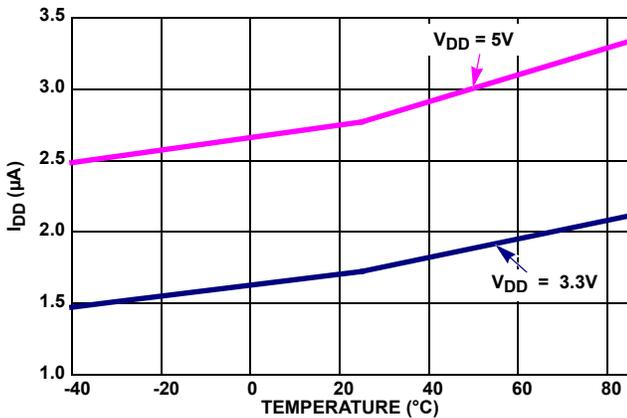
FIGURE 3. I<sub>DD1</sub> vs TEMPERATURE
