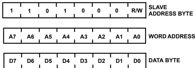
FIGURE 13. SLAVE ADDRESS, WORD ADDRESS, AND DATA BYTES
