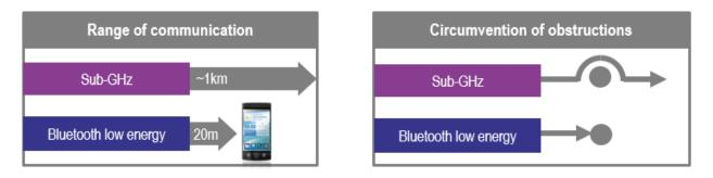
Figure 3. Bluetooth Low Energy and sub-GHz address different wireless connectivity requirements for IoT systems
