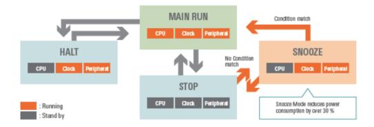
Figure 4. The RL78 has three low-power operating modes to maximize battery life
