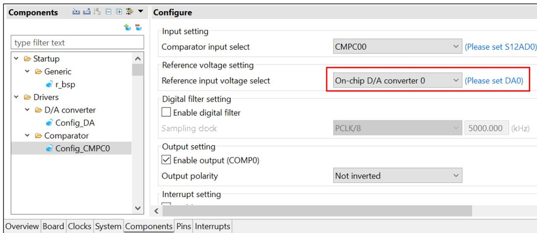
**Figure 1.3: Configuring reference input voltage to “On-chip D/A converter 0” on Comparator GUI**
