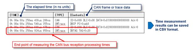
You can quickly locate a problem in the program by finding the measurement end point of the reception processing measurement time from the CAN communication log and checking trace data from the measurement end point.
