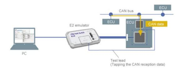
No missing data: The program stops if the reception processing time exceeds a design value.
